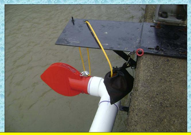
The specially designed cradle bracket holds the strainer end of the articulating arm until needed.
