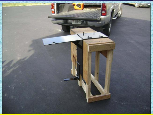
A two-piece mounting bracket was needed – again due to the double-rail guard rail system.
