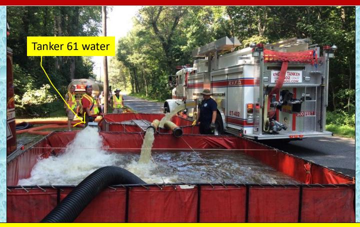
Once the dump site was up and running, tankers that could dump water did so in the dump tanks and tankers that could only pump off did so into Tanker 61. Tanker 61 then supplied water to one of the dump tanks.
