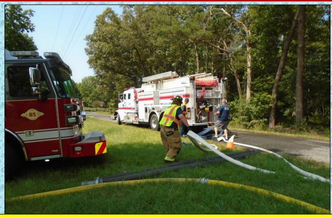
Engine 85 (1500 gpm) drafted from the creek and supplied several lines for loading tankers out on the main road.
