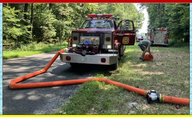
Preston Tanker 202 (2000 gal) was the first unit to arrive on the scene and the driver went right to work supplying a "rural hitch" layout to a simulated attack pumper. Flow was started as 250 gpm around the 2:45-minute mark.
