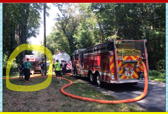
Easton Tanker 61 (6000 gal) arrived around the 20-minute mark and took over supplying the siamese. As additional tankers arrived, they pumped off their water into Tanker 61 using a siamese on Tanker 61.
