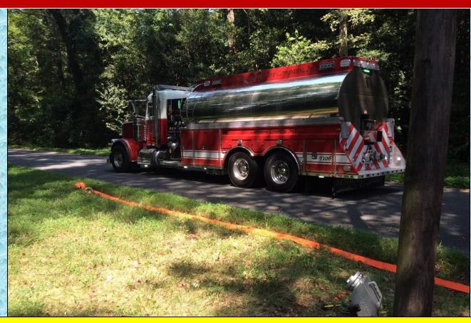
Federalsburg Tanker 106 (4000 gal) was the second arriving tanker and took position to supply the other side of the double-clappered siamese and take over supplying the attack pumper once Tanker 202 was out of water.
