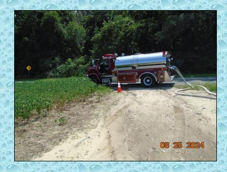
The irrigation system was fed by a stationary fire pump at a nearby creek and water was diverted from the system to the tankers using a valving arrangement on one of the system supply outlets..
