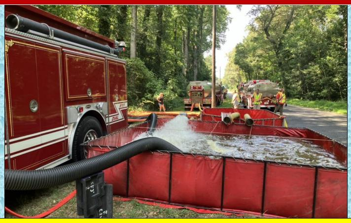
The operation was able to support a 750 gpm sustained flow; a peak flow of 1,067 gpm was achieved for a few minutes.
