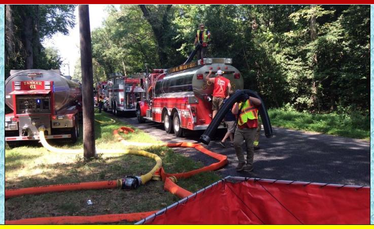
While crews worked on setting up the 2-dump tank operation tankers continued to arrive and pump off their water to Tanker 61 who then supported flow to the attack pumper.
