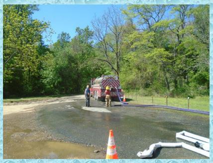
Sudlersville Engine 63 (1500 gpm) drafted from the river at this boat launch and supplied an LDH manifold which in turn supported the loading station.
