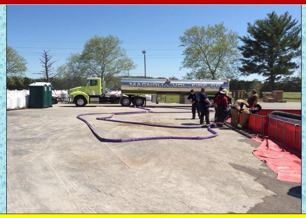
Magnolia Tanker 55 (6000 gal/1000 gpm) arrived at the 72-minute mark and positioned to support dump tank operations.
