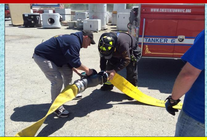
The use of the double-clappered siamese was important to the operation as it allowed for water to be sent to the attack pumper shortly after the arrival of the tanker.
