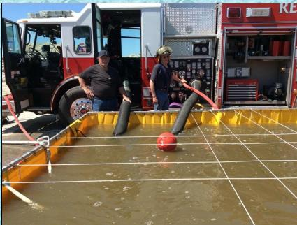
Kennedyville Engine 4 (1500 gpm) was able to deploy twin, 6-inch suctions which allowed the rig to support the fireground flow and the jet siphons.
