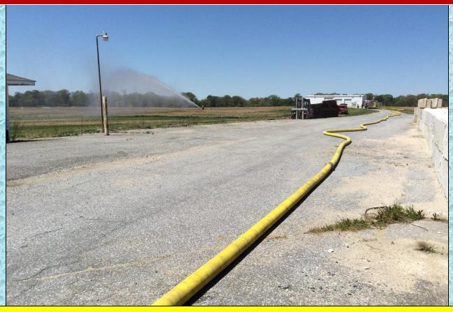
At the 4:30 minute mark water flow was started at 250 gpm at the attack pumper.
