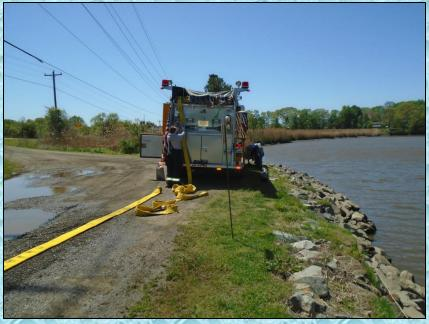
Betterton Engine 5 (2000 gpm) drafted from the river at this recreation area and supplied an LDH manifold which in turn supported a loading station.
