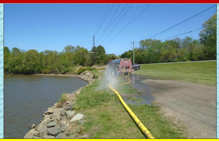
The crews worked hard to load the tankers at the 1000 gpm fill rate goal and get them back on the road to the dump site. Most every rig loaded using twin, 3-inch fill lines.
