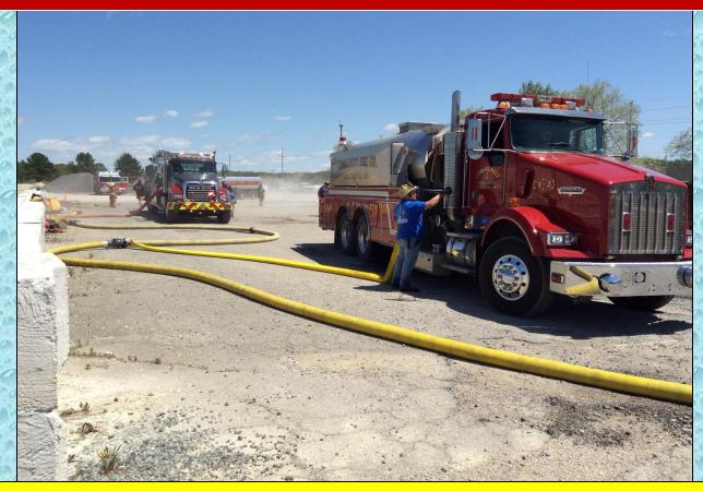
The second-arriving tanker positioned to support the rural hitch and plans were underway to locate a dump site for transition to dump tank operations.
