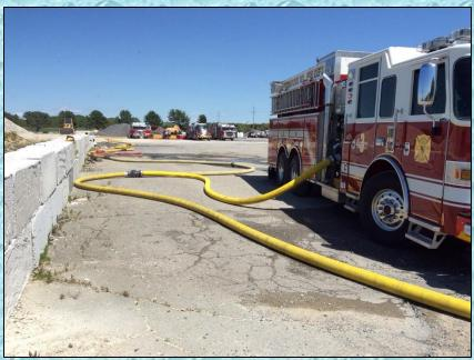
The first load of water is dumped into the dump tanks around the 24-minute mark and about one minute later the water supply transitions to a dump tank operation.
