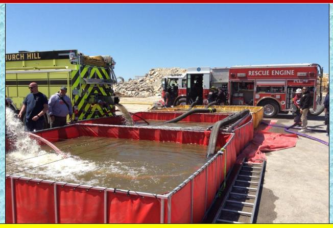
Flow was moved to 750 gpm around the 25-minute mark and 3 dump tanks were operational.
