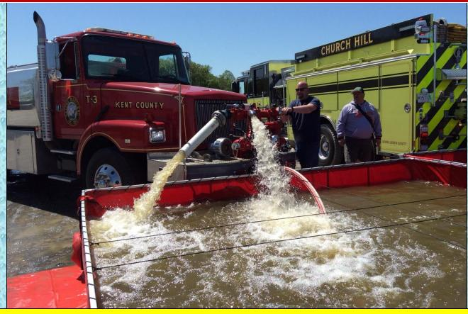
Additional tankers arrived and flow was moved to 1000 gpm around the 30-minute mark.
