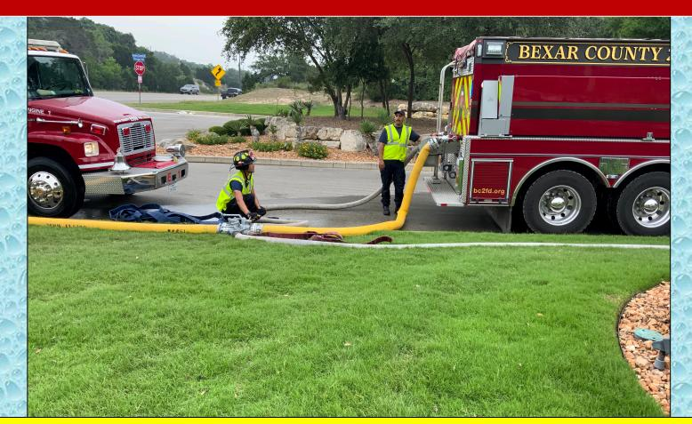
When possible, the crews tried to use LDH to load the tenders at the 1000 gpm target fill rate.
