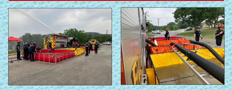
At the 45-minute mark flow was moved to 800 gpm using Engine 116's prepiped deck gun.
