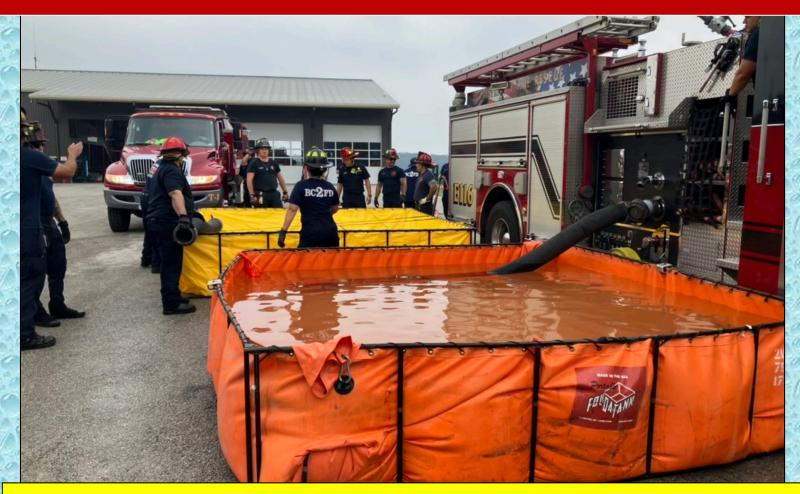
By the 8-minute mark, the first dump tank is in operation and water flow is restored to 300 gpm at a Mercury nozzle. A second dump tank is also deployed.
