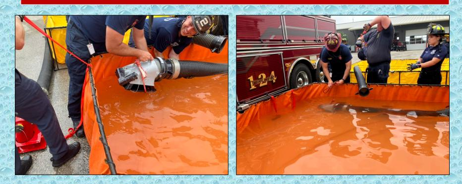
Around the 13.5-minute mark a TFT low level strainer replaced the initial strainer to improve the intake into the pumper. This made a big difference later on when the pump had to pump 800 gpm plus supply three jet siphons.
