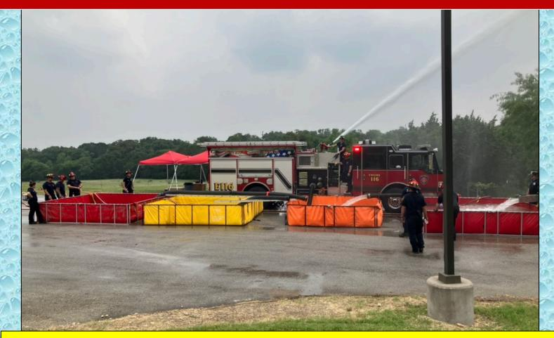
The final layout. Four dump tanks, two fill sites, and eight tenders were used to support the 800 gpm flow at this drill.
