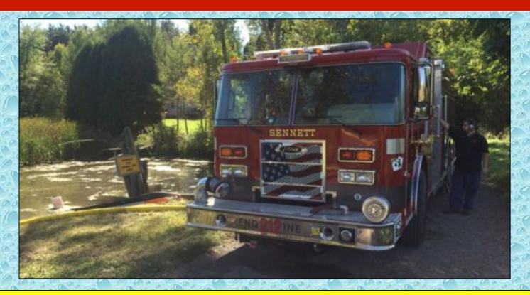
The crew from Sennett E2 struggled due to constant strainer clogging issues. This could have been remedied by a circulating line that was pointed at the strainer to keep the "gack" away. This engine fed an LDH line that terminated in a manifold with several fill lines at the end of the driveway.
