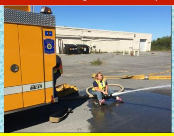
The crew stretched 25-feet of 4-inch hose to a Hose Monster flow diffuser that served as the means by which all water flow would be measured. The diffuser simulated the use of a portable master stream device. However, the first 10 minutes of water flow was done by handline at 250 gpm.
