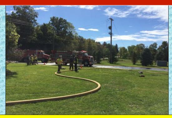
The crew stretched LDH to a gated wye and established two fill lines. They filled one tanker at a time but were able to hook up to the next one so no time was wasted between fills. A second manifold was used to help drain the LDH between tanker fills but this device was leaking and taken out of service due to safety concerns. However, the stretch did prove useful to get the tankers off the main road but allowed them to make a nice traffic flow and not have to turn around.
