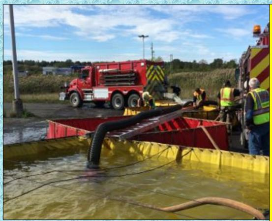
With the addition of a fourth dump tank and a third siphon water transfer operations became an issue due to the fire flow demands of the attack pumper combined with the required flows of the jet siphons.
