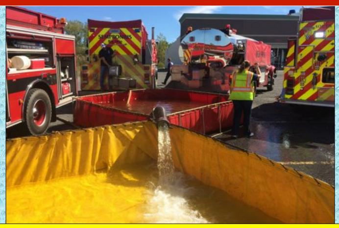
The dump site crew decided to set up the tanks in a diamond fashion so as to allow for rear dumping as well as side dumping.
