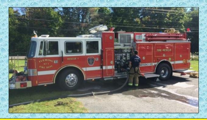
The crew from Fleming worked very quickly and had this fill site operational in about 10-minutes. This engine has a 1750 gpm pump but the crew realized a much lower flow due to the use of the front intake. With the use of the second "pony" suction this engine was able to fill at close to 1000 gpm.
