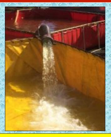
The flow from this jet siphon is a good, solid stream of water – which is exactly what is needed. Note the ladder spanning the tanks in the last slide - moving the water once is the most efficient way to manage multiple tanks.
