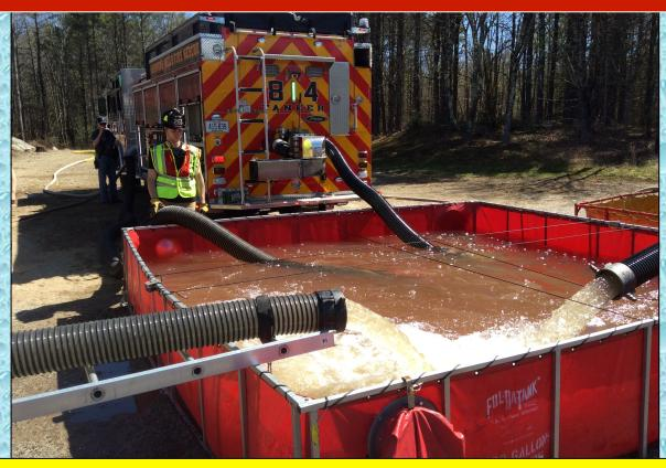
At the 37-minute mark Tanker 84 had twin suction lines in operation. No interruption in flow occurred because the suction intake had a control valve and the pump had an automatic air primer.
