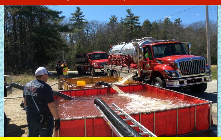
Kennebunkport Tank 1 (3500 gal) was the only vacuum tanker hauling water in the drill and did a good job of self-loading at the fill site. The tanker was also the largest tanker hauling water.
