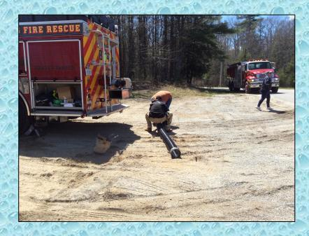
Goodwin Mills Tanker 84 arrives on scene and goes to work setting up as the dump site pumper. They are simulating supplying water to a first-arriving pumper – there just was not one available at drill time. The rig is equipped with a rear intake, so it was the first suction connection made.
