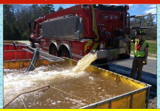
At the 45-minute mark, flow was moved to 800 gpm. The tanker approach route was changed so that the rigs could dump on their driver's side...which made it easier and faster for the drivers.
