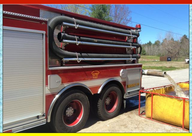
Alfred Tank 95 (2500 gal) carried plenty of 6-inch suction hose which was eventually used to get a second intake line up and running on Tanker 84, the dump site pumper.
