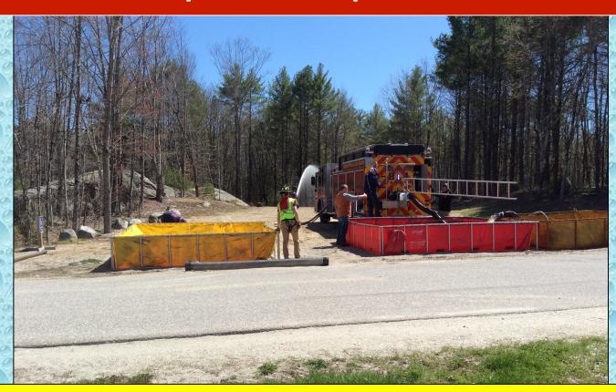
The plan to expand operations included the addition of a third dump tank (2500 gal). Folks took time to add some "space" when deploying the third tank so that two tankers could dump water at the same time. This was important since four of the five tankers hauling water were tandem-axle large capacity tankers.
