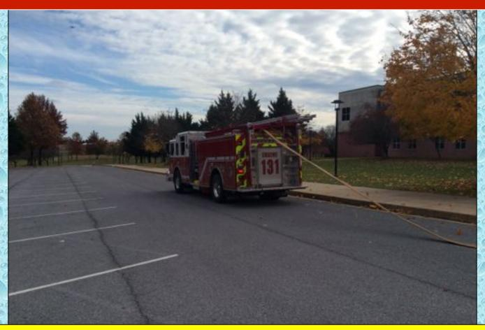
Gamber Engine 131 arrives on the scene and lays out several hundred feet of 4-inch LDH supply line. The unit will serve as the attack pumper at this drill.
