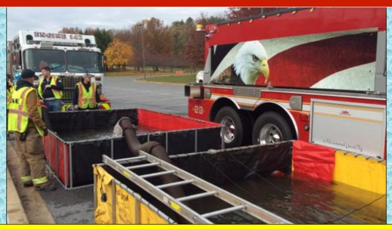
At the 15-minute mark flow was moved to 500 gpm and a two-dump tank operation was under way. Urbana Tanker 23 from the 1<sup>st</sup> Tanker Task Force is shown here arriving at the dump site and preparing to dump its water.
