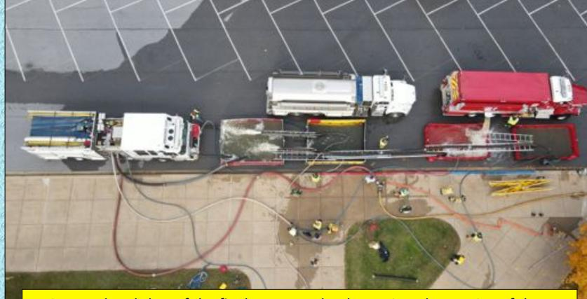
A nice overhead shot of the final set-up at the dump site. The spacing of the dump tanks in the single-lane arrangement was critical to allowing two tankers to dump simultaneously.
