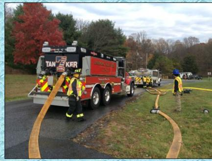
Special Unit 6 was able to load tankers at rates in excess of 1000 gpm using 5-inch LDH and.
