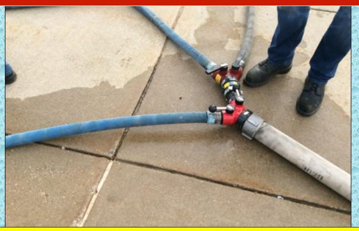
A little bit of creativity allowed one 3-inch line to supply and support the operation of three jet siphon water transfer devices.
