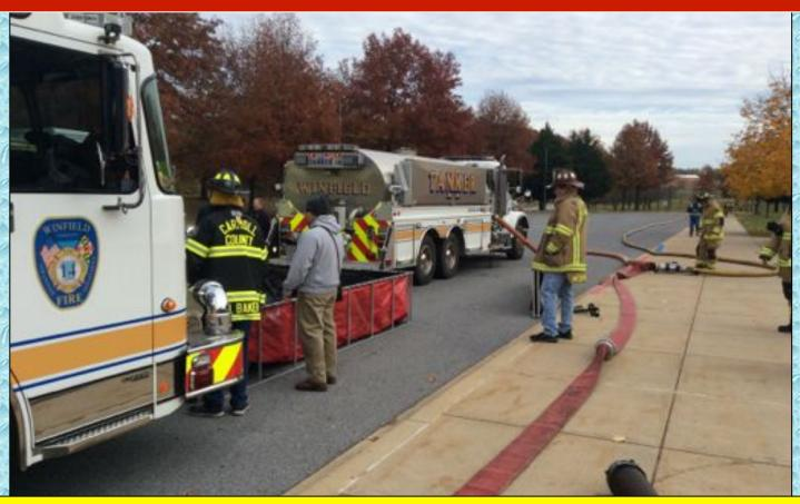
One goal of the drill was to use a "single-lane" dump tank arrangement in front of the dump site pumper.
