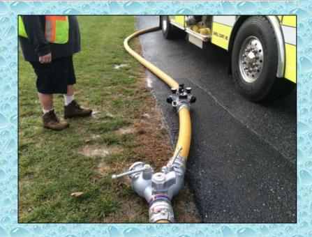
Brush 105 was able to load tankers at rates just under 1000 gpm using 4-inch LDH.
