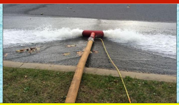
At the 75-minute mark, flow was moved to 1200 gpm where it was sustained for the remainder of the drill. A HoseMonster flow diffuser was used to measure the flow.
