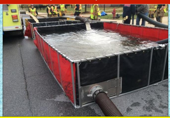
Two dump tanks in operation with flow just above 500 gpm and about 34-minutes into the drill.
