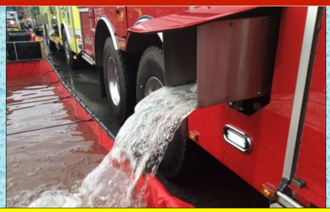
This tanker really needs to "cut and run" for a another load of water. There is no need to wait for all of the water to leave this tanker.....get on the road for another load....especially since there are tankers waiting behind this one to dump their water.
