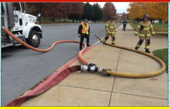
The rural hitch provided sufficient water supply to the attack pumper and allowed time to get the dump site set up.
