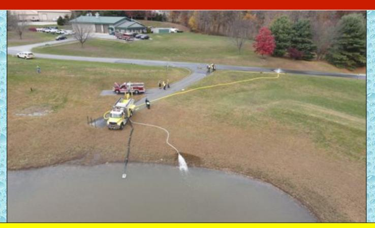
Pleasant Valley Special Unit 6 (1500 gpm) drafted directly out of the pond. New Windsor Brush 105 (1000 gpm) drafted from the dry fire hydrant. Both used LDH to load the tankers.
