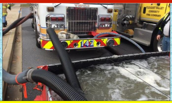
Engine 142 ended up drafting through three, 6-inch suction inlets which allowed the pumper to easily support the 1200 gpm flow to the attack pumper and supply all of the jet siphon devices. The Hale Qmax 1500 gpm powered by a 500 hp motor provided plenty of "pump" for this operation.
