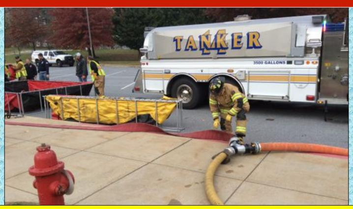
Tanker 14 (1500 gpm/3500 gal) supplied Engine 131's double-clapper siamese... aka "a rural hitch" operation. Meanwhile, Engine 142's crew grabbed the two dump tanks off of Tanker 14 and went to work building out a dump site in anticipation of a much larger fire flow.
