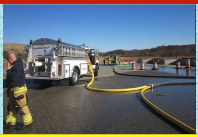
The next time Tanker 4-1 arrived at the dump site, they pumped off their water using the clappered siamese because another rear dumping tanker was using the offloading spot.
