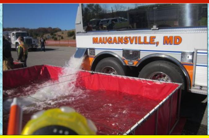
Maugansville Tanker 13 (3,000 gal) was the first tanker to dump a load of water. Clearspring Tanker 4 (3,000 gal) pumped off its first load of water using the "rural hitch" set up.
