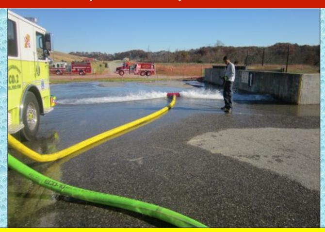
Units on the second tanker task force are seen staged in the background as flow continues at 500 gpm through the flow diffuser.
