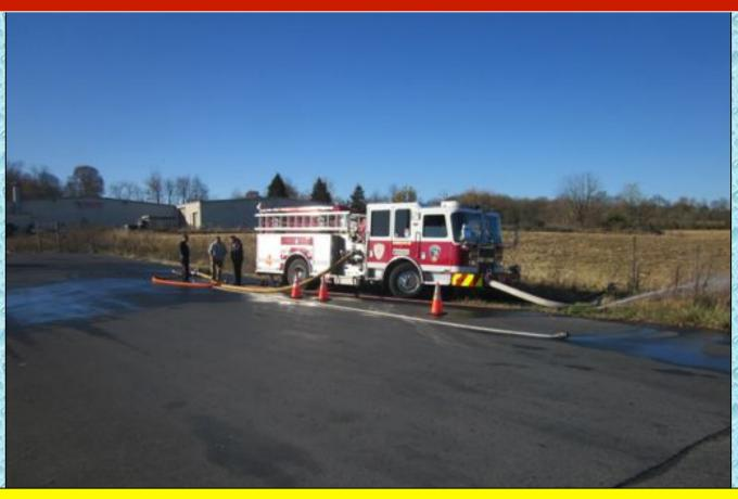
The hydrant fill site worked just fine and was able to load tankers and easily meet the 1,000 gpm loading rate.
