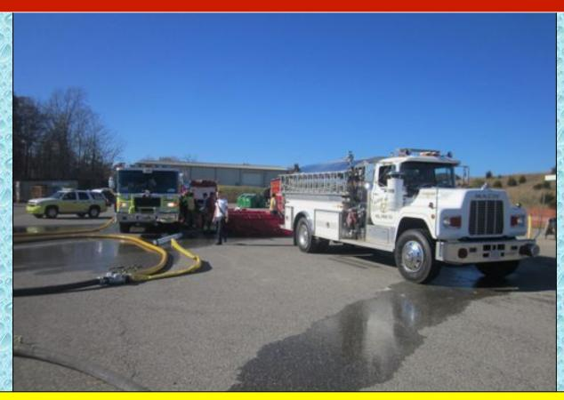
At the 16-minute mark, the flow was moved to 500 gpm and a dump site operation was completely underway. The nurse tanker line was left in place in case it might be needed later.
