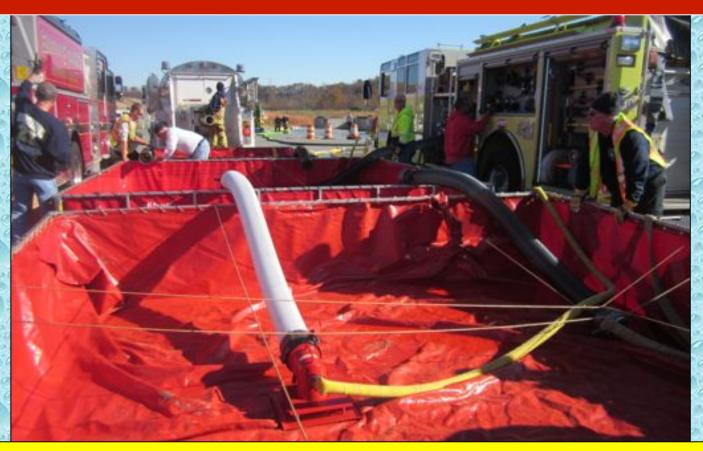
Crews set up a three-dump tank operation with multiple jet siphon transfer devices.
