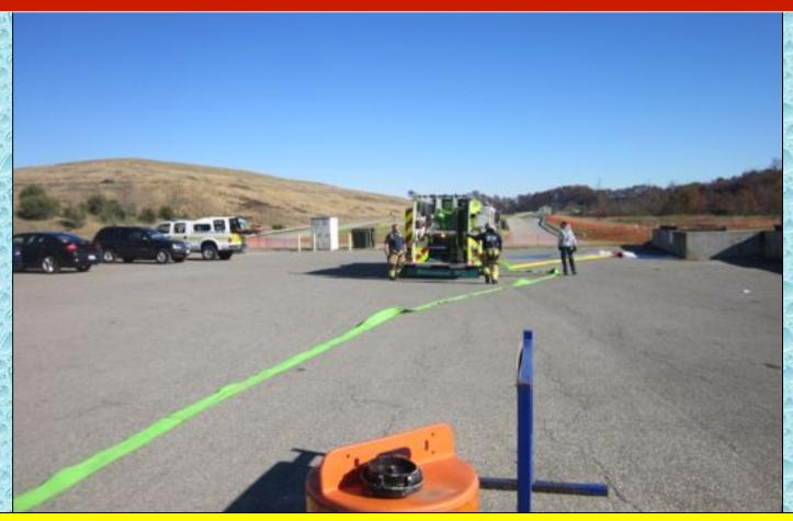
At the 5:00 minute mark, water flow was started at 250 gpm using a HoseMonster flow diffuser device supplied by Engine 21.
