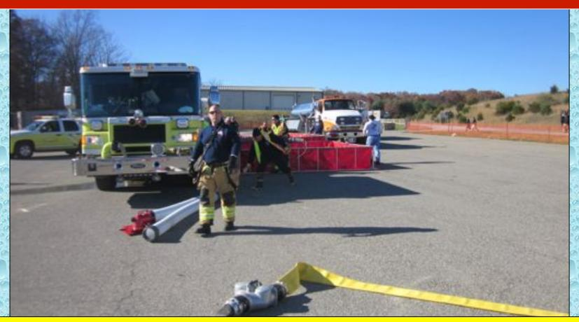
Engine 602 begins setting up the dump site. A 4-inch double-clappered siamese was used on the end of Engine 21's supply line in order to support a nurse tanker operation that could eventually transition to a dump site operation without interruption of water flow.
