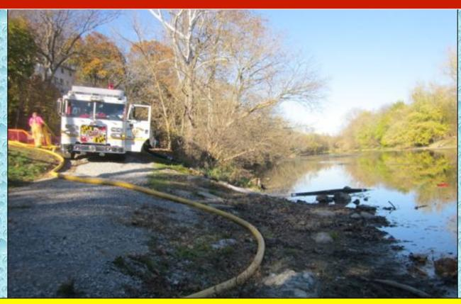
While water quantity was ample, quality was poor due to depth and debris. The crews at this site struggled to keep suction strainers clear of debris. They still were able to load tankers throughout the 2-hr drill – just well below the 1,000 gpm loading goal.
