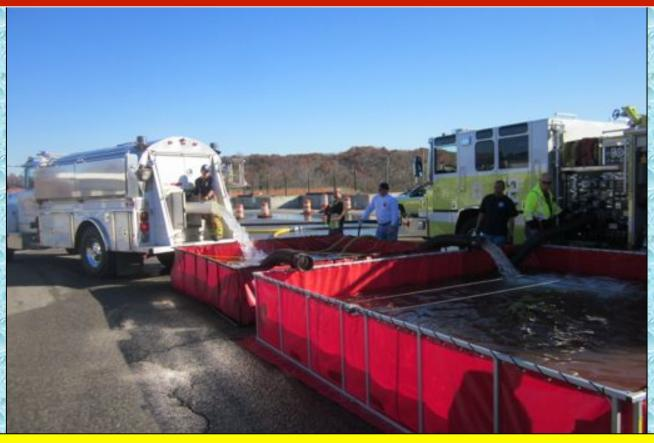
Clearspring Tanker 4-1 (2,000 gal) could only dump from the rear, thus it positioned past the last dump tank and backed up to the tank so that the side dumping tankers would not be blocked out.
