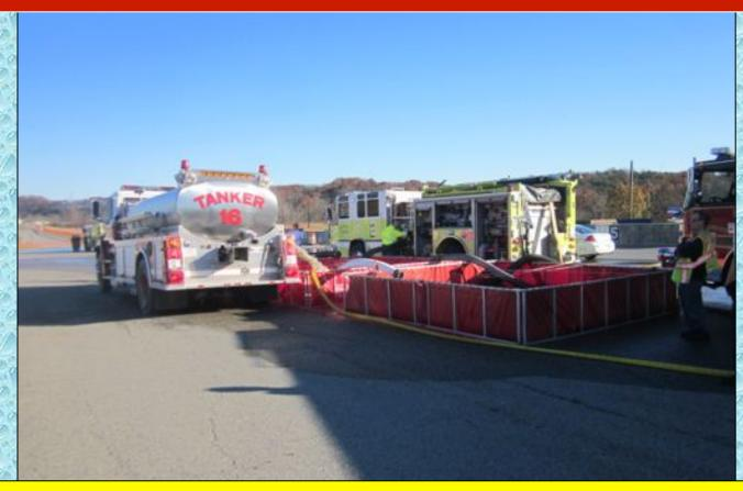
In the end, the dump site operation was able to reach a peak flow of 750 gpm at times. However, struggles at one of the fill sites limited the dump site ability to support the peak flow with any regularity.
