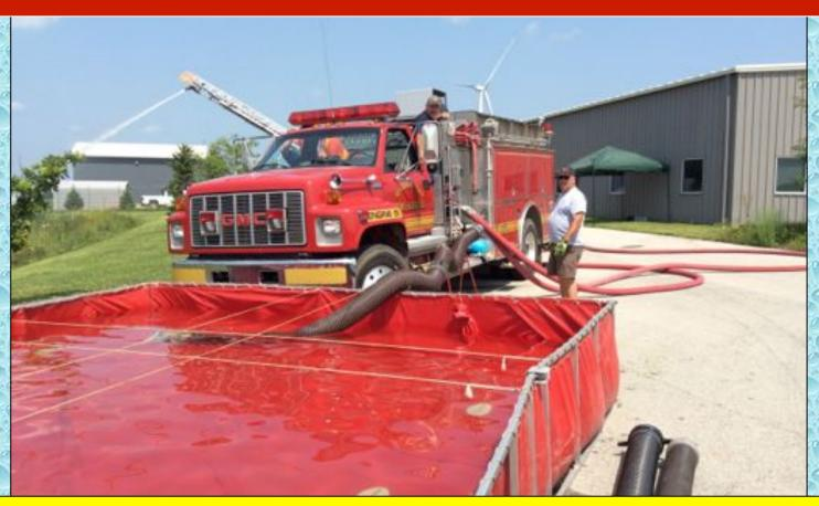
At the 5-minute mark, water flow was started to the ladder truck at 500 gpm using a single, 3000-gal dump tank as supply.
