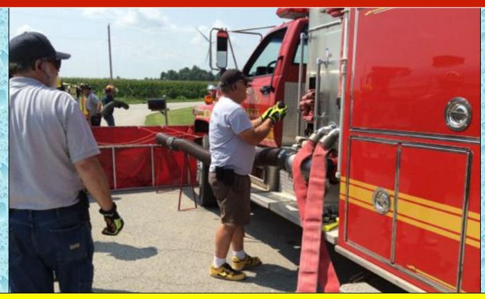
Crews worked very hard to get the first dump tank up and running by the 5-minute mark. They chose to place the first dump tank (3000 gal) in front of Engine 51 and used a suction elbow to assist in that process.
