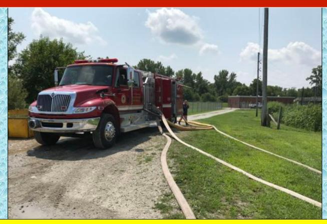
Incoming tankers were loaded using either dual, 2-1/2-inch lines or a single, 5-inch line.
