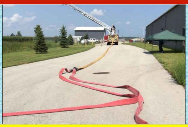
Wildcat Ladder 62 was pre-positioned for elevated master stream operations. A length of 5-inch LDH equipped with a clappered siamese was laid out by the ladder crew in preparation for the arrival of the engines and tankers. Engine 51 set up to supply the siamese using dual, 3-inch lines.
