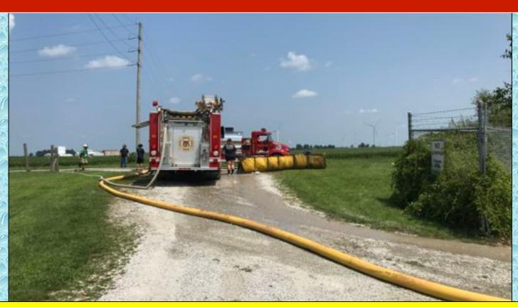
Wildcat Engine 61 was set up near the road and was supplied by Duck Creek Engine 881 through 500-ft of 5-inch LDH. Because flow was reduced by the front suction inlet on the Duck Creek engine, the Wildcat engine set up a dump tank and used a modified open relay to supply water for loading tankers at the 1000 gpm rate.
