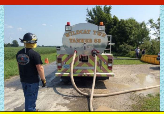
Most of the tankers hauling water were loaded using dual, 2-1/2-inch lines controlled at Engine 61's pump panel.
