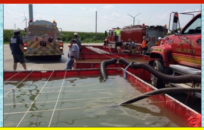
Crews deployed a fourth dump tank around the 45-minute mark and worked to get sufficient water transfer devices in operation. Sharpsville Engine 41 was brought in to support the jet siphon use by taking over pumping some of the jet siphons so that the dump site pumper could free up pump capacity to better support the ladder truck.
