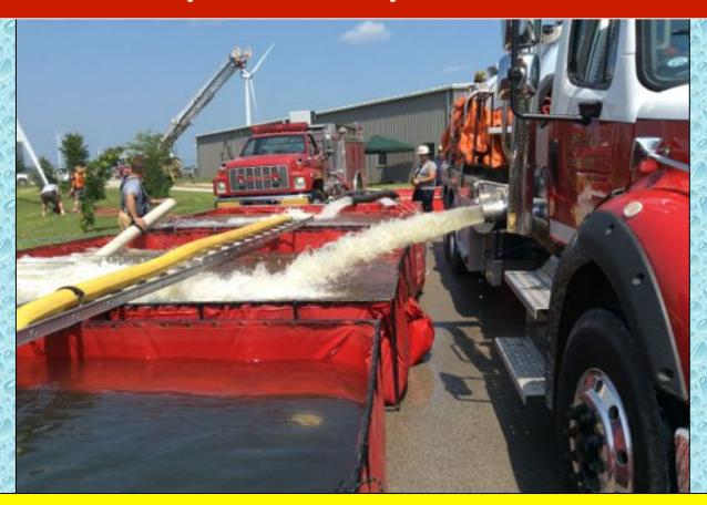
At the 59-minute mark, flow was moved to 1,000 gpm. Bass Lake's vacuum tanker is shown in this photo off-loading its water. A short length of 5-inch LDH was used in lieu of suction hose on one of the jet siphons.
