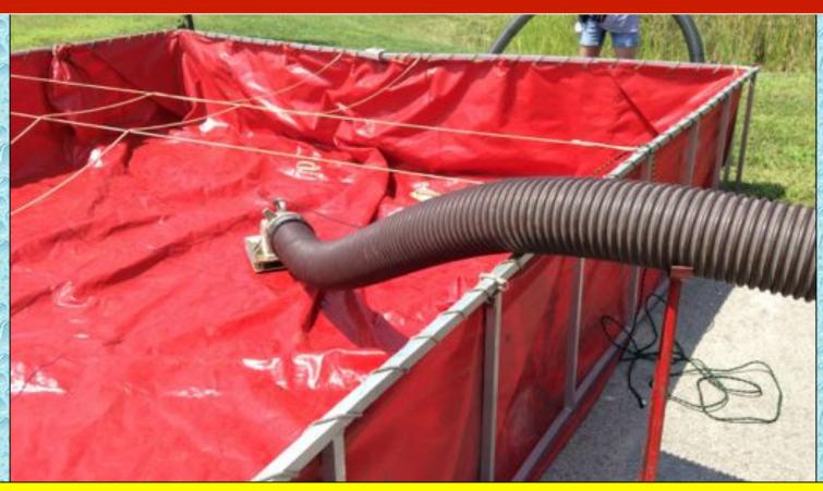
A Fol-Da-Tank low-level strainer was used as the suction strainer. The plan was to support the ladder truck with a 1,000 gpm flow so the dump site crew knew that they had to plan for the expansion of the system.
