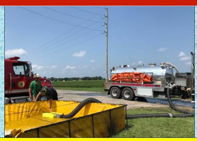
The Bass Lake vacuum tanker self-loaded each time simply by accessing the water in the 3,000 gallon dump tank.
