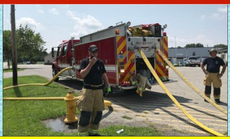
Atlanta Engine 351 used a Windfall fire hydrant as the water supply and loaded tankers using dual, 3-inch lines. They were able to load tankers at over 1,000 gpm.
