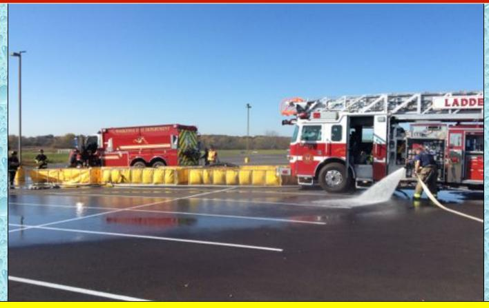
At the 5:00-minute mark water flow was started at 250 gpm using Ladder 1671's tank water (475 gal). By the 7-minute mark the first dump tank was in operation.
