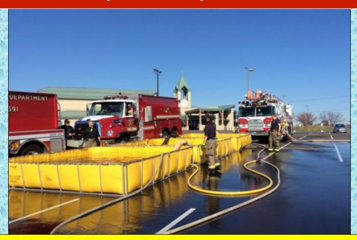
Around the 17-minute mark water flow was moved to 500 gpm and a three-dump tank operation was underway. All three dump tanks were 3500-gal in capacity.
