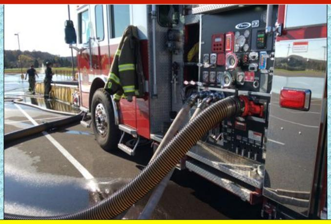
With the second suction line now in operation the crew was able to flow 1,000 gpm and operate three jet siphons.
