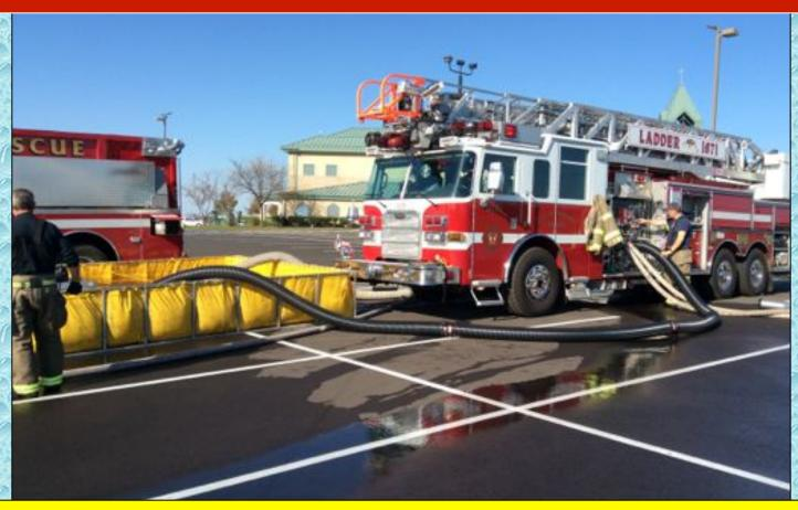
Eventually, enough suction hose was located to build out a second suction line using the driver side suction inlet.
