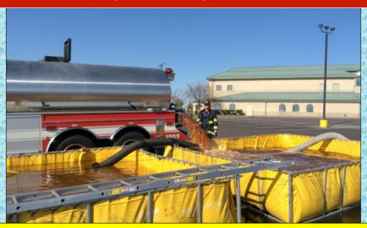
With two fill sites in use (a stream and a hydrant), tenders were directed to a specific site by the Water Supply Officer. Vernon Tender 1292 dumps a load of hydrant water here in this photo!
