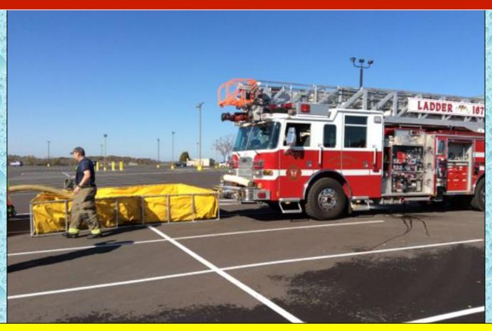
The dump site crew decided to arrange dump tanks in front of the 1500 gpm quint simulating a "Single-Lane Tank" layout. The first dump tank used was one of two, 3500-gal dump tanks carried on the first-arriving tender.
