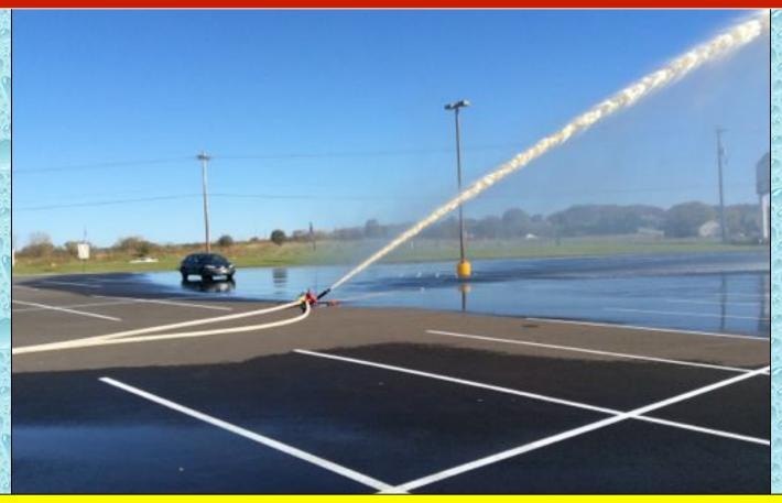
At the 102-minute mark flow was moved to 800 gpm and then to 1000 gpm at the 106-minute mark.
