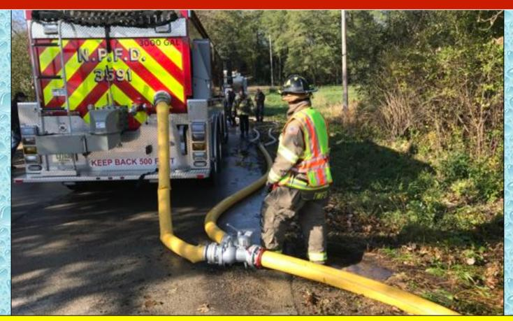
5-inch LDH was used at the stream fill site to load tenders. Loading operations were very efficient and tenders were quickly placed back on the road to the dump site.
