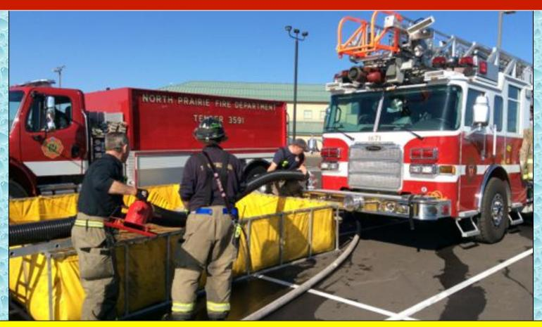
Because the suction strainer on the initial suction hose line was flow-limiting, the crews worked to build a second suction line using the quint's front intake.
