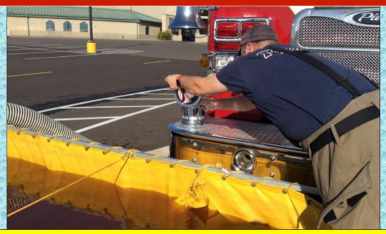
However, a mechanical issue arose with the front intake making it nonoperational and thus it had to be capped in order to eliminate a large air leak.
