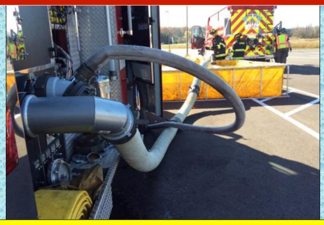
To facilitate full-flow drafting with the dump tanks located in front of the quint, a Kochek suction elbow was used on the officer side suction inlet.
