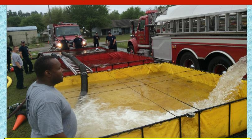
Three dump tanks and two jet siphons were eventually used to support the 1250 gpm operation.
