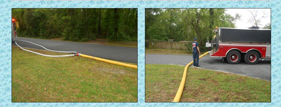
The fill site pumper did not have an LDH discharge so two smaller lines were siamesed into a 5-inch LDH fill line so that tankers could be loaded at a 1000 gpm rate.
