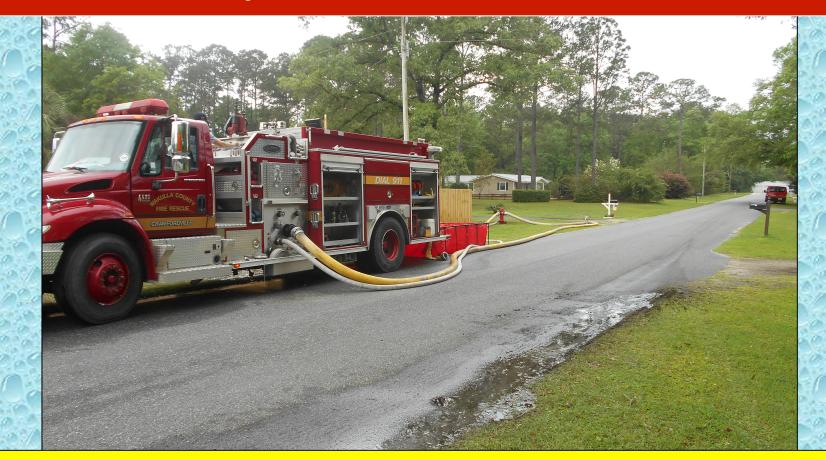
The second fill site used a similar set up arrangement to load tankers at the target 1000 gpm fill rate.
