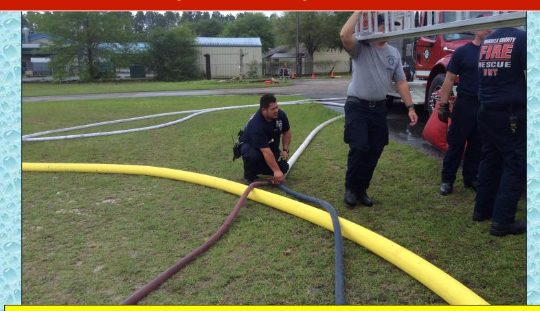
Jet siphon control was moved to a gated wye thus relieving the pump operator of having to manipulate water transfer devices.
