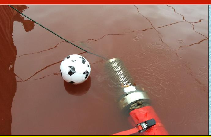
With no top-performing suction strainer available, Engine 11 chose a barrel strainer so that maximum capacity could be achieved using a single-suction inlet.
