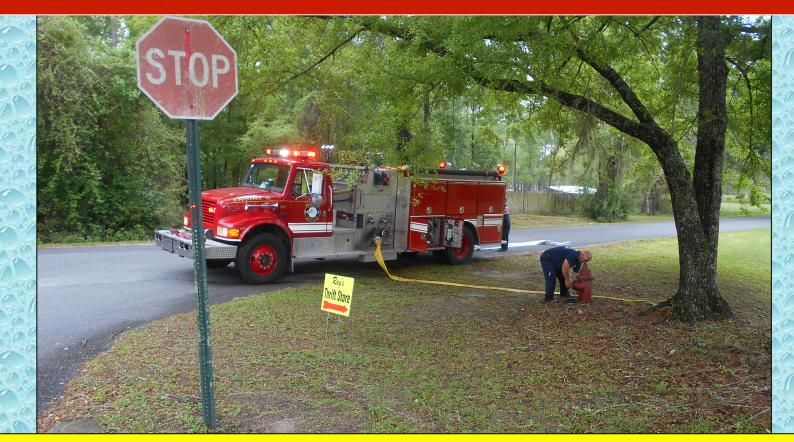
Water was taken directly from the fire hydrant into the fill site pumper (1250 gpm) and from there a tanker fill station was built out by the time the first empty tanker arrived on location.
