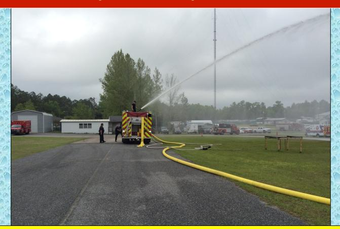
At the 105-minute mark flow was moved to 1250 gpm using Engine 3's prepiped deck gun.
