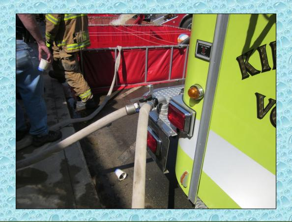
Two additional jet siphons were supplied by this pre-piped wye on the front of the Killingworth pumper.
