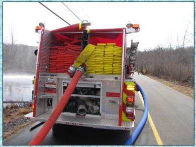
Durham Engine 1 (2,250 gpm) also used dual suctions and 5-inch LDH to support their 1,500 gpm tanker fill station.
