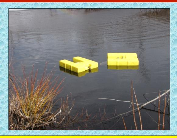
Floating strainers were used because of the silted bottom of the pond and the aquatic vegetation.
