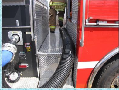
Durham's top mounted pump panel made it easy to run the additional suction hose.
