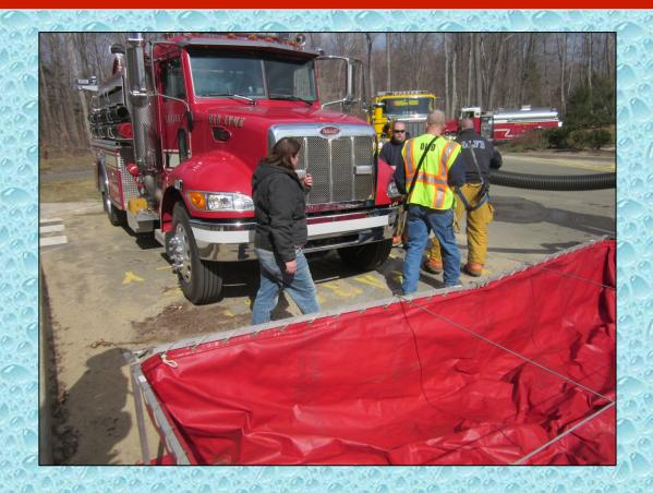
As soon as the pumper crew got the rig into position, the first tanker arrived and a dump tank was set-up in front of the Old Lyme pumper.
