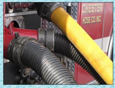
Chester Engine 3 (2,000 gpm) used dual suctions and 5-inch LDH to fill tankers at a rate of around 1,500 gpm. Very Impressive!
