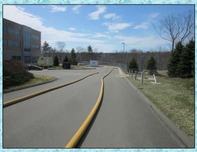
With the flow maximized at 1,300 gpm, action was taken to expand the operation to use all of the available resources. A second, 5-inch LDH supply line was laid (using another pumper) to the rear of the school in order to supply a second, aerial tower.
