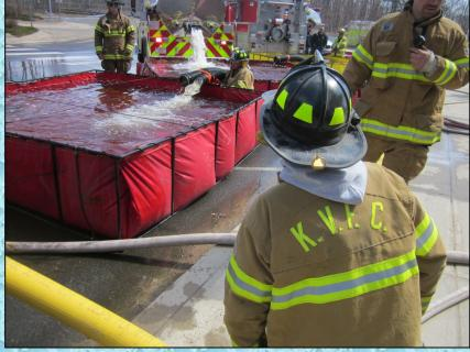
Two additional jet siphons were supplied using the gated wye arrangement shown above. The advantage of using the gated wye set-up is that it takes the jet siphon operation away from the pump operator – making one less concern for the operator. The disadvantage is that the wye requires another person to operate it.
