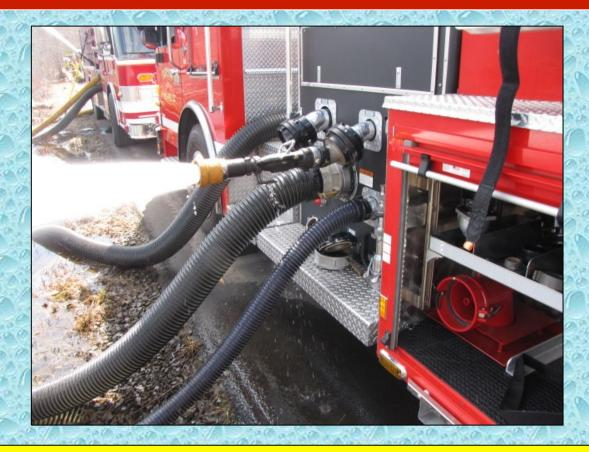
To enhance operations, the Durham crew added a third suction using the pump's 2-1/2-inch auxiliary intake.
