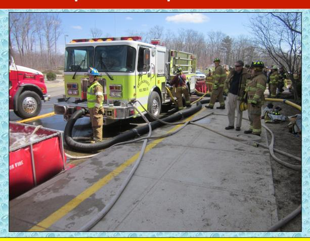
The Killingworth pumper used three suction lines in order to maximize its flow potential – this is another reason to carry additional lengths of hard suction hose.
