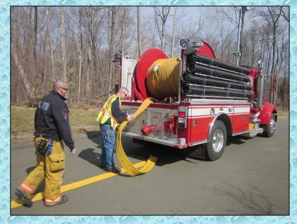
The drill began with Old Lyme's hose reel pumper (1,500 gpm) laying a 900-ft supply line of 5-inch LDH from an aerial tower in the rear of the school.
