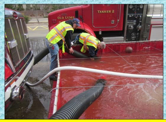
The low level strainer on the first suction line created a few issues throughout the drill – it kept trying to flip over and was also susceptible to taking in air when tankers dumped their water in that area of the dump tank.
