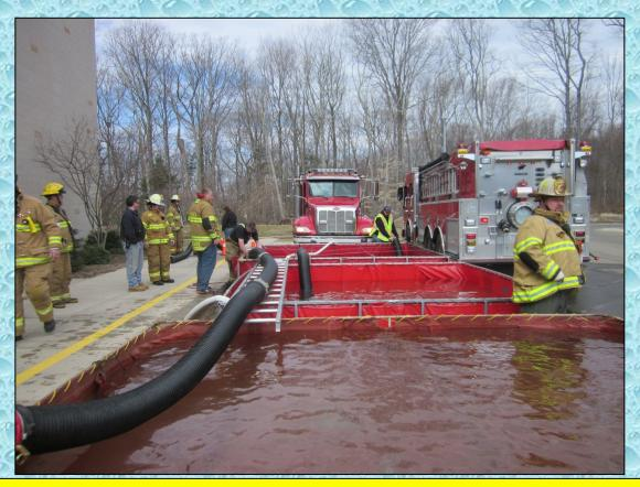
All of the tankers were very well equipped with suction hose and appliances – this made it easy to build out the water transfer devices for a multiple tank operation.
