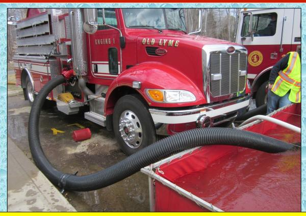
In order to increase flow, the dump site pumper crew connected a second, 6-inch suction line using the officer's side inlet. The pumper is outfitted with an MIV on all inlets – this drill is a good example of why suction inlet control valves are so useful on pumpers.
