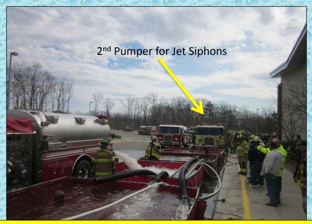
At around the 48:00-minute mark, a second pumper (Killingworth Engine 1) was placed into operation at the dump site to run jet siphons. The flow was then moved to 1,300 gpm.
