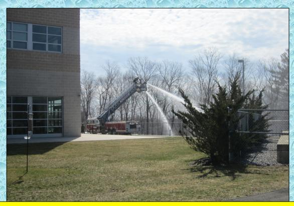
Flow to the first aerial tower could not be increased above 1,300 gpm - most likely because of a flow limitation at the rear discharge on the Old Lyme pumper and because of the 900-ft of 5-inch hose — the hose had reached its test pressure limitation.
