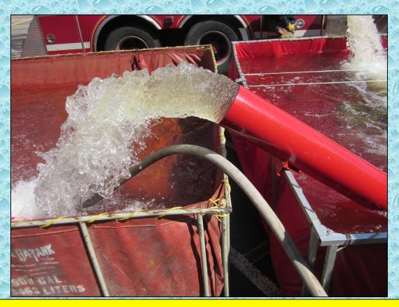
Of course, water transfer operations were critical to the success of this "big water" drill. An 8-inch Holley Tube (Kochek) is shown here being used as one of transfer mechanisms.
