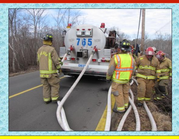
Crews used short lengths of 3-inch hose outfitted with Storz fittings to load the tankers.
