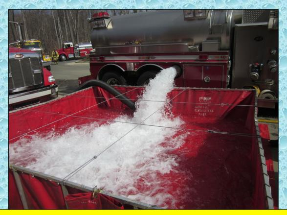
With everything set up, water is dumped into the first tank and water flow is started. One issue that arose was the position of the low level strainer in the dump tank in relation to where the tankers were to dump their water.
