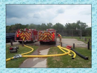
The use of the jumbo-wye made it much easier to load the tankers without having to have the pump operator open and close valves.
