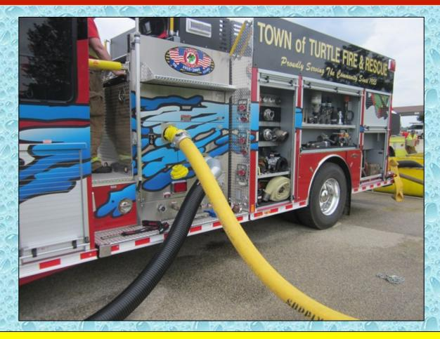
Engine 51's high-flow discharge was used to supply the portable monitor via 5-inch LDH.
