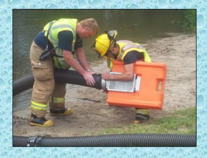
Several lengths of suction hose were needed to reach the creek. A floating strainer was the strainer of choice for the crew.
