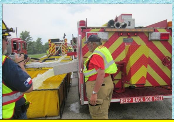
With the flow now at 1,000 gpm and tankers waiting to offload water, a fifth dump tank (3,000 gallons) was placed in service to the rear of Engine 51. This additional dump tank allowed tankers to offload their water and head for another load.
