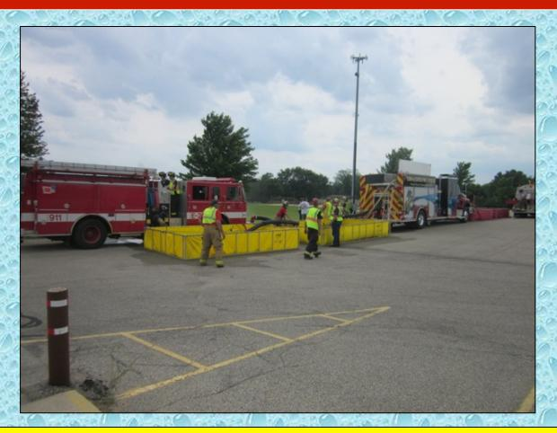
Water supplies were stretched thin at this point in the drill. There are no tankers waiting to dump and the rear dump tanks are almost empty.
