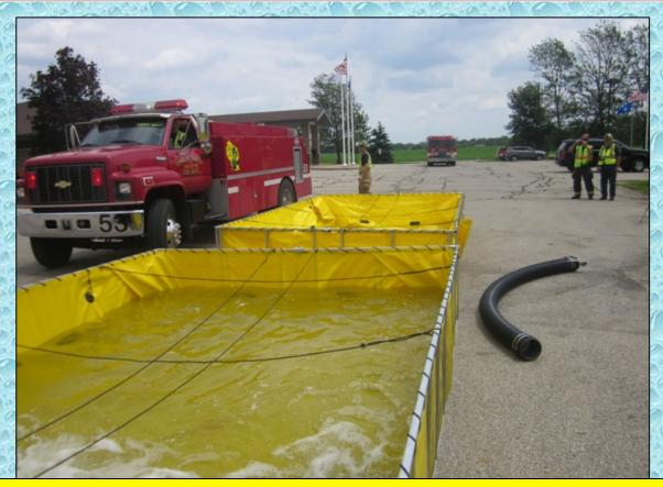
Turtle Tender 53 was the next unit to arrive and its crew went to work setting up a second dump tank. Notice that both of the dump tanks are rectangular in shape. They hold 3,000 gallons each.
