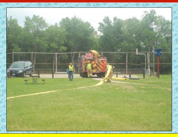
The crew was ready just in time and is shown here stretching a 5-inch supply line up to the tanker loading area.
