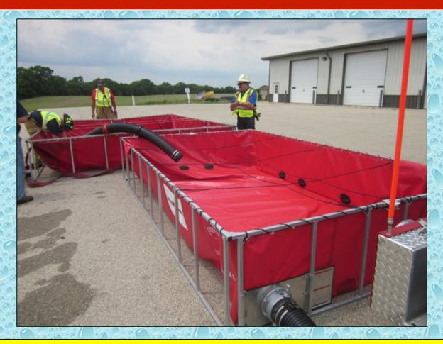
A fourth dump tank (3,000 gallons) was set-up in front of Engine 51 in preparation for moving to a higher flow.
