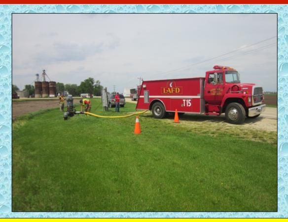
Perhaps the most impressive fill site was the one that used the 1,200 gpm irrigation well as the supply source.
