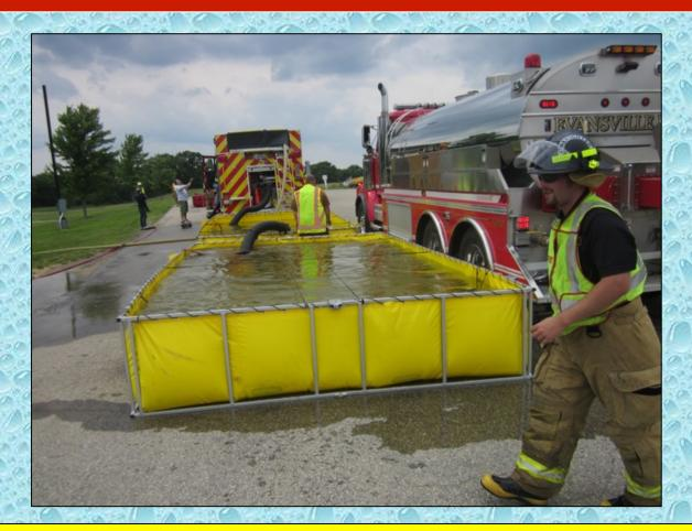
The units from the Water Supply Task Force provided plenty of water and at the 15-minute mark, the flow was moved to 500 gpm.
