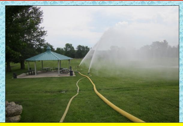
At the 70-minute mark the flow was moved to 1,500 gpm and then again to 1,750 gpm at the 80-minute mark. Unfortunately, one of the fill site pumpers had to respond to a "real" incident at the 85-minute mark and the flow at the dump site had to be reduced to 550 gpm for awhile.
