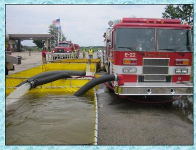
The five-tank arrangement proved to be a bit of a challenge to operate because of the arrangement of tankers in front of and in the rear of Engine 51. However, the crews worked hard and were able to sustain the flow. Water transfer operations between tanks were critical.
