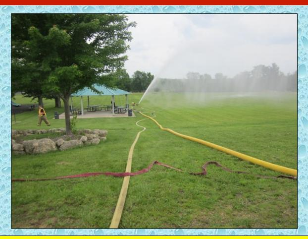
At the 44-minute mark, all four dump tanks were full of water and the flow was moved to 1,000 gpm.
