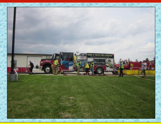
As additional units arrived, the dump site operation grew. The plan was to aim for a flow of 1000 gpm while drafting from both side suction inlets on Engine 51.
