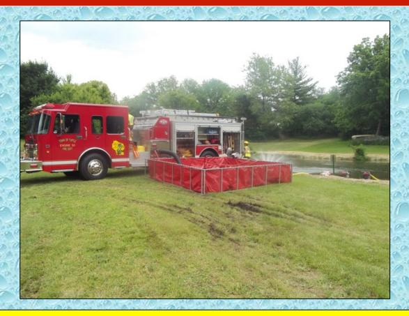
Eventually, two portable pumps were used to aid Engine 50 in the water supply process.
