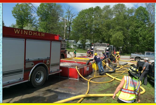
A few of the tankers could only dump off the rear of the rig. Windham's rig is seen here backed up to the last tank and dumping off its rear chute.
