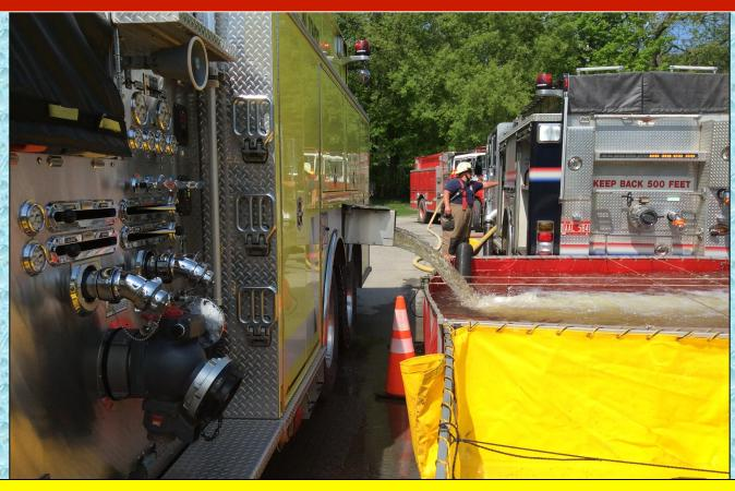
The black line on the dump chute is the water level mark at which the driver closes the valve and heads for another load of water.
