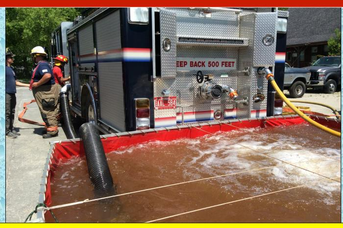
Weston Engine 1 (1500 gpm) had plenty of pump capacity to support the fire flow demand and supply the water transfer devices. A second, 6-inch suction line was added around the 37-minute mark and flow was moved to 750 gpm.
