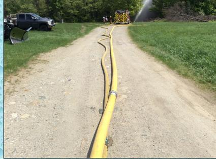
All water for the entire drill was supplied by Weston Engine 1 (dump site) pumping a 4-inch and a 2-1/2-inch supply line (500 ft) to Londonderry Engine 1.
