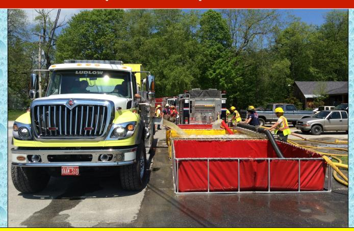
Ludlow Engine 3(3000 gal) offloads its water. Dump site operations have now moved to a 3 dump tank operation.
