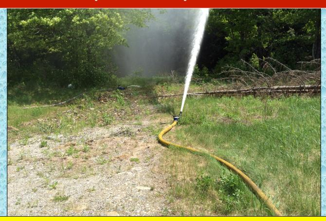
A 250 gpm flow was started at the the 5:00 minute mark using Engine 1's tank water.
