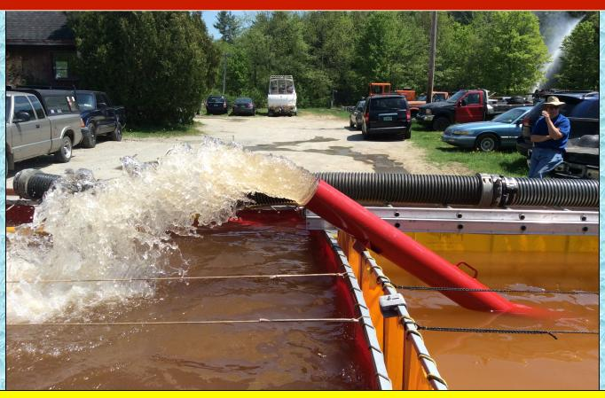
A 6-inch, Kochek Holley Transfer Pipe was the first water transfer device deployed and worked fine in moving water between the first two dump tanks.
