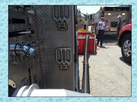
Folks set-up the dump site in a "single-lane" arrangement and used a Fol Da Tank suction elbow to facilitate drafting from the rear of Weston Engine 1.
