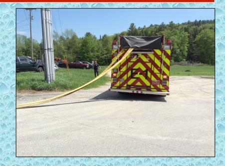
Londonderry Engine arrives on the scene and lays dual lines (4" and 2-1/2") in preparation for operating as the attack pumper. Meanwhile, Weston Engine 1 arrives on the scene and begins work on setting up as the dump site pumper.
