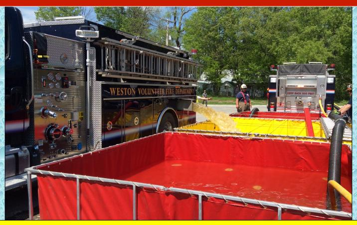
Weston Tanker 1 (2000 gal) side dumps its load of water. The single lane tank arrangement made tanker off-loading operations very easy for the side dumping tankers.
