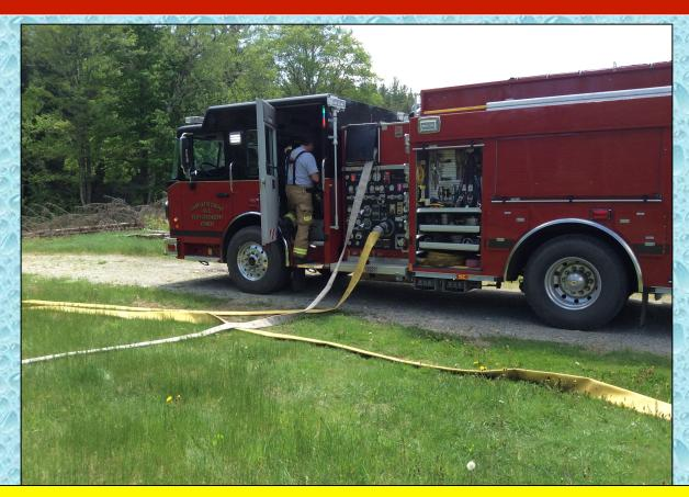
Once in position, Londonderry Engine 1 goes to work as the attack pumper and the crew deploys a TFT Blitzfire. A second Blitzfire is eventually deployed to support higher total flows.
