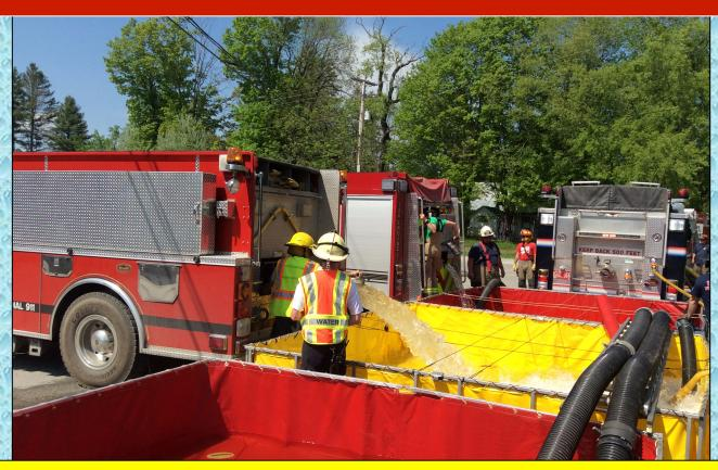
At one point, only rear dumping tankers had arrived at the dump site; this posed a positioning problem. However, once a side dumping tanker arrived the rear dumping tankers were moved out of position to allow the side dumpers access to the tanks. The process was well-orchestrated and did not prove a problem.
