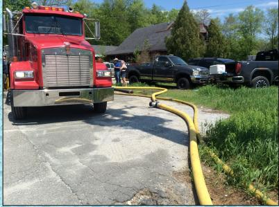
Meanwhile, back at the dump site crews worked to build out a dump tank operation and supply a 4-inch "rural hitch" feeding the attack pumper. Flow was moved to 500 gpm at the 15-minute mark.
