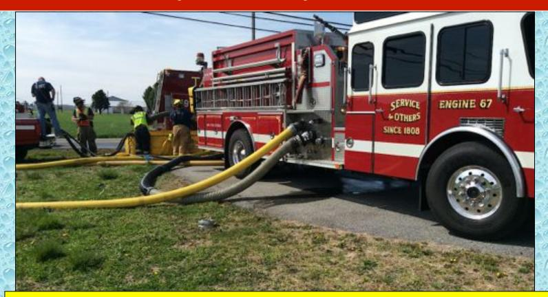
At the 102-minute mark, a second, 6-inch suction line was deployed by Engine 67 which allowed the intake flow capacity to increase which allowed output to increase 1760 gpm at the 105-minute mark.
