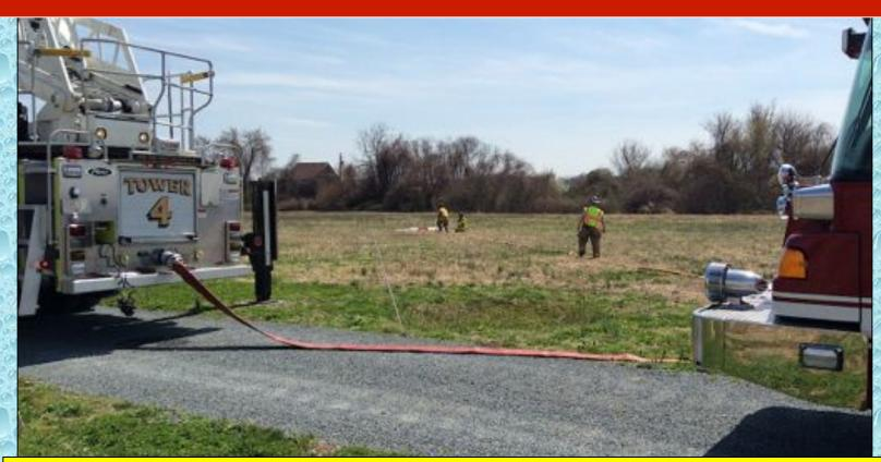
A 250 gpm water flow was started from Engine 85 at the 5-minute mark using a Hose Monster flow diffuser. Flow was never interrupted for the remainder of the drill. Meanwhile, Engine 54 stretched a supply line to Tower 4 in preparation for transition to a large flow.
