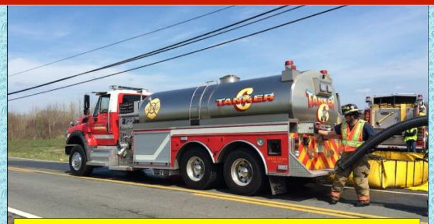
Sudlersville Tanker 6 dumps its 3500 gallons while crews remove more suction hose in order to further expand dump site operations.
