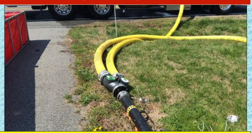
The nurse tankers supplied the double-clappered siamese which in turn supplied Cordova Engine 54.
