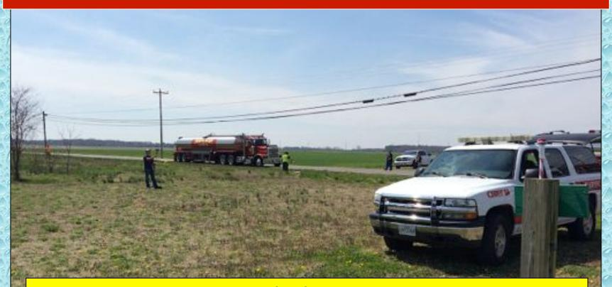
Easton Tanker 61 arrived not long after flow was moved to 500 gpm around the 15-minute mark. Thus far, all water supply operations were using a nurse tanker operation supplying a double-clappered 5-inch siamese.
