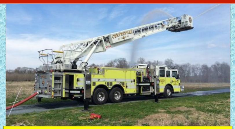
At the 75-minute mark, flow was moved to 1430 gpm. Tower 4 was used to disperse the water and had been in use since the 750 gpm flow mark.
