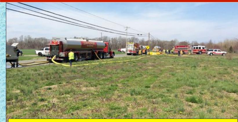
Flow was increased again at the 60-minute mark to 1250 gpm. Goldsboro Tanker 706 (6400 gal) was now being used as a nurse tanker. However, it supplied the primary dump tank by using a flow diffuser directly into the tank.
