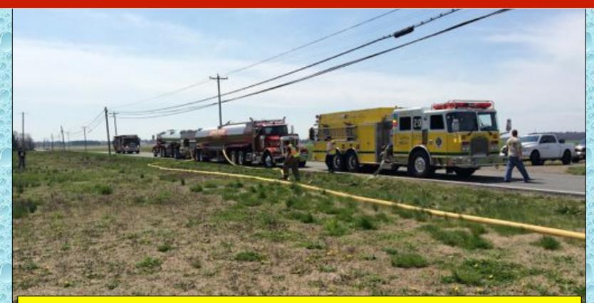
At the 28-minute mark, flow was moved to 750 gpm using a combination of a dump tank operation and a nurse tanker operation.
