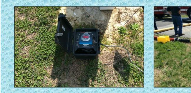
A flow meter (calibrated) was placed in-line after the siamese as the means by which all flows would be recorded.
