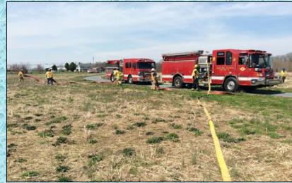
Centerville Tower 4 was pre-positioned before the drill began so that water flow could be measured once the flow became large. Queen Anne-Hillsboro Engine 85 arrived first and the crew stretched a 2-1/2-inch attack line for initial flow. Cordova Engine 54 arrived next and laid a 5-inch supply line from the park's entrance. The intent was for Engine 54 to assume the attack engine operation once the dump site was established.
