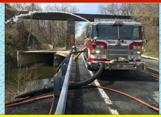
Denton E302 drafts using dual, 6-inch suction lines and loads tankers at a rate of 1500 gpm.
