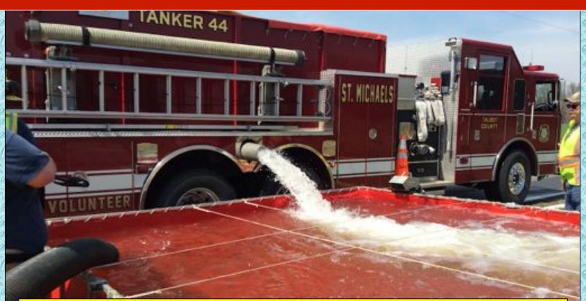
At the 41-minute mark, flow was moved to 1000 gpm as the dump site was now fully-operational.
