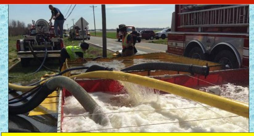
Brush 87 was brought in to help run jet siphons so that the dump site pumper could focus on supplying the 1760 gpm to the aerial tower. The 250 gpm brush truck was able to support two jet siphons.
