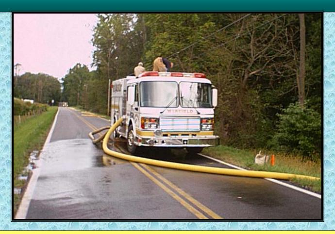
Winfield Engine 141 (1,500 gpm) receives water through 2,000 ft of 5-inch and pumps it out through 1,500 ft of 5-inch to Mt Airy VFC E12
