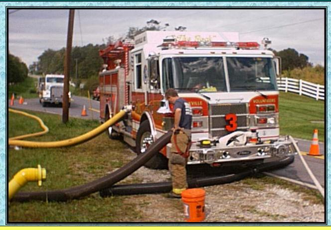
Rockville VFD Rescue Engine 703 drafts from a pond to support the relay. The dry hydrant seen in the lower left of the photo was defective.
