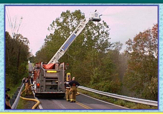
Walkersville Quint 11 (1,500 gpm) serves as the attack engine in this drill and is supplied by Mt Airy E12 through 100-ft of 5-inch hose.
