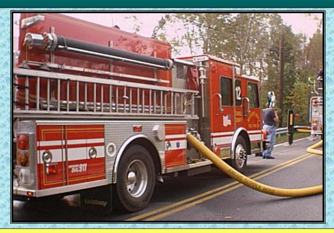
Mt Airy Engine 12 (1,250 gpm) is the final relay pumper. It is supporting Walkersville VFD Quint 11 through 100 ft of 5-inch LDH.
