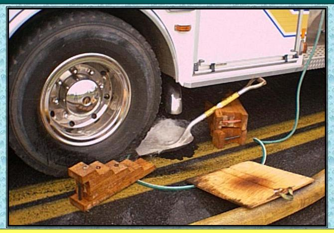
Exhaust heat from E141 proved a little problematic for the pavement and hose – both had to be shielded.
