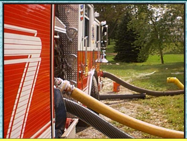
RE703 uses its 2000 gpm capability to take suction through two suctions and pump through 900-ft of 5-inch hose to Westminster E32
