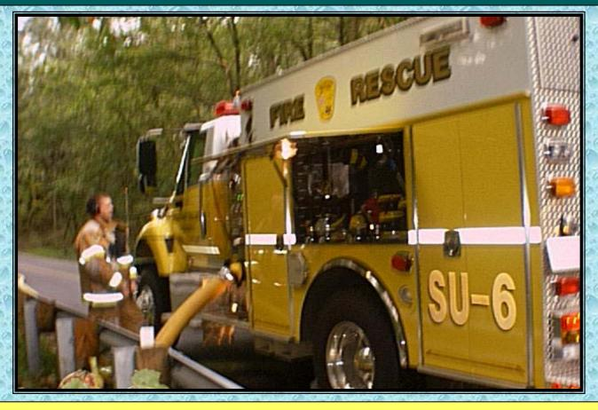
Special Unit 6 (1,500 gpm) operates as the second relay pumper. It takes in water from a 1,500 ft lay of 5-inch and then pumps it to Winfield VFD E141 via 2,000 ft of 5-inch hose.
