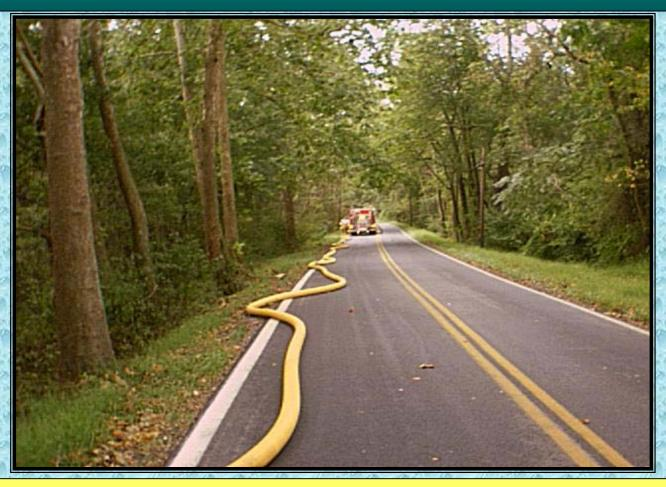
900 feet of 5-inch LDH is laid between the supply pumper and the first relay pumper.
