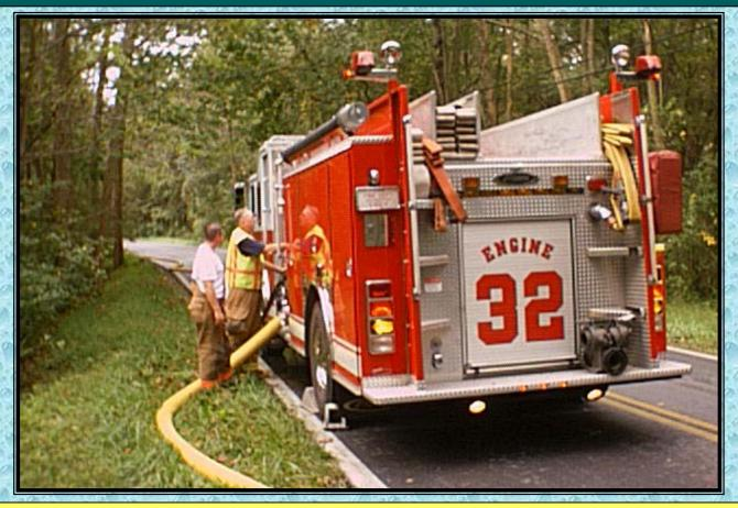
Westminster Engine 32 operates as the first relay pumper and moves the water along through 1,500 feet of 5-inch LDH to Pleasant Valley VFC SU6
