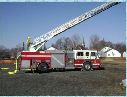
Fayette and Ovid crews work feverously to get the water supply set up before the 5-minute mark arrives. A 5-inch supply line is used to supply the quint.
