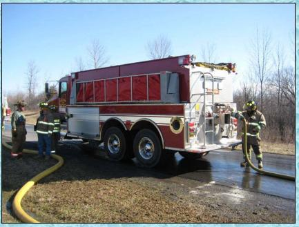
As operations progress, Rescue Engine 1141 establishes a 2<sup>nd</sup> fill line using 4-inch hose. This allows one tanker to be filled while a second tanker gets connected and stands ready.
