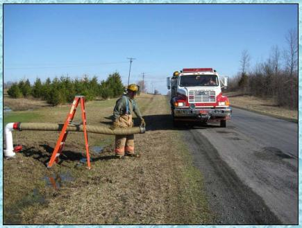
One person and a step-ladder helped make the suction hose connection: this is rather ingenious. The ladder is carried on the rescue engine and was used here to help hold the hose in the correct position so one person could thread on the coupling.
