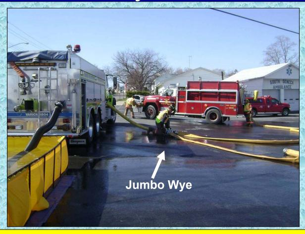
The operator of Engine 1503 uses the 2,000 gallons from his onboard tank and the 2,100 gallons from the portable tank to fill tankers as they arrive at the site.
