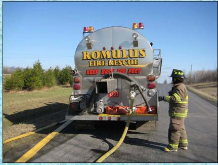
Romulus Tanker 1321 was the first tanker to arrive and the crews had to use a section of 3-inch hose to fill it because they did not have an LDH line ready to go. This first fill time was a bit slow but the switch to LDH soon made a difference.
