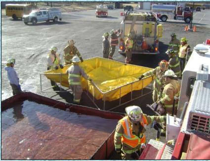
Around the 4-minute mark, Ovid Engine 1104 arrives and dumps its 1500 gallons. The crews grab the engine's dump tank and set-up it also.
