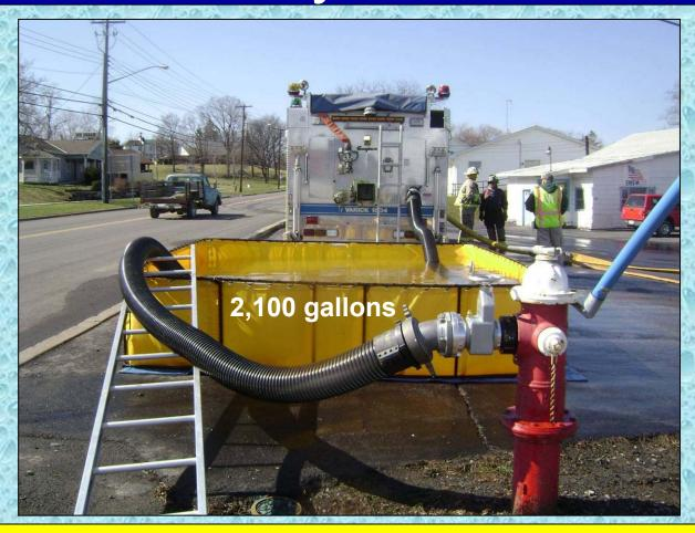
Engine 1503 uses its rear suction to draft from the portable tank and then pumps a 5-inch hose to a jumbo wye.
