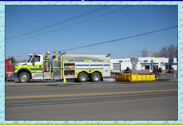
Varick Engine 1503 (1500 gpm/2000 gal) was part of the 1<sup>st</sup> Tanker Task Force and responded to a fire hydrant in Ovid to set-up a second, tanker fill site. Because the hydrant had a flow less than 800 gpm, a 2,100-gallon portable tank was used to facilitate the tanker loading operation.
