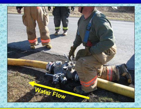
The fill site crews worked quickly to get a 5-inch fill line in place. A LDH manifold is shown here being used to control the flow of water into the tanker. The manifold is reversed so that the 2-1/2" outlet can be used to drain/bleed off pressure.
