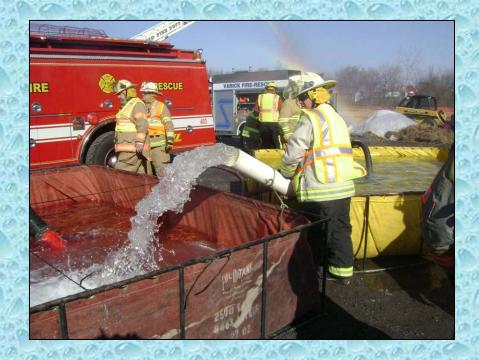
With water now flowing, the transfer of water between tanks is critical to success. The PVC jet siphon appears to be working quite well.
