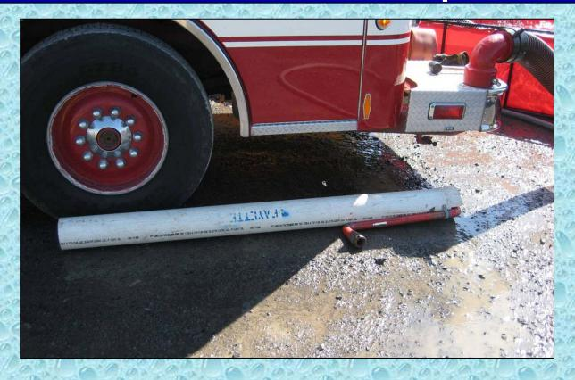
This homemade jet siphon consists of a section of 6-inch PVC pipe and a section of 1-inch steel pipe. Using this style of jet siphon can free up suction hose for other uses in a tanker shuttle operation.
