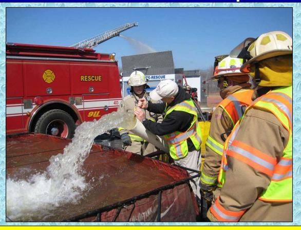
An attempt was made to pitot the 6-inch PVC pipe to see if the flow could be measured. Unfortunately, no reading could be obtained. However, for reference, 1 psi from a 6-inch opening equals 1069 gpm using Freeman's formula for flow from a smooth bore nozzle/opening!!!
