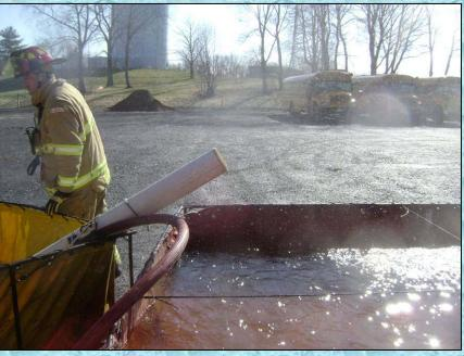
Varick Rescue 1544 is shown above being used to run two of the jet siphons. The unit established its own draft and pumped the jet siphons which allowed the dump site engine to dedicate all of its pumping capacity for supplying the quint.
