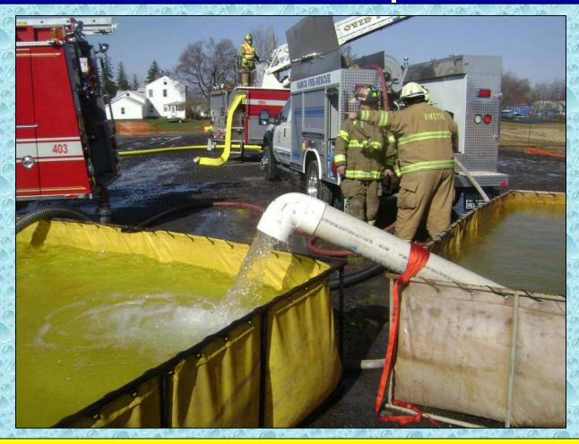
If needed, a 90-degree elbow attachment can be used on the 6-inch PVC jet siphons to help direct water discharge.
