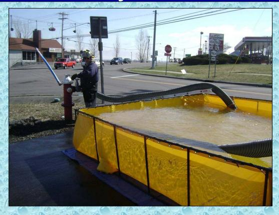
When filling operations begin, one person operates the hydrant valve with the responsibility of keeping the dump tank as full as possible. Doing this allows the engine to fill tankers at a rate of 1,000 gpm even though the hydrant supports only about 800 gpm.
