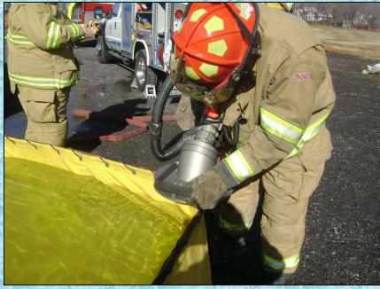
With three dump tanks now set up, jet siphons are needed so that water can be transferred to the primary drafting tank. A homemade PVC jet siphon is shown above being placed into operation.
