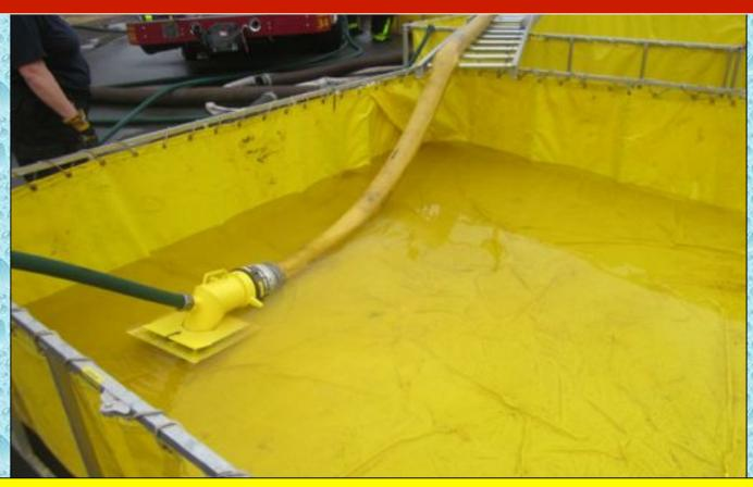
The folks tried using a short length of 5-inch LDH in place of suction hose to transfer water. An adaptor was needed, and water was transferred from the 4<sup>th</sup> dump tank into the primary dump tank. It seemed to work okay.
