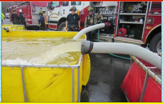
At the 35-minute mark, the flow was moved to 750 gpm as conditions at the dump looked stable.
