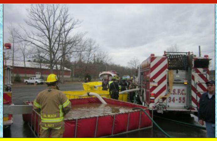
At the 15:24-minute mark, a third dump tank was brought on line and flow was being maintained at 500-gpm.
