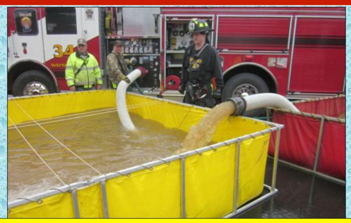
By the 10:00-minute mark a second dump tank was brought on line. Notice the good looking, solid stream of water coming from the jet siphon. This is the type of flow we want to see when transferring water between dump tanks.
