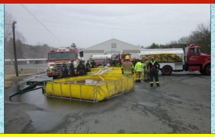
By the one-hour mark, four dump tanks were in operation and the flow was moved to 1,000 gpm. Two fill sites were up and running and the operation had stabilized.
