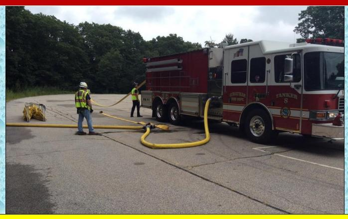
The drill began with executing a "rural hitch" operation to a simulated attack pumper. Stratham Tanker 8 arrives first and begins pumping off its 3000 gallons of water into the clappered-Siamese.
