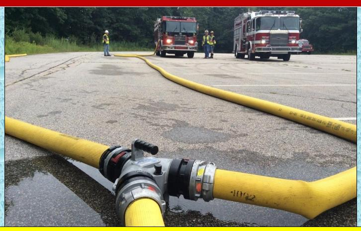
New Market Tanker 4 (3000 gal) was next to arrive around the 5-minute mark and connected to the other side of the siamese and prepared to take over rural hitch operations once Tanker 8 was empty.
