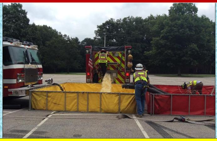
At the 20-minute mark, the first load of water was dumped into a dump tank and the transition to dump tank operations was complete. Flow remained at 500 gpm.
