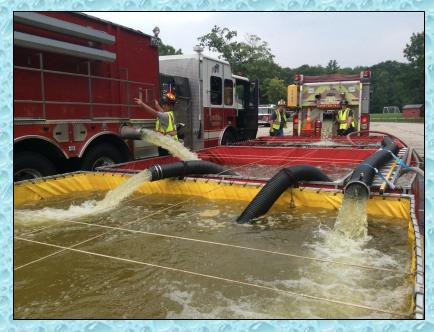
Engine 3 was eventually able to get three suction lines in operation and support two jet siphon devices. A peak flow of 750 gpm was achieved during the last 20 minutes of the drill.
