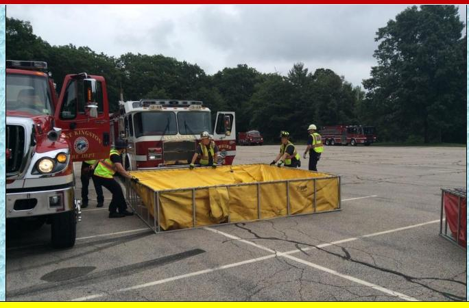
Engine 3's (1500 gpm) crew begins setting up for dump tank operations. Water flow was moved to 500 gpm at the 10:45 minute mark using the rural hitch.
