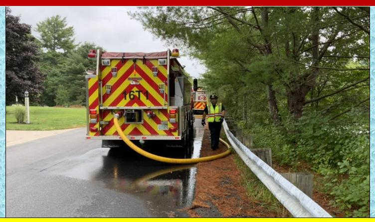
All of the tankers loaded using 4-inch LDH which helped keep the turn-around time relatively short at this loading site.
