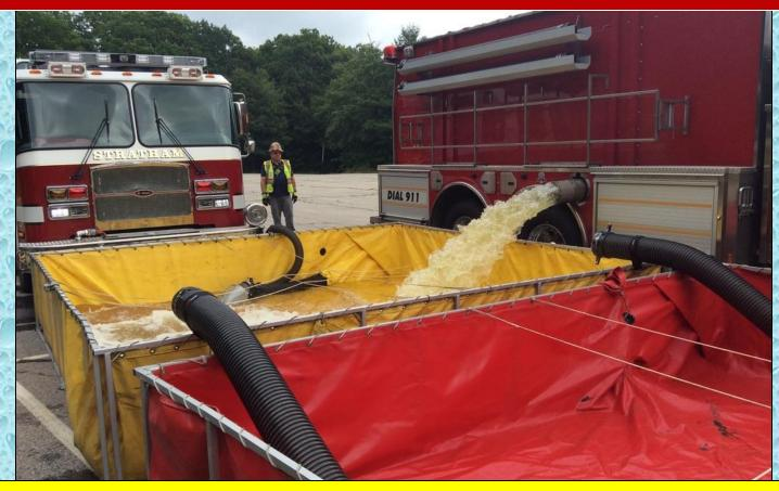
As tankers arrived at the dump site they no longer pumped the rural hitch; they all dumped their water into dump tanks.
