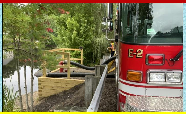
East Kingston Engine 2 (1750 gpm) took suction at the dry fire hydrant and loaded tankers using 4-inch LDH
