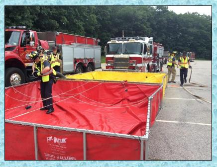
Crews were able to get two, 3000-gallon dump tanks down in a "single-lane tank" arrangement.
