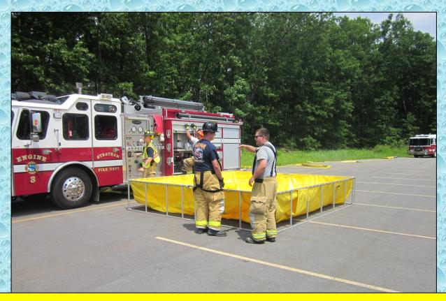
When Stratham Tanker 8 arrived on the scene, its 3,000-gallon dump tank was removed and placed next to Engine 3. The position of the dump tank was changed soon after, because the folks wanted to simulate a more congested area.
