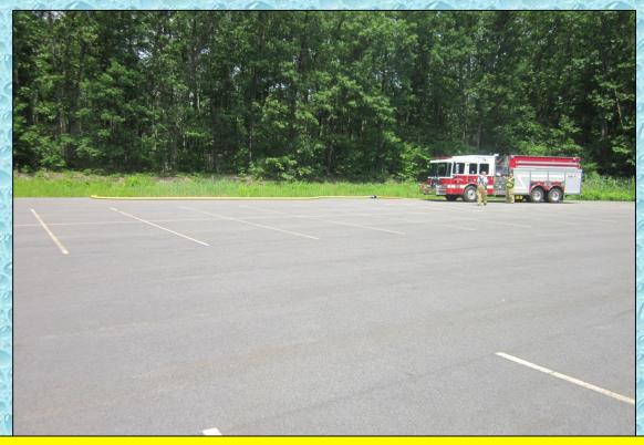
Stratham's Tanker 8 made a huge difference in the early stages of this drill by operating as a nurse tanker. The unit's 3,000 gallons of water in conjunction with the attack engine's 1,000 gallons allowed for enough time to build out the dump site without the stress of immediately needing water.
