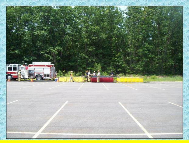
The arrangement of tanks was a bit different but it worked out just fine and flow was not restricted because suction was taken using the driver side suction inlet.
