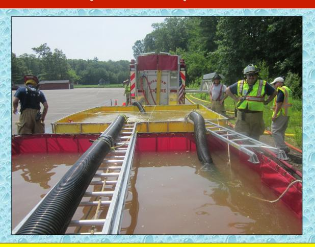
With a final change in strainers and the reconfiguration of the jet siphons – the flow peaked at 900 gpm. Flow seemed most stable at around 750 gpm.
