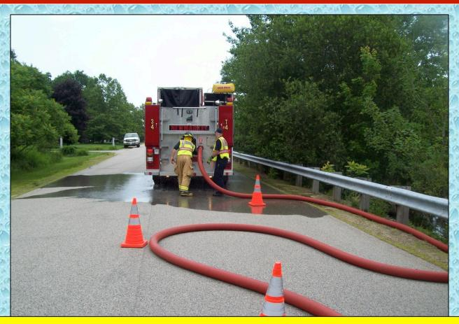
4-inch LDH was used to fill the tankers with an average fill rate in the neighborhood of 950 gpm to 1100 gpm.
