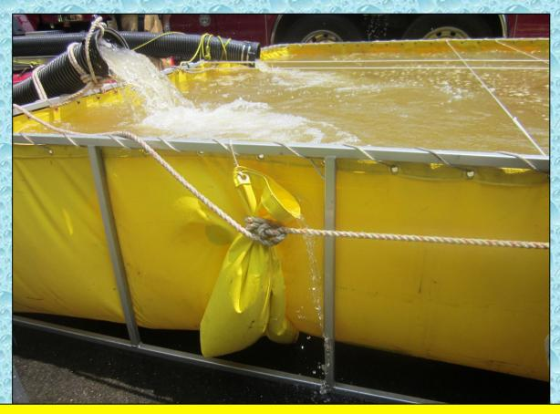
Drains that still use rope as their securing mechanism need to be tied up on the inside of the tank in order to reduce the "mess" created when they spill over.
