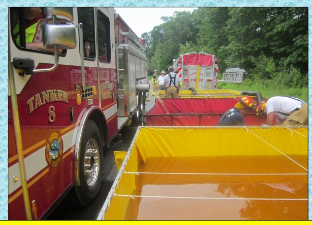
With the dump site now operational, Tanker 8 broke free from nurse tanker ops and dumped the remainder of its first load of water into the dump tanks.
