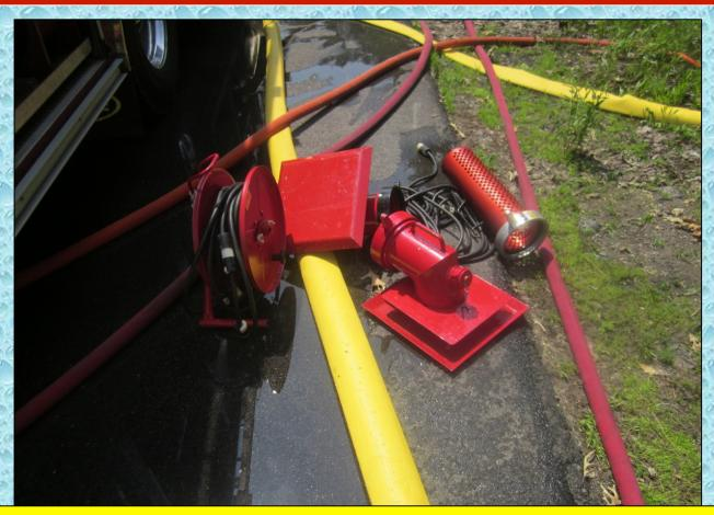
The bottom line is that strainer selection is critical to the success of a dump tank operation. Each strainer shown in this photo had a different flow limit.
