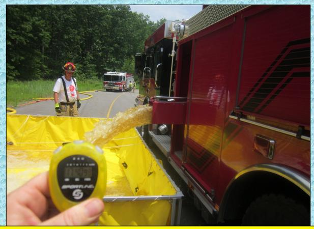
At around the 18-minute mark, New Market's tanker arrived and the operation transitioned to a dump site operation. The flow was also increased to 500 gpm.
