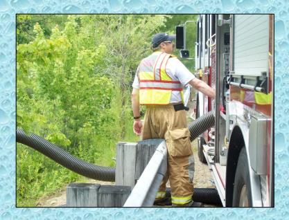
The second suction line was able to be added without having to shut down the operation - once again showing the value of outfitting a pumper with suction inlet control valves.
