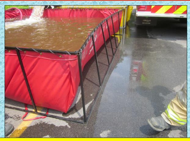
When setting up a dump tank, be sure to take a moment to straighten out the tank material – otherwise uneven loading can occur as shown in this photo.
