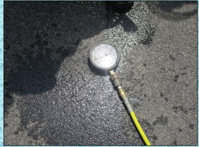
At the 5-minute mark, water flow was started at 280 gpm using a Hose Monster flow diffuser for flow measurement. The diffuser was supplied by a 100-ft section of 5-inch LDH from Engine 3's high-flow discharge.
