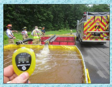
At the 50-minute mark, water flow was moved to 750 gpm and jet siphons were re-configured to improve flow. A ladder and additional suction hose were used to "jump" the red tank.
