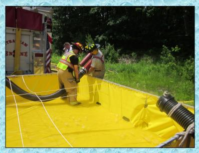
When attempting to raise the flow above 750 gpm, the low level strainer proved problematic. The first strainer seemed to peak at around 950 gpm (750 gpm plus two jet siphons). Water flow was interrupted whiles crews tried other strainers – without much success
