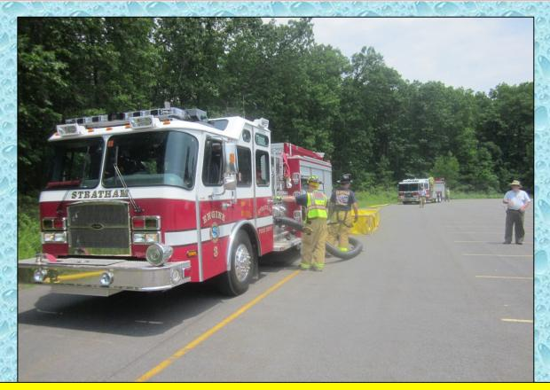
Tanker 8 – with its 2,000 gpm pump – supplied water to Engine 3 via 300-feet of 5-inch LDH until such time that the first dump tank could be placed into operation.
