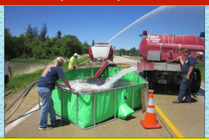
A two-dump tank operation was used to support the drill. Aurora Rescue Engine 1 (1250 gpm) drafted using a single-lane tank arrangement. Stanley Tanker 514 (2500 gals) is seen dumping water into the 3,200-gallon Fol-Da-Tank Type II SLT.
