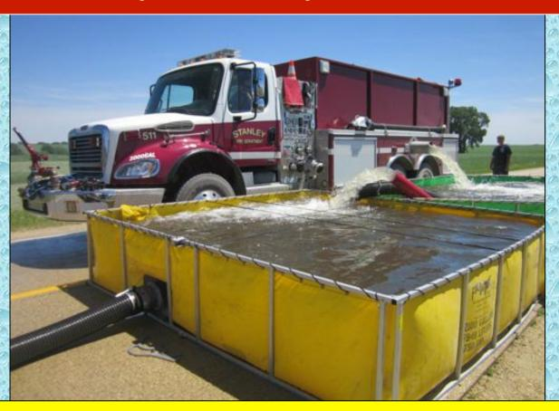
Four tankers were used to haul water during the drill. Water flow was started at 500 gpm and peaked at 800 gpm for the last 20 minutes of the drill.
