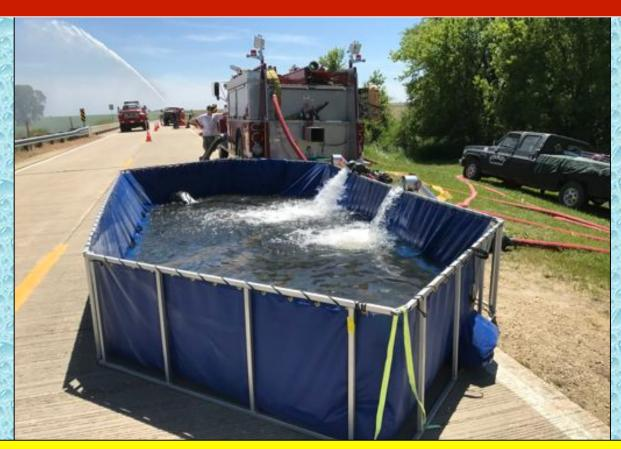
Engine 511 (1,000 gpm) then drafted from the open-relay set up and supplied water to a loading station that then filled tankers. This arrangement allowed tankers to be loaded at close to 1,000 gpm.
