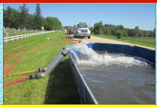
The portable pumps supplied water to a 3500-gallon dump tank. Lift to the dump tank was over 14-ft...so this diminished the flow ability of the pumps some.
