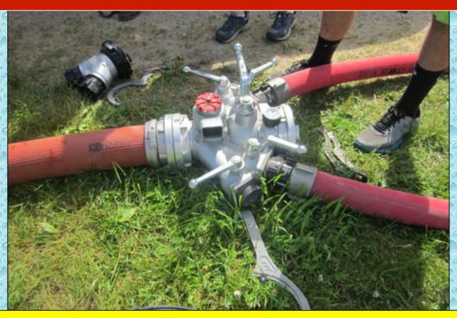
An LDH manifold was supplied by Engine 511 and tankers were loaded from that point. The goal of the loading operation was a 1,000 gpm fill rate.
