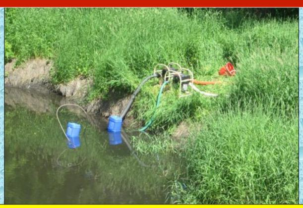
Two portable pumps were used to complement the Turbodraft device at first. However, the pumper was unable to support the Turbodraft and load tankers at the same time, so two additional portable pumps were brought on line and the Turbodraft operation was discontinued.
