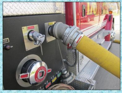
A short length of 6-inch hose was used to feed the relay valve. The hose was connected to the high-flow discharge – however, it was unclear if the discharge was capable of full-capacity.
