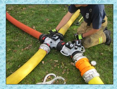
Manchester Engine 176 (1250 gpm) was the first relay pumper and it was located at the end of the 6-inch hose lay. A Task Force Tips Oasis valve was used as an in-line relay valve. An in-line gauge (orange) was also used to measure friction loss.
