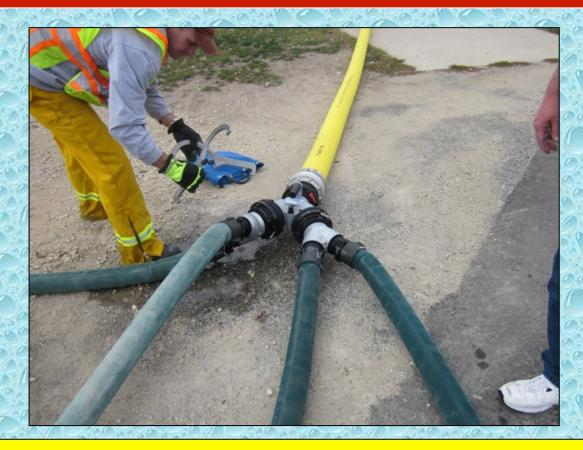
Because Engine 3 did not have a high-flow discharge, four, 3-inch lines were used to supply a jumbo siamese via two smaller siamese fittings. Again – not a perfect situation, but it worked just fine.
