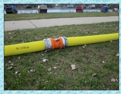
An in-line pressure gauge was used around the 1000-ft mark in the 6-inch hose lay so that friction loss could be observed. Even at the highest flow point, there was very little (<20 psi) friction loss in the entire length of 6-inch hose!
