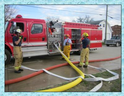
Palo Engine 344 (1250 gpm) was used as the second relay pumper. It too connected to a TFT Oasis valve. The pumper had a throttle problem and never was able to support the operation.
