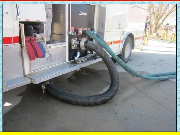
The driver side suction was run underneath of the pumper. Thirty feet of 6-inch suction hose was needed to reach the water – but the operation worked just fine.
