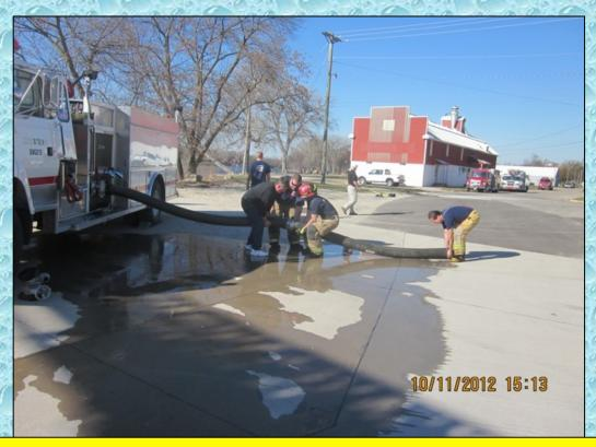
The drill started with Independence Engine 3 (1,250 gpm) establishing a water supply at the dam. The crew set up dual suctions using 30-feet of 6-inch suction hose and 20-feet of 4-1/2-inch suction hose to reach the water. Both suction lines were equipped with a barrel strainer.
