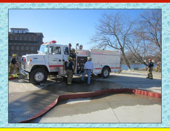
Because of the limited quantity of suction hose, the pumper was parked parallel to the water's edge and the driver side suction hose was run underneath the pumper.
