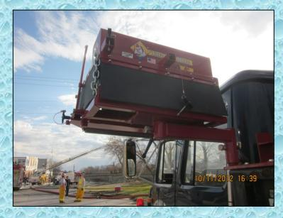
When the drill was over, it was time to pick up 3500 feet of hose! The Stanley FD had a stake body style flatbed truck that was equipped with a "Hose Mule" loading device that helped to make the loading process simpler.
