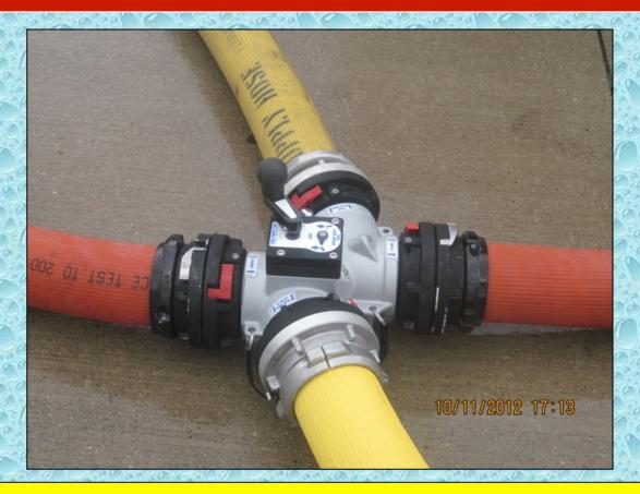
The Oasis valve is really just a newer version of the old "Z-valve" that many folks in New England carried for relay pumping operations. The Oasis valve can be used for hydrant operations and relay pumping.
