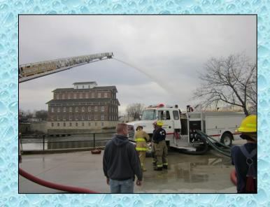
Water flow was handled at the Vinton ladder truck which was 1100-feet from the Palo pumper. At first, flow was measured through a Hose Monster flow diffuser. At the end of the drill, flow was switched to the Vinton truck.
