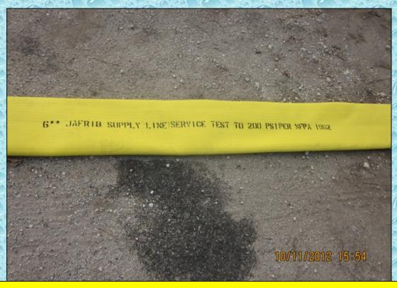
The 6-inch LDH was supplied by the Stanley FD. The hose was recently purchased as part of a large, federal grant for water supply equipment. The grant also included several thousand feet of 5-inch hose plus many LDH appliances and fittings. Six-inch LDH is supposed to be able to move 2,000 gpm.
