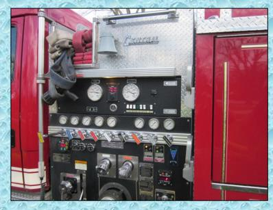
Using the relay valve makes the insertion of a relay pumper very easy. The water flow does not have to be stopped to connect the pumper. Once all of the hose is connected – it is simply a matter of opening one valve.
