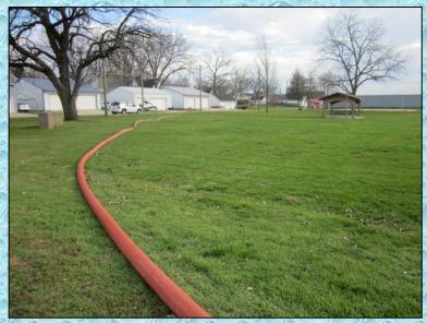
From Engine 176, the water traveled down 1100-feet of 5-inch hose to Palo Engine 344 – which served as the second relay pumper.
