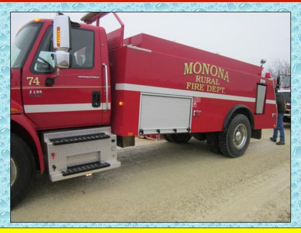
An interesting feature of the Monona tanker is that the tank body can be lifted about 18-inches in the front – this helps offload the water faster as the level in the tank gets lower.
