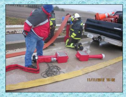
Because of limited access for pumpers, the decision was made to use three, Turbo Draft devices to supply water back to a dump tank from which the second pumper would draft and then fill tankers.
