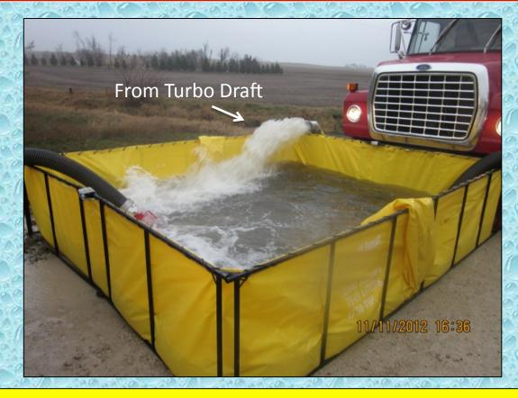
With the dump tank now being filled, the tanker loading operation could be started.
