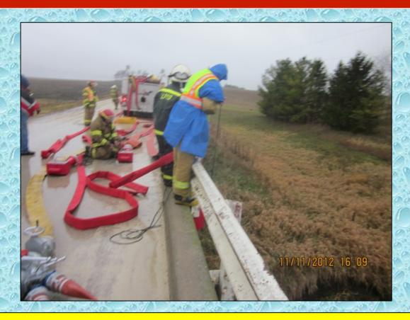
The Turbo Drafts are lowered into the creek one at a time.
