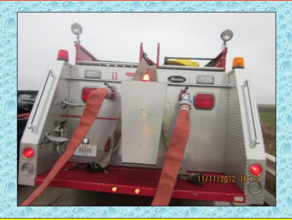
Monona's 2,000-gallon tanker is ready to be loaded using dual, 4-inch fill lines.
