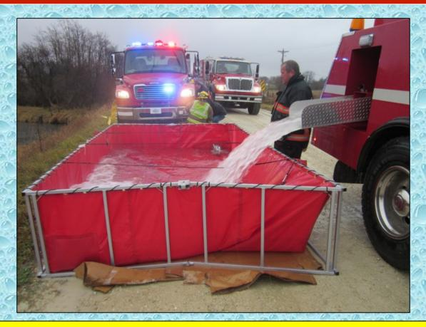
The 2,000-gallon rectangular dump tank fits nicely along the narrow road and in front of the pumper.
