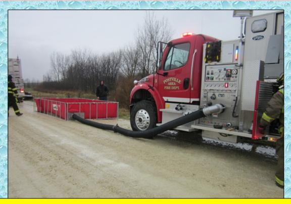
Along with the single-lane dump tank, a special suction hose connection was provided that allowed suction hose to be connected directly to the tank. In conjunction with using the suction elbow, this feature keeps the suction hose out of the roadway.
