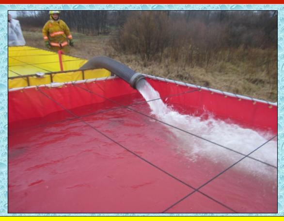
Because the two dump tanks were about 20 inches apart, the suction hose worked better than the Holley Tube – which required the tanks to be closer together.
