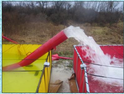
An 8-inch Kochek Holley tube was used as the initial transfer device for moving water from the second tank to the primary tank.
