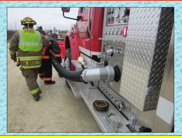
The new dump tanks are rectangular in shape – thus allowing them to be placed in front or behind a pumper. The suction elbow helps reduce the width "profile" of the operation.
