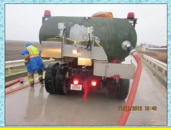
Stanley's 2,500-gallon tanker is filled using a single, 4-inch fill line through a Fireman's Friend check valve.
