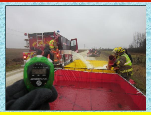
At the 12:55-minute park, water is dumped into the second tank and it is time to commence water transfer operations.
