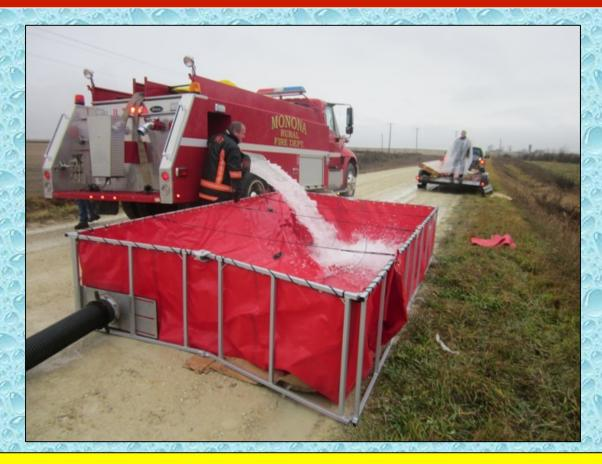
With the first dump tank in position. Monona's tanker offloads its 2,000 gallons of water.
