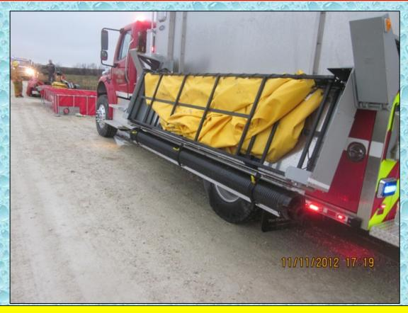
The decision was made to change out the Holly Tube for a jet siphon and suction hose arrangement. A length of 6-inch suction hose was taken from the Postville pumper.
