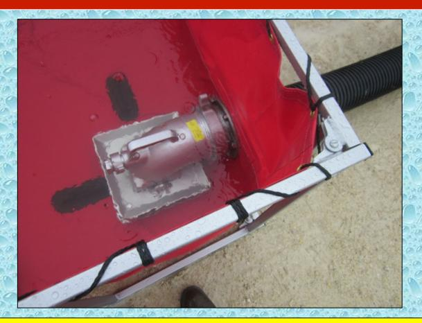
On the inside of the dump tank, a low-level strainer is attached to the pass-through fitting.
