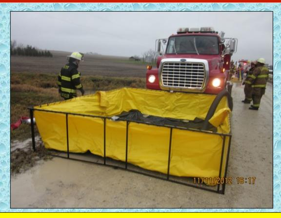
A dump tank was set-up so that the Turbo Drafts could dump water into the tank and the fill pumper could draft and fill tankers.
