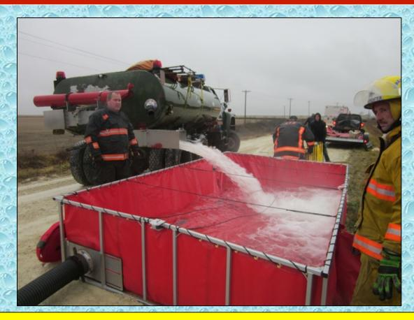
At around the 9:30-minute mark, Stanley FD's tanker arrives and offloads its water while the dump site crew works to set up a second 2,000-gallon dump tank.
