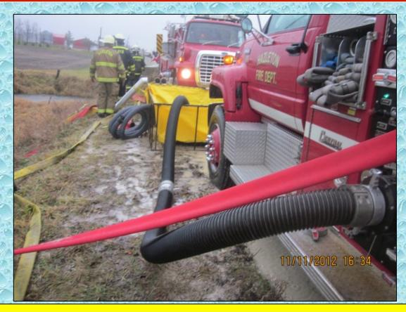
Two pumpers shared the same dump tank. The pumper in the foreground (Hazelton) operated the Turbo Draft devices.
