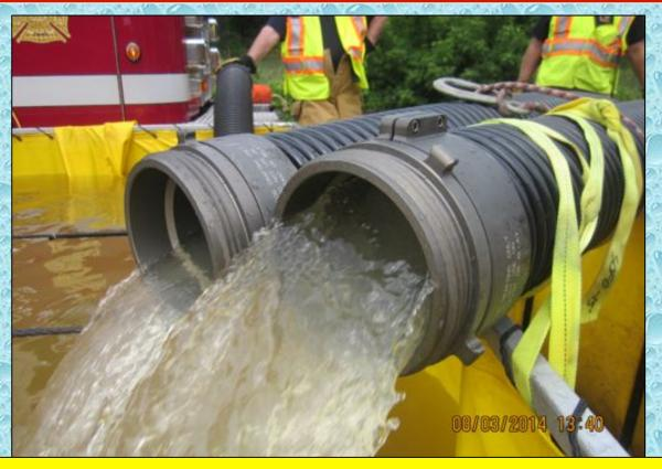
As the number of jet siphons increase, so do the pressure and capacity demands that are placed on the pumper. These two jet siphons are moving water – just not as much as they can. There needs to be a "full" stream coming out of each suction hose. When pressure was increased – the flow got much better.
