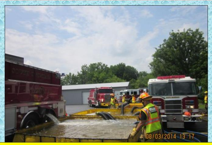
Otisco Tanker 1 is shown arriving with its second load of water. Three dump tanks are down but only two are in operation at this time.
