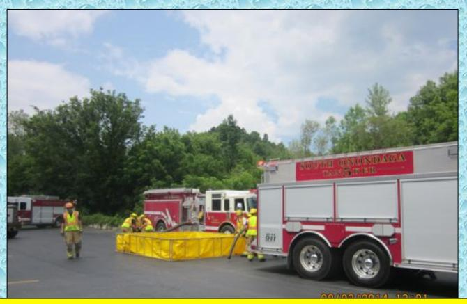
The crews quickly went to work getting the first dump tank set up before water flow had to be started. The plan was try and avoid using a nurse tanker operation.
