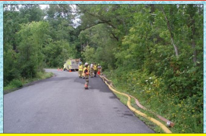
Because of the somewhat narrow road and the pumper having to set up on a curve, the 4-inch lines were run to the rear of the pumper and were built in staggered lengths to allow tankers to position without blocking out others.
