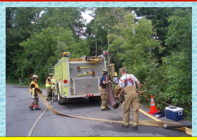
Some of the crew members help set up for drafting out of the creek while others help get the two, 4-inch lines ready for tanker loading.
