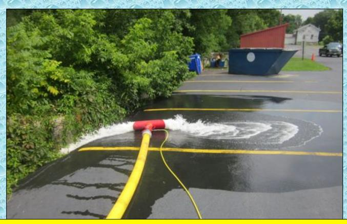
At the 5-minute mark, water flow was started at 250 gpm using Engine 6's on-board tank water for about 30 seconds and then the operations transitioned to drafting from the dump tanks.
