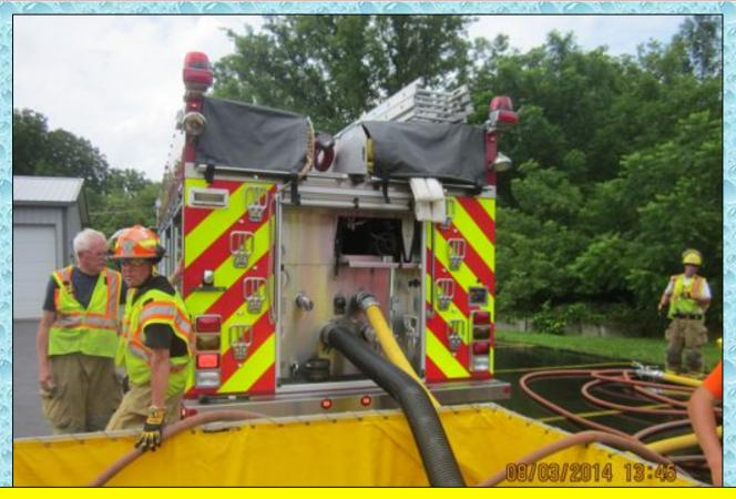
Otisco Rescue Pumper 2 drafts from the third dump tank and supports two of the four jet siphons. By inserting this pumper into the operation, flow was able to be increased to 1,000 gpm.
