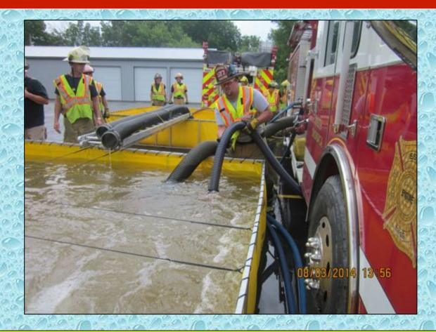
To assist with the 1,000 gpm flow, Engine 6 added a third suction line using 2-1/2-inch suction hose connected to the driver's side auxiliary suction inlet.
