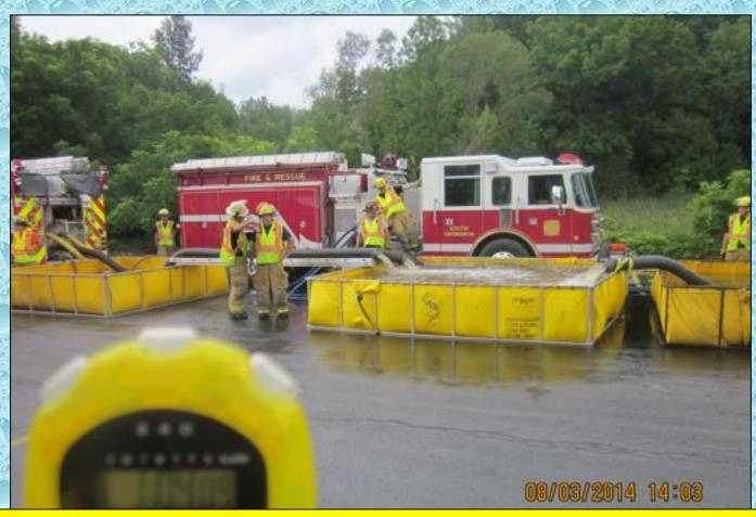
Flow was moved to 1,000 gpm without incident and the goal was to sustain the 1,000 gpm mark for the remainder of the drill.
