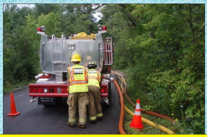
Sentinel Heights' 2,000 gallon tanker gets filled in just about 2-minutes using a single, 4-inch fill line.
