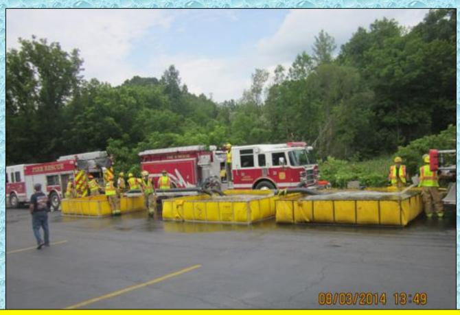
At the 50-minute mark, the three tank operation has stabilized and preparations are made to increase the flow to 1,000 gpm at the one-hour mark.
