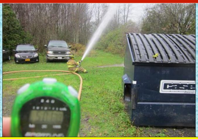
At the 5-minute mark, water flow was started at 250 gpm using a 2-1/2-inch attack line supplied by Skaneateles Engine 12's tank water.
