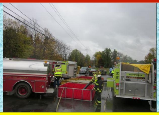
As additional tankers began to arrive, the dump site crew worked to gather additional dump tanks and equipment. The plan was to eventually move to a 4-dump tank operation.
