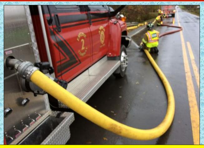
Amber Engine 2 (1,000 gpm) drafted from the creek and loaded tankers using LDH as well.
