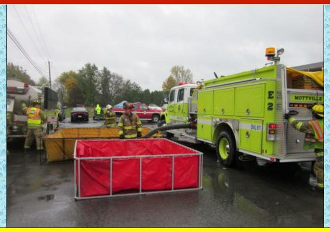
The dump site crew deployed the 2,500-gallon dump tank from the Amber tanker and began to set up for a multiple dump tank operation.
