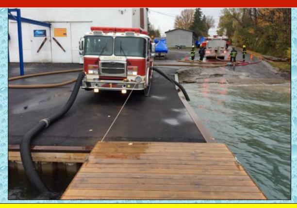
Eventually – the Marcellus crew located more suction hose and was able to increase pump capacity by drafting from both the front and officer side suction inlets. The pumper is outfitted with an MIV on the front intake which allowed for the easy addition of the second suction line.
