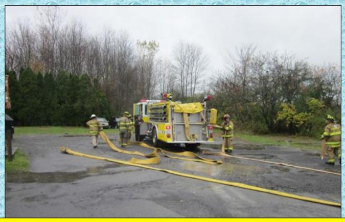
The crew quickly went to work deploying a 2-1/2-inch attack line so they could be ready to flow water at the 5-minute mark. In the mean time – the driver was preparing to receive water via the 5-inch supply line that had been laid.
