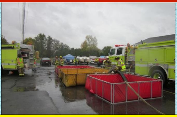
At the 9:40-minute mark, three dump tanks had been deployed and two were in operation.
