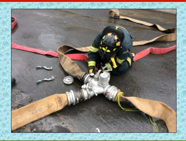
The crew used LDH to load the tankers at rates over 1,000 gpm – once again emphasizing the value of LDH in tanker loading operations.
