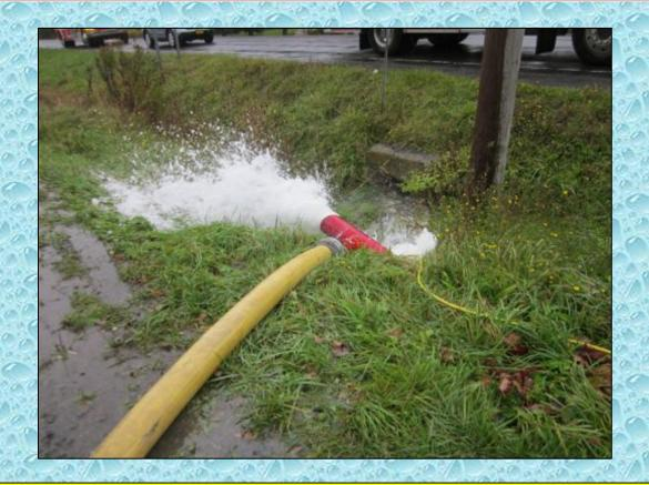
At the 15:00-minute mark, water flow was increased to 750 gpm. A Hose Monster flow diffuser with a fixed-pitot was used to accurately measure flow.
