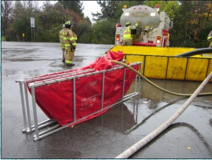
The dump site crew switched out the 1,000-gallon tank with a 2,500-gallon dump tank that arrived on one of the tankers. This allowed for greater storage capacity on the ground.
