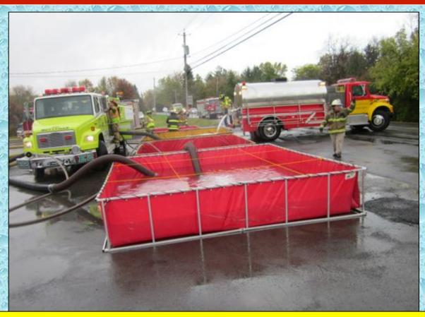
Four dump tanks are now in operation and Mottville Engine is now drafting from both side suction inlet ports. The officer side suction inlet is taking water from the red 3,500-gallon dump tank shown in the foreground.
