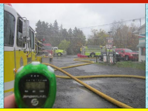
Not long after the water flow was started through the attack line, the 5-inch supply line was charged from Mottville Engine 2 to Skaneateles Engine 12 – and from then on – water flow was never once interrupted.
