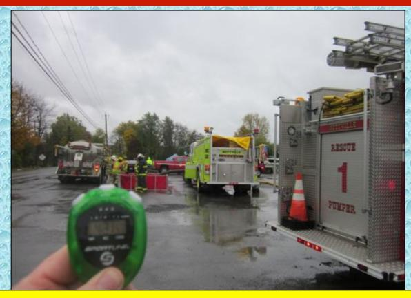
At around the 4:31-minute mark, the first dump tank was down and in position to receive water. The tank came from Mottville Engine 2 which carries a 1,000 gallon dump tank. Amber Tanker 1 (2,500 gal) is also seen in the photo – it was the first tanker to arrive.
