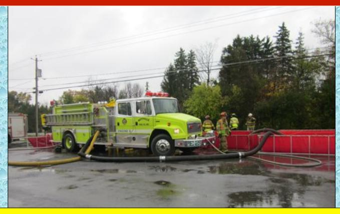
By drafting from both side suction inlets, this 1,500 gpm pumper was able to support the entire dump site operation without the need for another unit to run jet siphons. The additional suction hose had to come from other pumpers and tankers.
