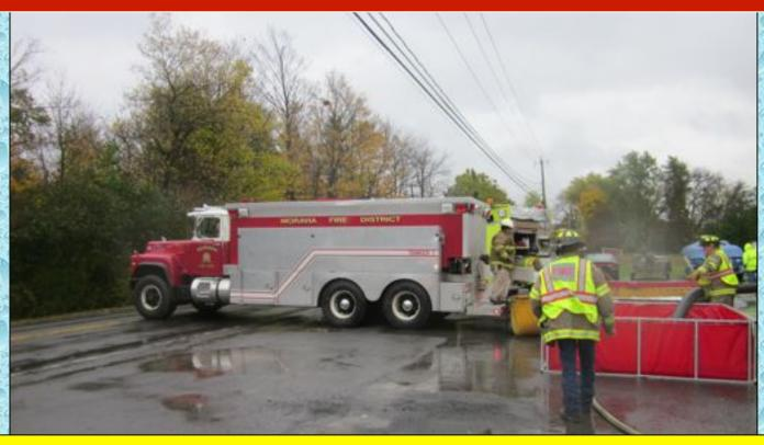
Around the 10-minute mark, the "first wave" of additional tankers began to arrive. Moravia's Tanker 1 was one of tankers on the first "Tanker Box" and is seen here off-loading. One of the problems that arose was electing to dump off of the rear – the road got blocked at times. Fortunately – that eventually was changed to a side dumping operation later in the drill.
