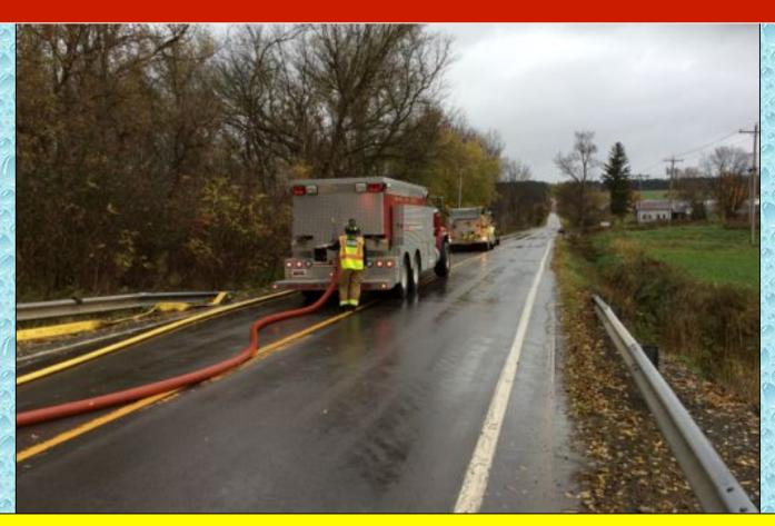
The fill site crew did a very nice job of cycling tankers through this fill site. While one tanker was being loaded, the next one was connected and ready to go once the first one was filled – thus, very little lost time.
