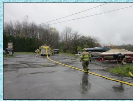
Skaneateles Engine 12 arrives on the scene as the attack engine and the timer starts once the pumper stops to lay out the supply line.
