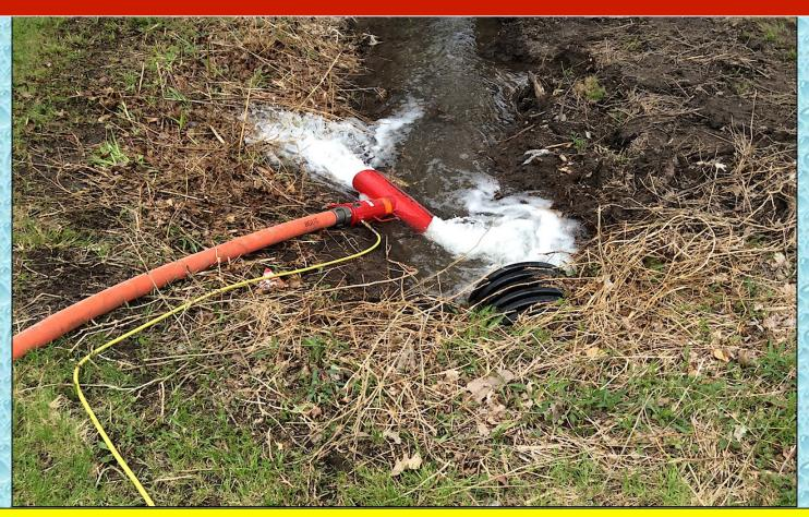
Flow was moved to 500 gpm at the 15-minute mark using a Hose Monster flow diffuser with fixed-pitot.
