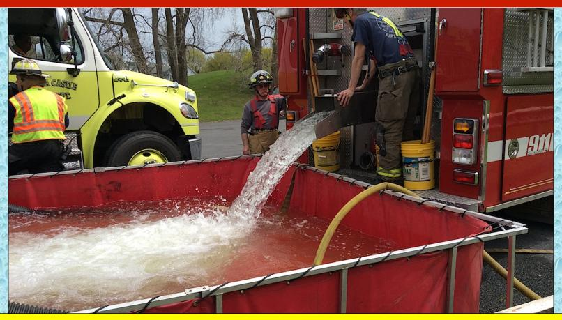
One of the tankers hauling water was a rear-dumping tanker only. The dump site officer did a good job of directing rigs so that the rear-dumping tanker could always get in position at the last dump tank.
