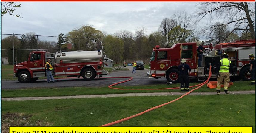
Tanker 2541 supplied the engine using a length of 2-1/2-inch hose. The goal was to support a 250 gpm attack until a dump tank operation could be established.
