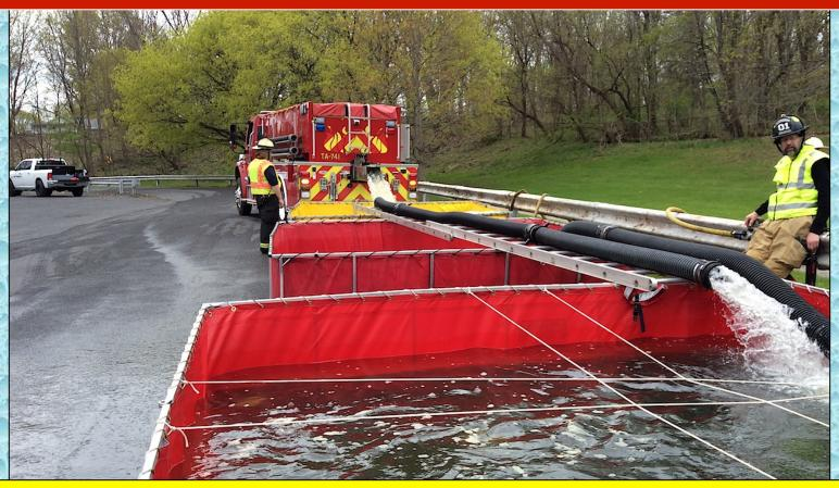
Using the three dump arrangement behind the pumper necessitated the transfer of water from the third tank to the primary tank...thus the need for additional suction hose.
