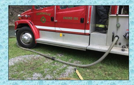
Shortsville Engine 2511 drafted out of the creek at this fill site and supplied a 300-ft 5-inch line up to an LDH manifold in a parking lot. Tankers were then loaded in the parking lot. In addition to drafting using a 6-inch suction line, Engine 2511 also located a sufficient quantity of 3-inch suction hose to add in another suction line.
