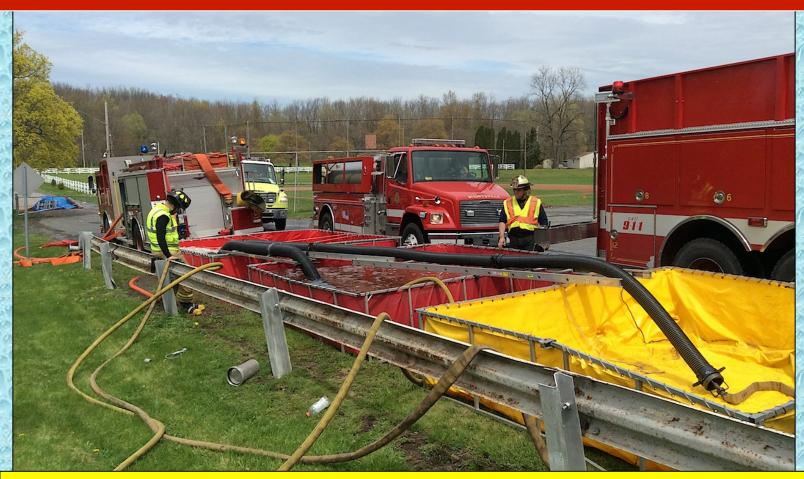
At 39-minutes, the flow was moved to 750 gpm and at the 54-minute mark, three dump tanks were down and in operation.
