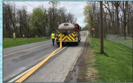
Port Gibson Pumper Tanker 2231 (1500 gpm) drafted from the same creek but used a dry fire hydrant as the supply point. They too loaded tankers using LDH.
