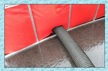
The dump site crew chose to use a "through the drain sleeve" set-up and place the dump tanks to the rear of the pumper. This arrangement allowed tankers to drive past and side dump their water.
