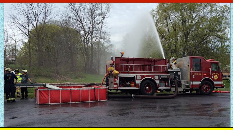
At the 92-minute mark, the dump site pumper deployed a second, 6-inch suction line and one-minute later, flow was moved to 1000 gpm and maintained for the remainder of the drill.
