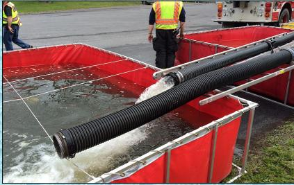
Water transfer operations became critical at the dump site. A short length of 2-1/2-inch hose was used to supply a gated wye which then supplied two jet siphons. One firefighter was assigned to control the jet siphons at the wye.
