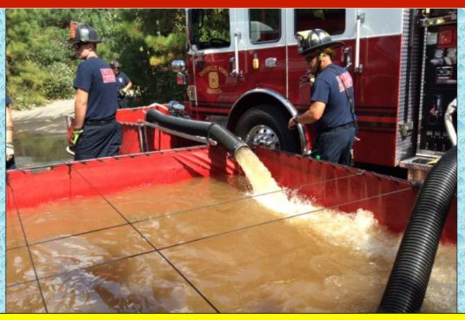
At the 59-minute mark, three dump tanks were now in operation and water flow had never been interrupted. Water transfer operations were critical to the sustained flow at this drill.
