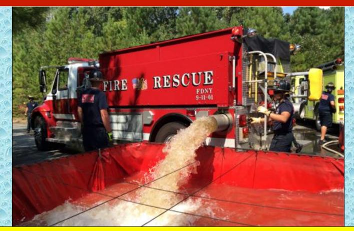
SFTFR Tanker 3 offloads its 1800 gallons of water as two dump tanks are now in operation.
