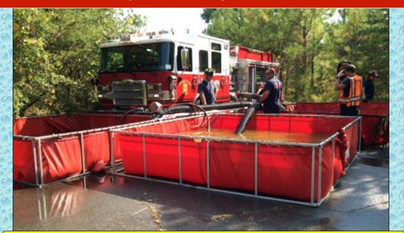
The final set-up. Three dump tanks were positioned in a tight intersection on a narrow road so that two tankers could dump simultaneously. The operation required strong oversight by the dump site supervisor.
