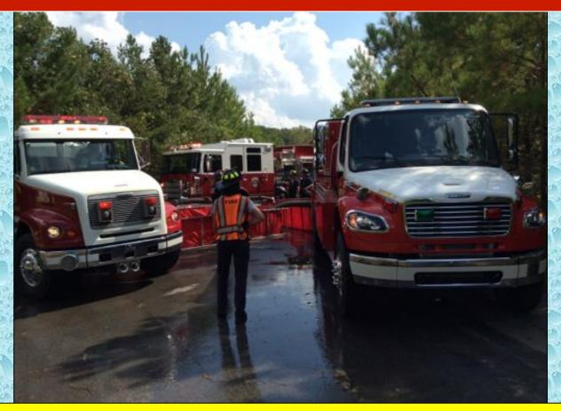
At the 81:00 mark, flow was moved to 800 gpm and the 3-dump tank set-up was operating quite smoothly.
