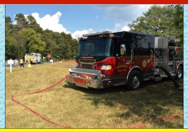
Maiden Engine 3 drafted from a 30,000-gallon underground tank and supplied water to the tanker loading station via 5-inch LDH.
