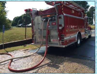
Denver FD's Fireboat 13 (1500 gpm) loaded tankers at greater than 1000 gpm load rate. 3-inch camlock style fittings were as fill connections.
