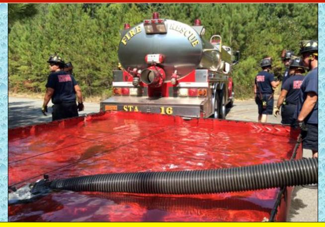
SFTFR Tanker 1 (3000 gal) was the first tanker to arrive. The crews deployed the tanker's 3000-gallon dump tank and transitioned to a dump tank operation began.
