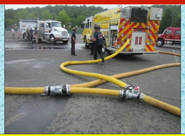
Engine 11's crew simply hooked up an intake line from the jumbo wye and then discharged into the clappered siamese. Once the changeover was made, the wye was closed going to the original side of the siamese.
