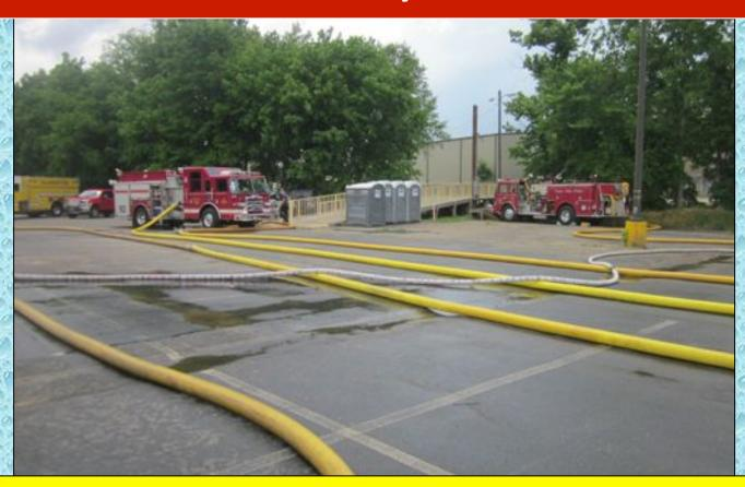
The hose layout was accomplished using Brierfield Engine 203's and Montevallo Engine 93's 5-inch supply hose. In total, 2,200 feet of 5-inch hose was laid out in an accordion fashion in the Civic Center parking lot.
