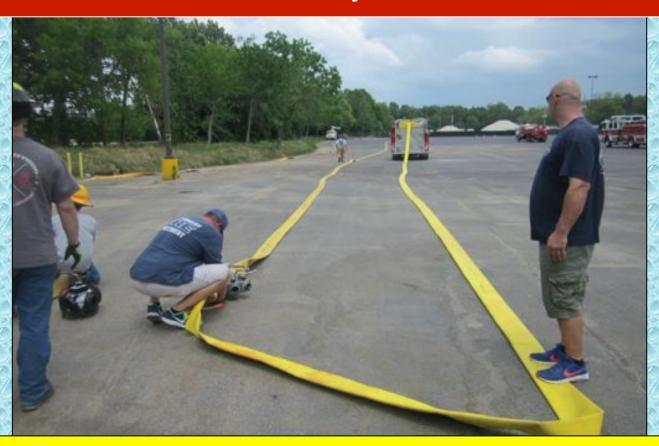
At around the 1,200 ft mark from the supply pumper, an LDH manifold was inserted with the intent of inserting a relay pumper at that location sometime during the drill.
