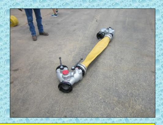
Alabaster Engine 11 (1,500 gpm) was added as a second relay pumper. Their rig was inserted around the 1700 ft mark from the source pumper. A homemade relay valve setup was made using a jumbo wye and a clappered siamese and was inserted before the drill started.
