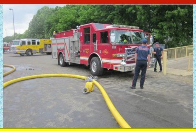
The first relay pumper added to the hose layout was Pelham Engine 92, a 1,250 gpm pumper. The crew added their rig in at the LDH manifold which was located 1,200 feet from the source pumper.
