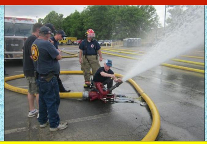
All water flow was measured at a portable monitor equipped with a 2-inch tip. A hand-held pitot gauge was used to capture the flow readings.
