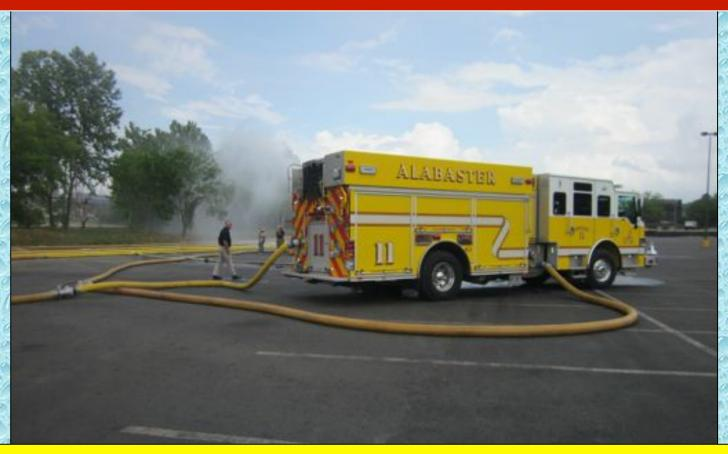
The relay valve arrangement allowed the pumper to be added into the relay pumping without shutting down the water flow to the attack pumper.
