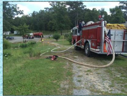
West Shelby Engine 241 (1,000 gpm) drafted from the lake and supplied water to an LDH manifold on 5-inch supply hose. The engine did not have a high-flow discharge, so two smaller lines had to be used to support the 5-inch LDH.
