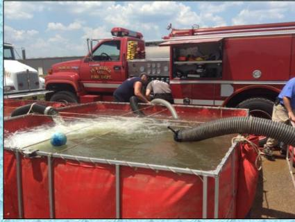
In order to prepare for the 1,000 gpm flow, the Pea Ridge engine needed to take in more water. Two, 2-1/2" suction lines were added to the operation which allowed the engine to achieve the 1,000 gpm flow and still run a jet siphon.
