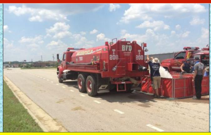
Brierfield Tanker 200 (3,000 gallons) was the first large capacity tanker to arrive at the dump site. Crews grabbed the dump tank off of this tanker while the driver dumped water. Flow was moved to 500 gpm at 13-minute mark, two minutes ahead of schedule.
