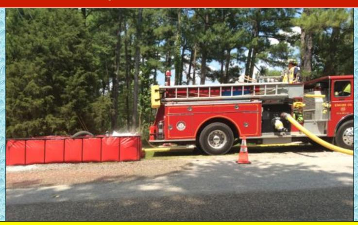
Brierfield Engine 203 (1,500 gpm) drafted water from a dump tank which was filled using water from the fire hydrant. This allowed the tankers to be loaded faster than if they simply connected directly to the fire hydrant.
