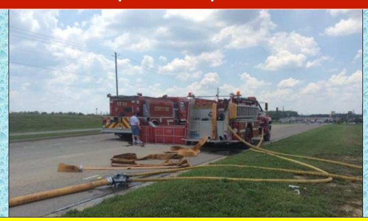
Pea Ridge Engine 101 (1,000 gpm) was used as the dump site engine and its crew went to work setting up as fast as possible for a dump tank operation. Without a high-flow discharge, the engine had to pump several smaller lines into an LDH manifold which supplied the 5-inch hose going to Calera Engine 21.
