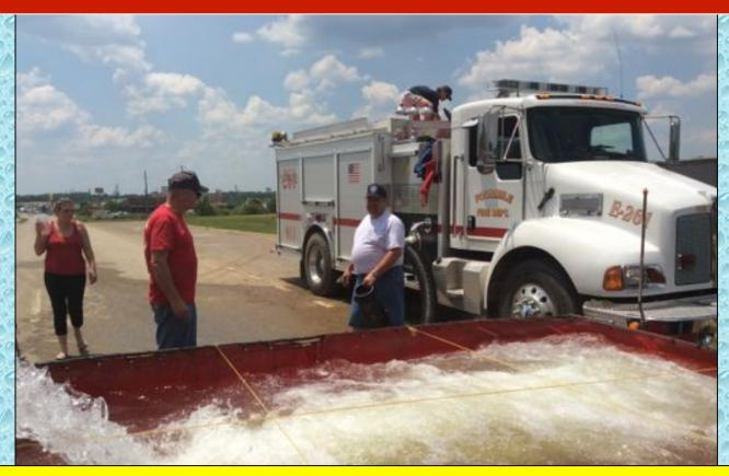
Four Mile Engine 261 (1,250 gpm) was brought in to support the operation by running jet siphons. The engine drafted from one dump tank and then ran several jet siphons, thus allowing Pea Ridge Engine 101 to concentrate on just supplying the attack pumper.
