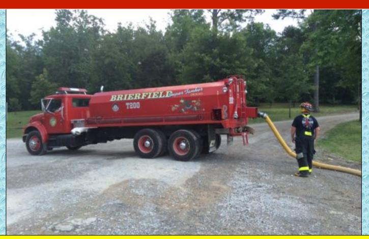
Tankers were loaded using 5-inch LDH when possible – this made for a quick turn-around and was critical to supporting the 1,000 gpm flow.
