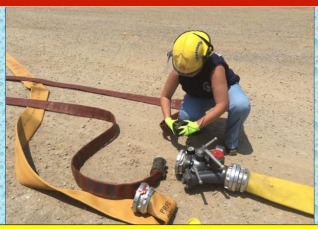
The supply line was equipped with a  $5" \times 2-1/2"$  "water thief" type of appliance. The intent was to use the valve during the initial phase of the drill so that a nurse tanker operation could support the attack engine while a dump site was set up.
