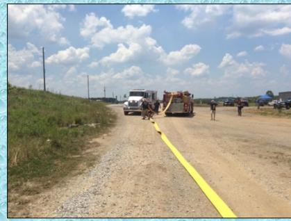
Calera Engine 21 was the first-arriving unit and assumed the role as the attack pumper. The 3-person crew divided up tasks and deployed an attack line and a 5-inch supply line. The stopwatch was started when the engine driver applied the air brakes. The nurse tanker is seen in the photo on the right (white tanker).
