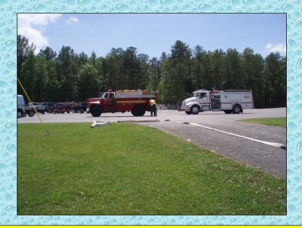
Tankers were filled at the top of the boat ramp which allowed the tankers to get into position without much maneuvering.
