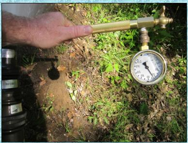
Water flow was a bit delayed in getting started, but at the 8:04-minute mark, water flow was started at 396 gpm. A hand-held pitot device was used to measure the flow.
