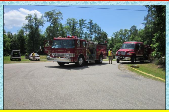
Brierfield E203 and County 17 Tanker 213 were next to arrive on the scene. E203 laid out 100-feet of 5-inch hose from the clappered siamese and Tanker 213 connected to the siamese and pumped its water to the attack engine.
