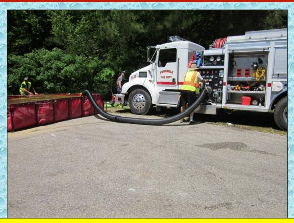
Around the 41:00-minute mark, Four Mile Engine 261 was brought in to run jet siphons so that Engine 203 could focus on increasing the flow to the attack engine. At 51:00 minutes – the flow was increased to 752 gpm.
