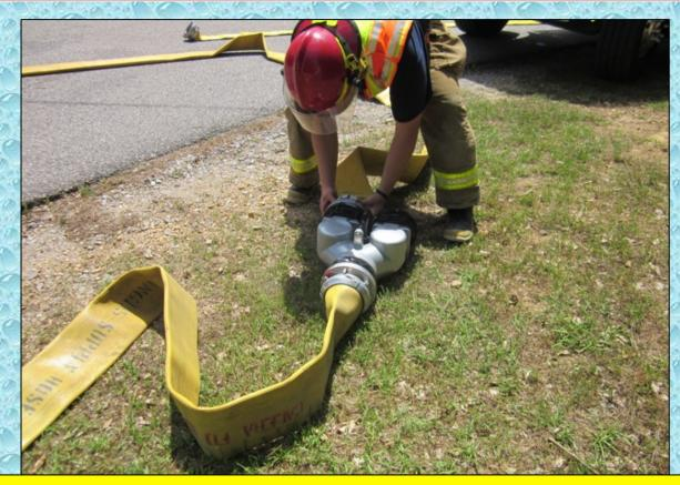
The double-clappered siamese was the critical piece in the initial operation. Its use allowed the dump site engine to get set-up while the engine/tankers pumped off their water to the attack pumper via the siamese.
