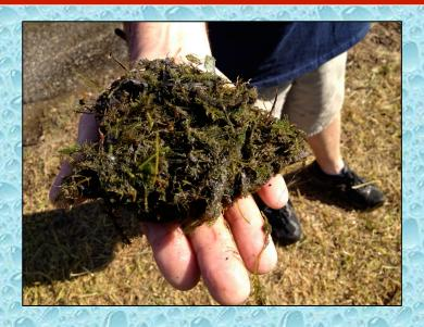
The suction inlet screen on E203's officer's side was clogged with some aquatic vegetation from drafting earlier in the day. This is a good example of the importance of back-flushing a pump after every drafting operation.
