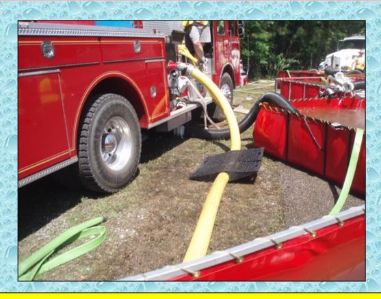
On most FD incidents, there is little concern about vehicle exhaust because the pumpers don't spend much time on the scene. However, during a water supply operation, exhaust is something to consider – especially when hose is nearby.
