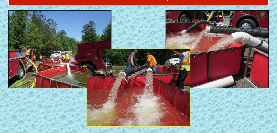
When moving to 1,000 gpm, the need for transferring water is huge. The folks here had to "jump" a dump tank using a ladder in order to get adequate flow into the primary dump tank.
