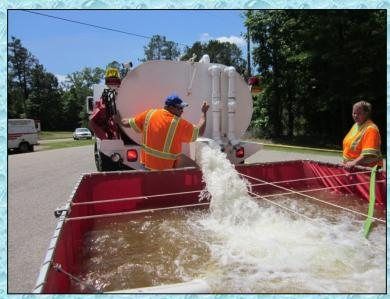
The dump site continues to be built out with three dump tanks now down and in operation at the 14:12-minute mark. However, the dump site pumper is still having difficulty increasing its flow.
