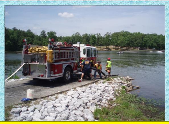
The pumper was positioned in a spot that allowed for easy access to the water. A second suction could have been used off of the driver side suction inlet – however, that was never pursued.
