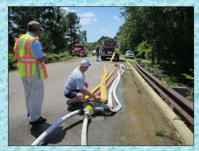
The fill site crew did a great job of making a variety of fill line choices available. The choices minimized the need for adaptors and allowed the loading crew to make and break connections very quickly. The goal is to run a tanker fill site like a NASCAR pit stop – that happened at this fill site!
