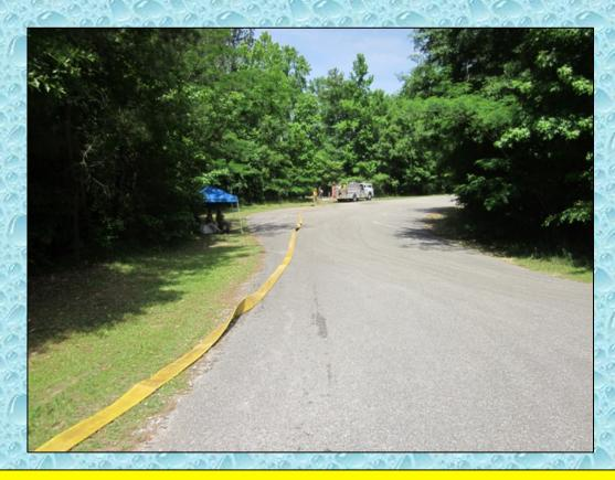
Engine 266 laid out 300-feet of 5-inch hose outfitted with a double-clappered siamese.
