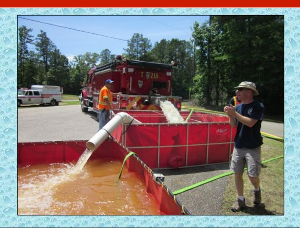
As in any multiple dump tank operation, water transfer operations are critical to the success. A homemade PVC jet siphon is used in this dump tank.
