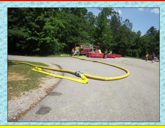
A critical point in the operation – no tankers waiting to dump, no tankers pumping to the siamese, and the dump site pumper can't increase flow. Thus – at the 19:00-minute mark – water flow was interrupted.
