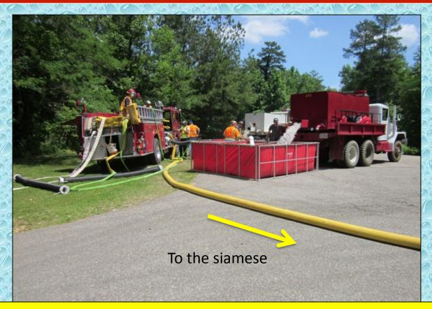
With the dump site now operational, the dump site pumper supplied water to the siamese and the nurse tankers could break free and begin hauling water in a regular, tanker shuttle format.
