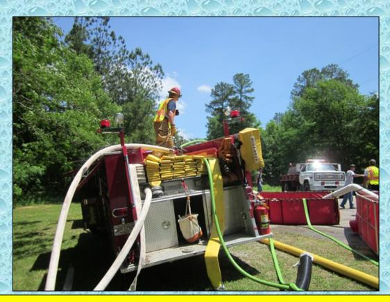
E203 supported the operation of two jet siphons which were controlled by one person atop E203's hose bed. The jet siphons were controlled by a gated wye placed on the end of a 50-ft section of 3-inch hose.
