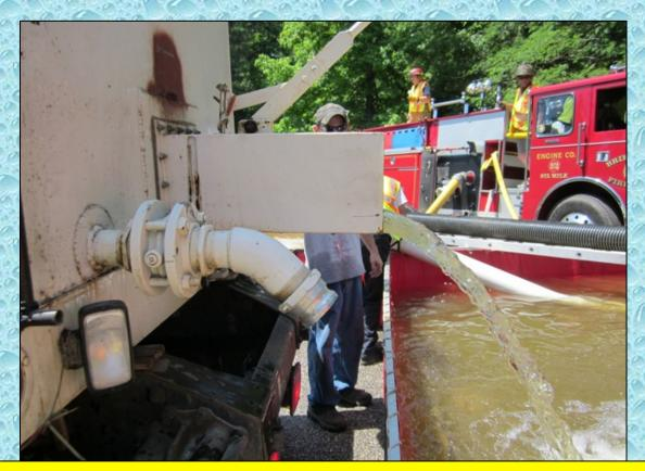
When the water level coming out of a dump chute gets this low, it is time to "cut and run" and get another load. The tanker will be a more efficient water hauler if it does not wait for every last drop to come out.
