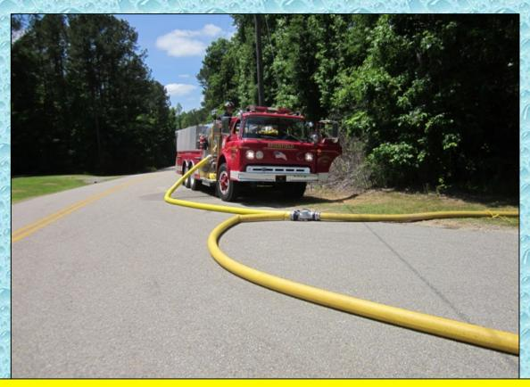
Tanker 206 remains in position as it off-loads the rest of its water before breaking and switching the operation over completely to a tanker shuttle.
