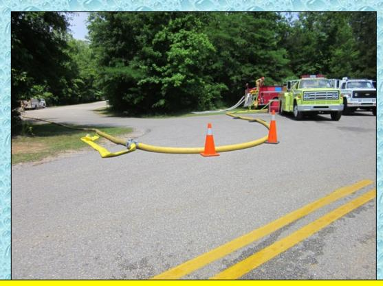
The double-clappered siamese is now being fed entirely by the dump site pumper. However, a short length of 5-inch hose was left attached in case the operation had to resort back to nurse tankers (e.g. mechanical failure of dump site pumper.)
