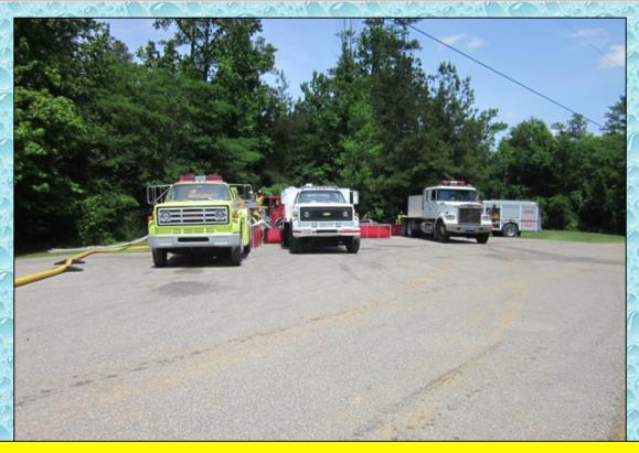
Dump tanks were arranged so that all of the tankers could off-load via their rear dumps. While not necessarily the most ideal arrangement, it worked okay at this drill because there was adequate space and many of the tankers could only dump from the rear.
