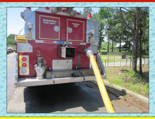
LDH was used to fill Brierfield's Tanker 206 – the fill time was impressive and reinforced the efficiency of using LDH in fill site operations.
