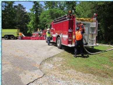
A plan was implemented that allowed the pumpers to pull past the dump tanks, and pump back to the site via 3-inch hose and discharge elbows attached to the primary dump tank. This process worked out well and kept the pumpers out of the way of the tankers, while still using the water carried on the pumpers.
