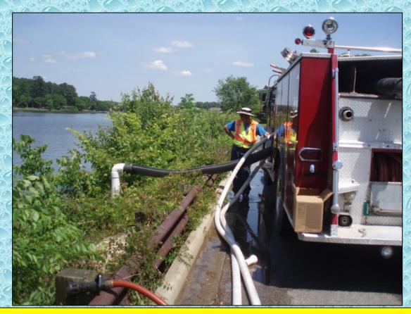
The crew used a dry fire hydrant as the suction point and then fed an LDH manifold using two, 2-1/2-inch lines because the pumper had no high-flow discharge.
