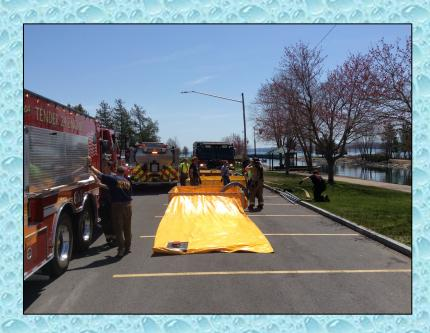
One of the dump tanks used was a 3000-gallon Single-Lane Max tank from Fol-Da-Tank. This was one of just two times where we have seen the Single-Lane Max tank used. It worked quite well.
