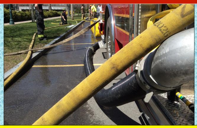
The dump site crew chose to use a single-lane tank arrangement. Traffic cones were used to restrict lane access to the tanks thus simulating a real life road condition in the large parking lot. A 90-degree suction elbow was used to better access the dump tanks.
