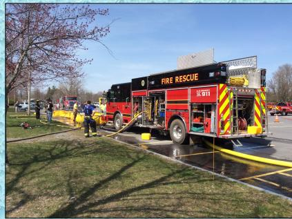
By the end of the drill, flow peaked at 1700 gpm using a Hose Monster flow diffuser and a TFT Blitzfire device. The single, 2000 gpm pumper was able to support the entire dump site operation.
