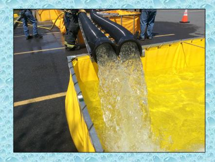
With three dump tanks in use and flow expected to exceed 1500 gpm, one person was assigned the job of controlling the water transfer devices.
