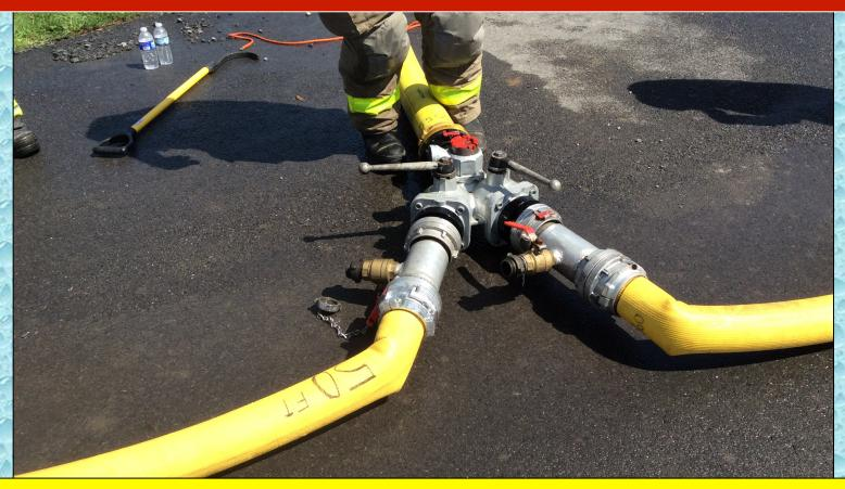
"Special" drain devices provided by Plainville were used to speed up the draining process of the fill lines in between loading operations.
