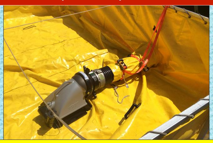
The folks chose to use a "through-the-drain sleeve" set-up for drafting. A TFT low-level strainer was used as the suction strainer.
