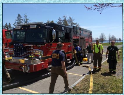
The drill was run as a simulated deployment of the Tri-County Water Supply Task Force. Crews rallied at the Sennett fire station and then convoyed several miles away to a simulated fire event location. The goal was to have a large-scale (1000 gpm+) operation up and running within 10-15 minutes of arrival. Weedsport Rescue Pumper 1 (2000 gpm) operated as the dump site pumper.
