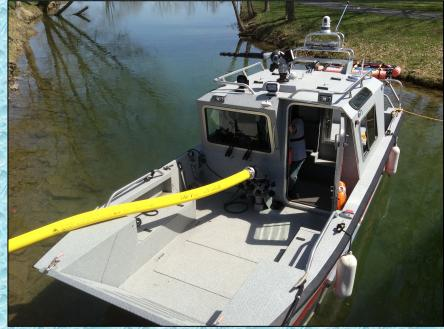
Owasco Marine 1 (1250 gpm) took water from a canal location and supplied an LDH line out to an LDH manifold were tankers were then loaded.
