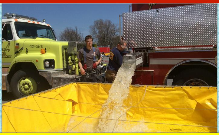
The initial grouping of resources included water hauling rigs plus two engines to assist with dump site and fill site operations. Owasco's fire boat was also deployed as a fill site resource.
