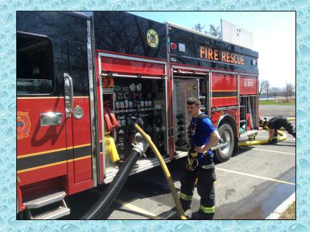
The 2000 gpm pumper had plenty of capacity to support a 1000 gpm+ flow and operate water transfer devices at the same time.
