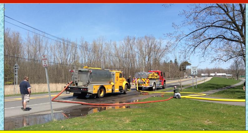
Three personnel were used to load the tankers; two folks made and broke connections and one person served as the "loader" and operated the LDH manifold control valves. While two tankers might have been connected at one time, only one at a time was loaded.
