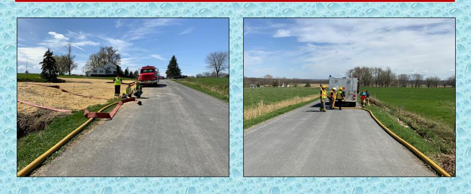
Canoga Engine 302 (1250 gpm) drafts from the pond using a dry fire hydrant and loads tankers using 4-inch LDH.
