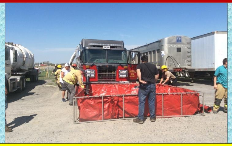
The 1<sup>st</sup> dump tank was deployed at around 90-second mark due to the quick arrival of the 1<sup>st</sup> tanker.
