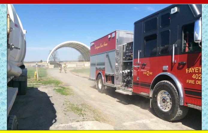
Fayette 402 arrives on the scene and lays out several hundred feet of 5-inch LDH supply line simulating a reverse lay from the fire out to a dump site area.
