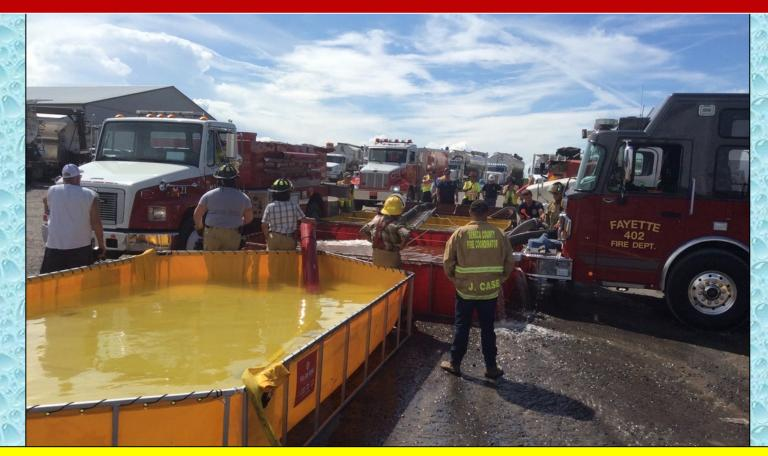
By the 46-minute mark, four dump tanks were in use and flow was moved to 1000-gpm.
