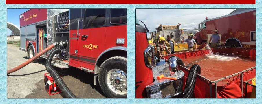
Around the 20-minute mark a second, 6-inch suction line was added to Fayette 402 and water flow was increased to 750 gpm..
