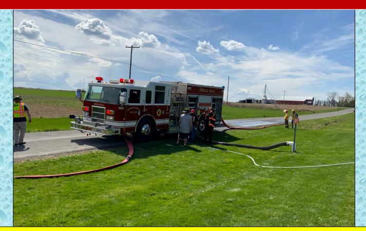
Seneca Falls Engine 1403 (1500 gpm) drafts from the pond using a dry fire hydrant and loads tankers using 4-inch LDH.
