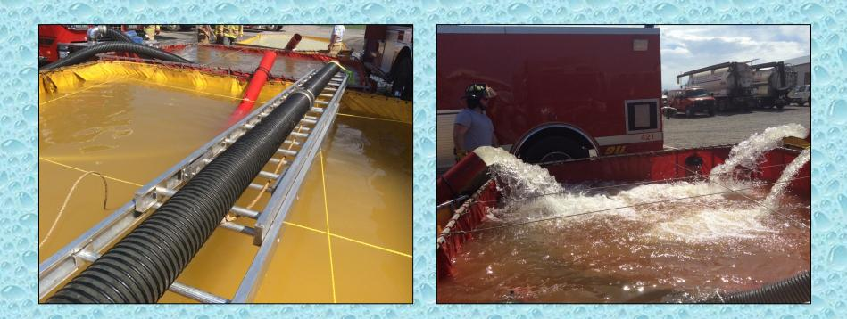
As flow increased, the need to transfer water between the dump tanks also increased. Transfer devices included Holley Pipes and traditional suction hose jet siphons.
