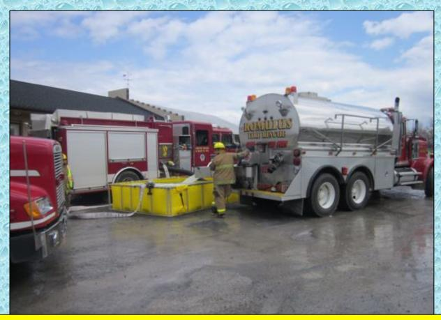
At the 33-minute mark the flow was moved to 750 gpm and two fill sites were in full operation.
