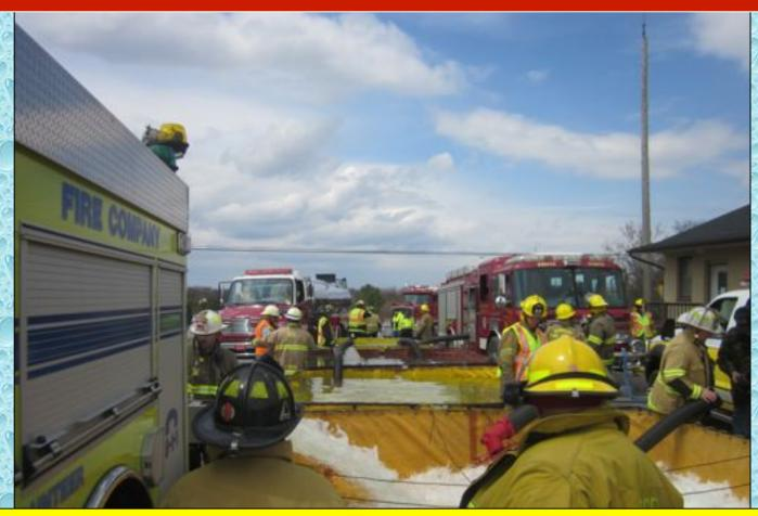
At the 15-minute mark, three dump tanks were down and in operation and the flow was moved to 500 gpm at the attack engine.
