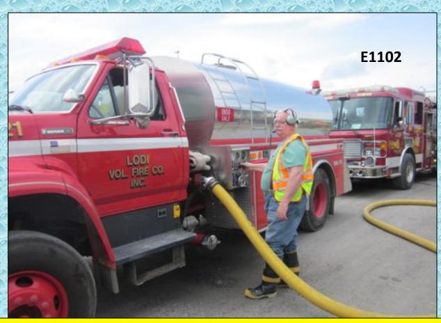
While the Lodi tanker operator was busy supporting the attack pumper, Ovid FD Engine 1102 (1,750 gpm) arrived and began setting up for a dump tank operation.
