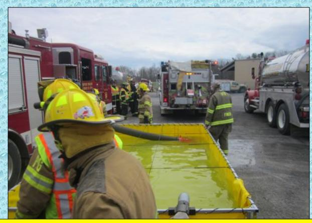
More tankers began to arrive and operations were underway in preparation for moving the flow to 500 gpm at the 15-minute mark.
