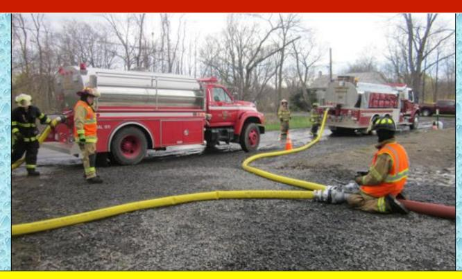
Tankers were loaded using 4-inch LDH supplied through a jumbo-wye which was fed by a 5-inch line from Engine 402. The "loader" (valve guy) never left the jumbo wye. The "pit crew" made and broke fill connections and the loader simply opened the jumbo wye. Most IMPORTANTLY — only one tanker was filled at a time. Two could be connected — but only one loaded.
