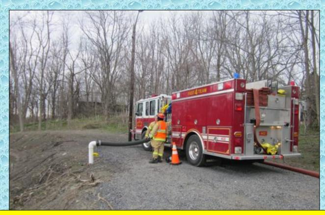
Fayette Engine 402 (1,500 gpm) responded as part of the 1<sup>st</sup> Alarm assignment and went directly to the Church Street pond to set up for loading operations. The first tanker was loaded and back at the dump site 24-minutes after the initial dispatch.
