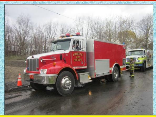
Traffic cones were used to mark where the loading crew wanted the incoming tankers to stop – very similar to "pit row" during a NASCAR race.
