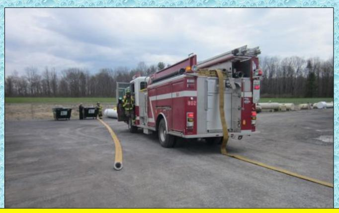
Engine 802 laid 200 feet of 4-inch supply hose and got into position to pump a 5-inch line that was pre-connected to a Hose Monster flow diffuser equipped with a fixed pitot for accurate flow measurement.
