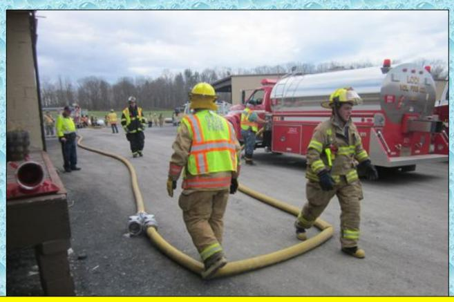
The use of the double-clappered siamese is often called the "rural hitch" and it can be a very useful operation when arriving on the scene with limited staffing and an urgent need for water.
