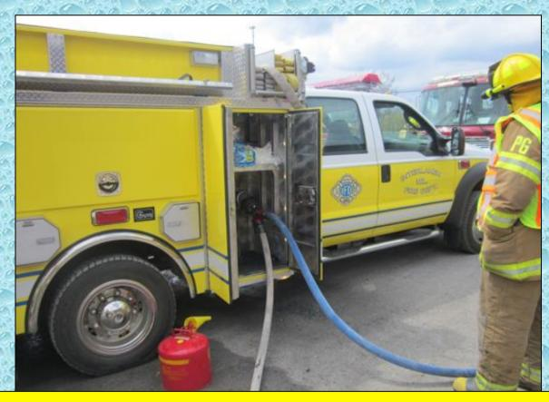
With the flow increase also came the need to improve water transfer operations. Interaken's mini-attack unit (500 gpm) was brought in to run some of the jet siphons.
