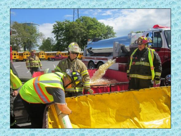
Border City Tanker 221 is shown here off-loading its 3,000 gallons of water as folks begin to set up water transfer devices.
