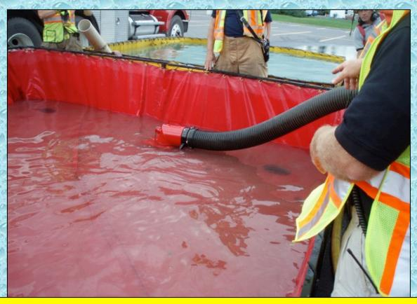
At one point, it got dangerously close to running out of water in the primary drafting tank, but the crews resolved the jet siphon problems and water flow was not interrupted.
