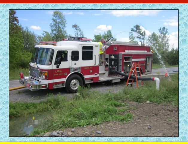
The crew used LDH as the tanker fill line. The step ladder was used to aid in connecting to the dry fire hydrant.
