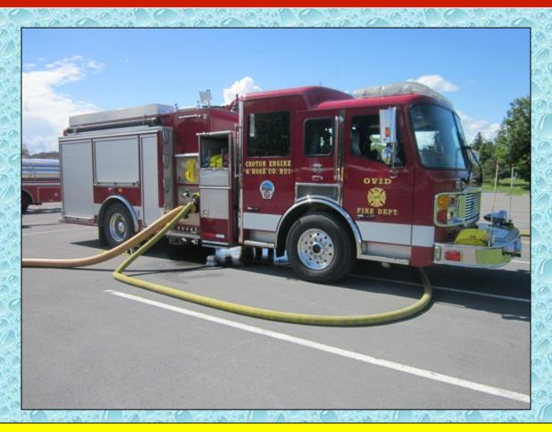
The dump site pumper is now supplying the attack pumper and dump tank operations are underway.
