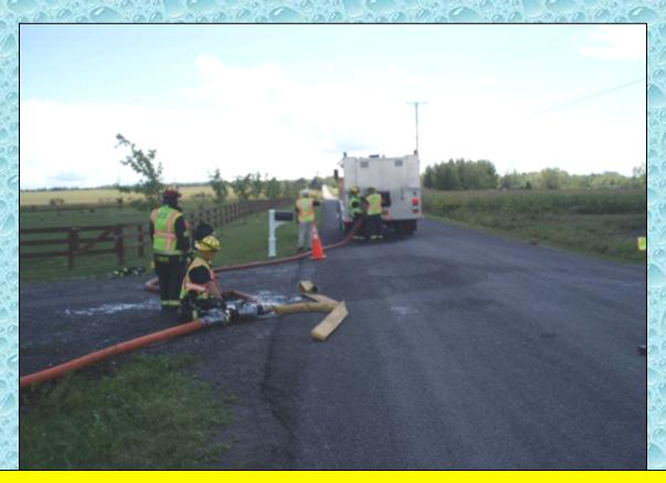
Crews work to fill Fayette's Tanker 421. The use of the LDH manifold simplified the filling operation by placing control of the flow at the loading station instead of at the pump panel several hundred feet away.
