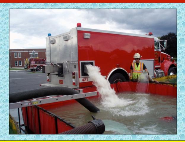
Fayette's tanker offloads its 2400 gallons of water into the primary drafting tank.
