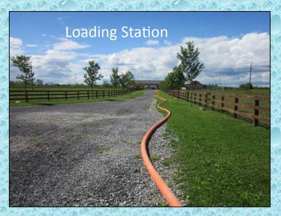
This fill site was the second site to open and required coordination between the pumper and the fill crew. The folks working here did a nice job of filling tankers. The use of 5-inch LDH would have improved the pumper's capability, however, the site was still pretty efficient in its operation.
