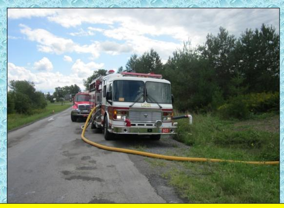
Lodi Engine 802 (1500 gpm) established a tanker loading station at a pond on Smithtown Building Road. The pond was equipped with a 6-inch dry fire hydrant and provided plenty of water for filling tankers.
