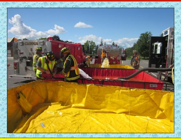
At the 9:42-minute mark, a third dump tank was deployed but not placed into operation. It still needed a water transfer device.
