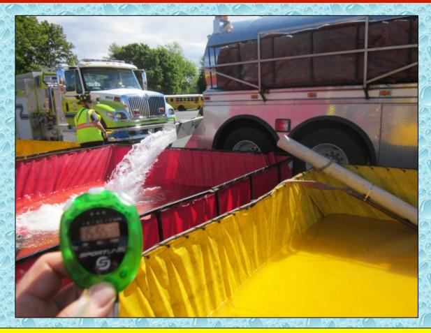
At around 16-minutes, tankers from the second Tanker Task Force arrived just in time because the flow had been increased to 504 gpm at the 15-minute mark.
