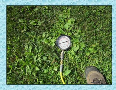
At the 5:00 minute mark, water flow was started at 334 gpm. A Hose Monster flow diffuser device with a built-in pitot was used to accurately measure the flow.
