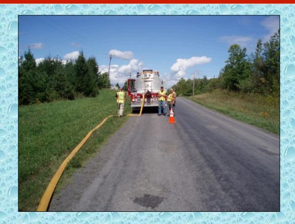
The use of LDH to load tankers can really cut down on the fill time when compared with using 2-1/2-inch hose — even if the tanker does not have an LDH direct fill intake.
