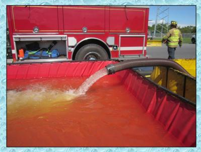
With the goal to move to a 4-dump tank operation, crews work to assemble addition water transfer devices. The plan is to jump the third tank using two sections of hard suction hose and a jet siphon.
