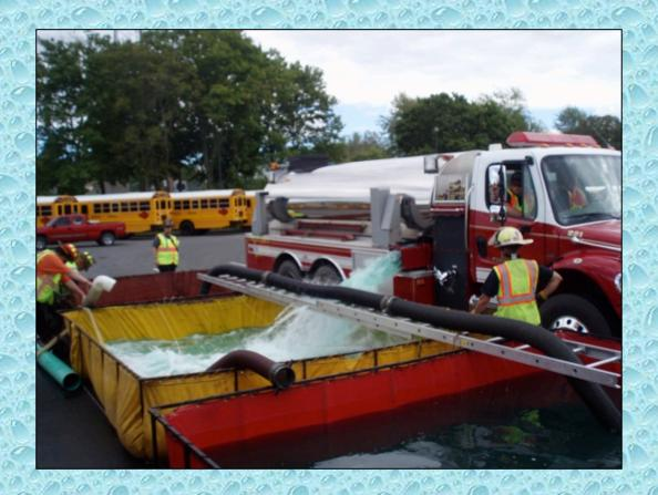
Border City's tanker offloads another load of 3,000 gallons. There were a couple of issues with the water transfer process – but they were worked out.
