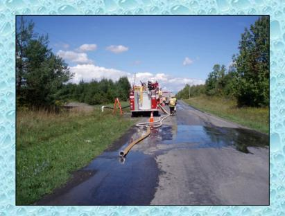
Since E802 only had one, high-flow discharge, the second tanker fill line was created by manifolding two, 3-inch lines together using a 3-way valve.
