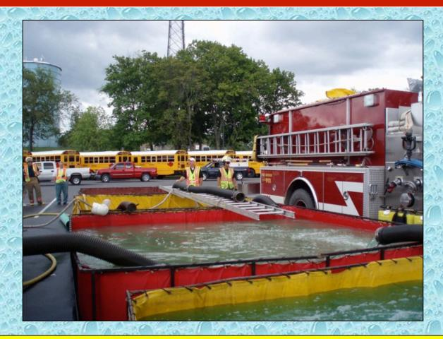
At the 90:00-minute mark, the flow was moved to 1024 gpm where it remained through the end of the drill.
