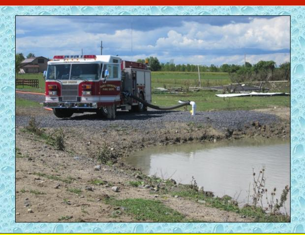
Oaks Corners Engine 3211 (1500 gpm) was used as the supply pumper at this fill site. The farm pond was outfitted with a 6-inch dry fire hydrant.
