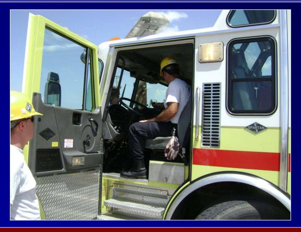
During the 16 hours of practical skill work, students learned the basics of attack, relay, and supply pumper operations. Here, a student learns about the do's and don'ts of engaging the fire pump.
