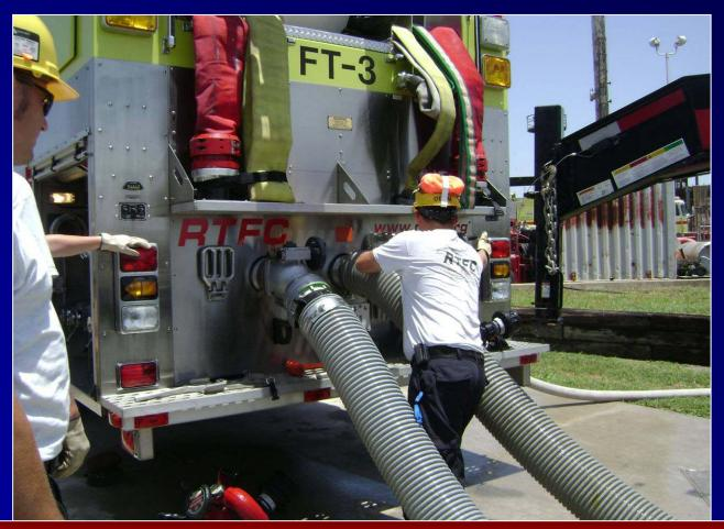
Students learned how to draft through one suction and then use the water movement through the pump to prime the other length of suction hose.
