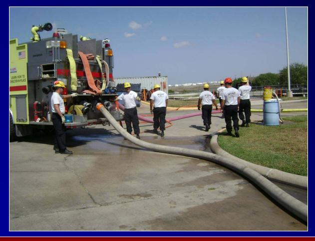
Foam 5, a 3,000 gpm foam pumper was used as the attack pumper - giving the students plenty of pumping capability for the day's events.
