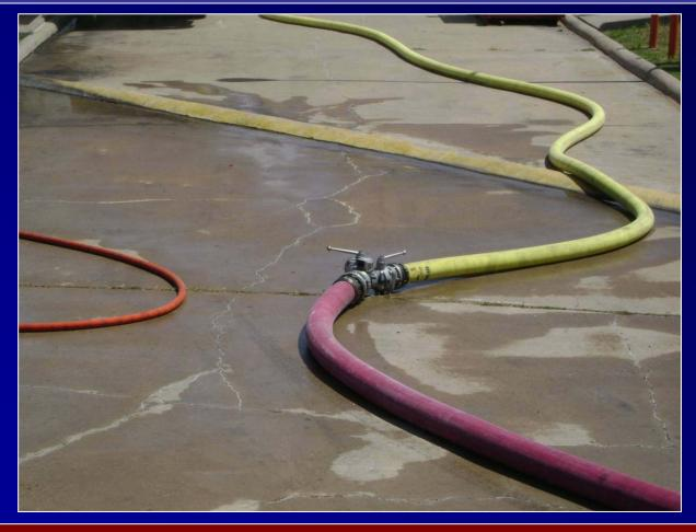
The crews used 6-inch hose to supply a jumbo-wye and then a 5-inch line to a TFT 1,250 gpm CrossFire portable monitor.
