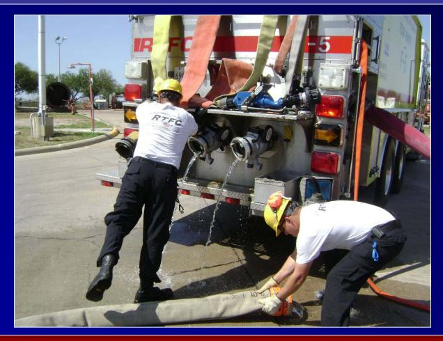
Foam 5 is set-up to take three, 6-inch supply lines into the rear-mounted pump. When all three lines are in use, the pump can discharge over 4,000 gpm.
