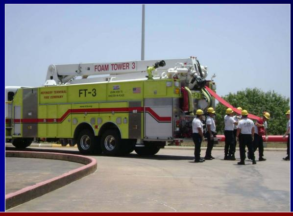
Foam Tower 3, a 3,000 gpm rated pump, was used for the relay pumping operation on the second day of skills. Students are shown above stretching a 7-1/4-inch supply line which was fed by Foam 5 using a 150 psi fire water system.
