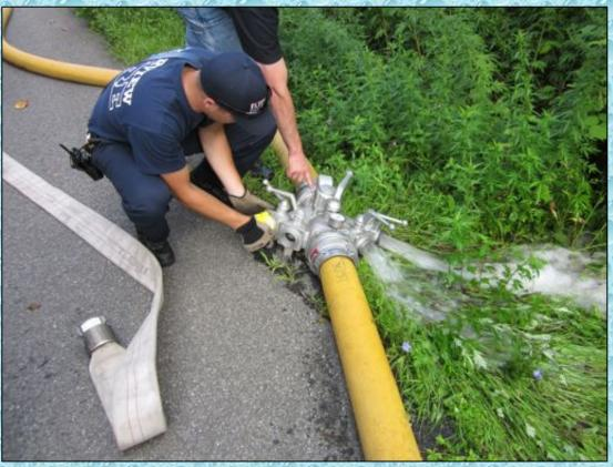
Fairview Engine 41-12 was added as a third relay pumper. The pumper was inserted 1,500-feet past Roosevelt E63-14 at the LDH manifold that had been left by the LaGrange pumper.
