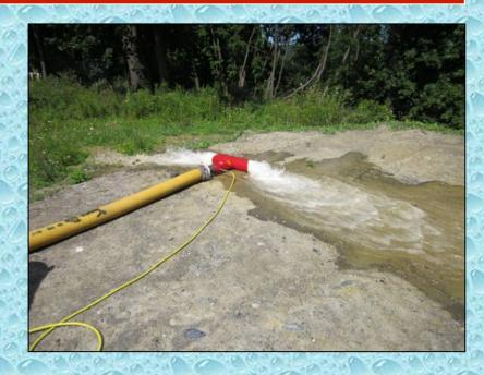
Engine 47-14 receives water through the 2,100 feet of 5-inch LDH that it laid out. The plan had been to lay all 3,000 feet, but space did not permit that amount of hose to be laid. Thus, the total lay was 5,100 feet of 5-inch LDH. A Hose Monster device was used to accurately measure the flow.
