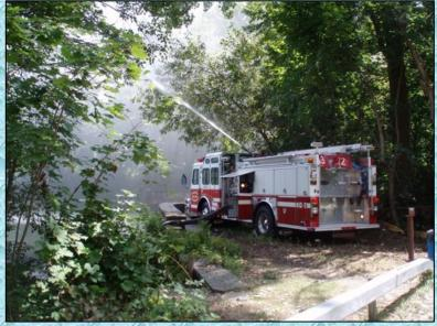
The drill started with Roosevelt Engine 63-12 (1,500 gpm) establishing a water supply at the dam. The crew used several lengths of 6-inch suction hose and a floating strainer to reach the "best" suction point for drafting.
