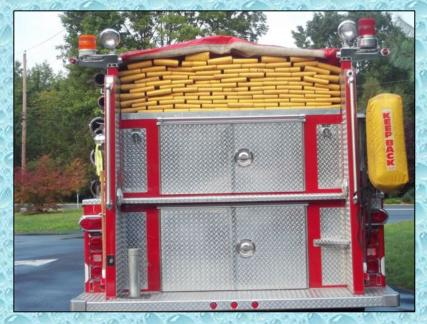
Engine 63-14 operated as the lone relay pumper in the first evolution. The 1,000 gpm pumper carries 3,000 feet of 5-inch LDH - plus all of the appliances and adaptors to make a long lay of LDH work.
