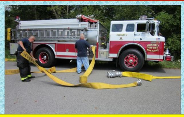
After laying out all of its 5-inch LDH, Engine 63-14 begins to set up as the relay pumper. The plan was to pump to LaGrange Engine 47-14 through its 3,000 feet of 5-inch LDH. However, because of space limitations, Engine 47-14 only laid out 2,100 feet of LDH.
