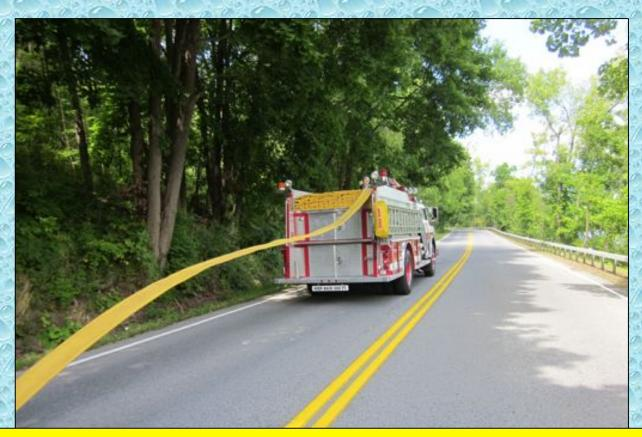
Engine 63-14 lays out its 5-inch LDH. Although this photo looks like the pumper is driving about 60 mph, the hose was laid at a much more moderate speed. The roadway was closed to regular traffic during the drill period.
