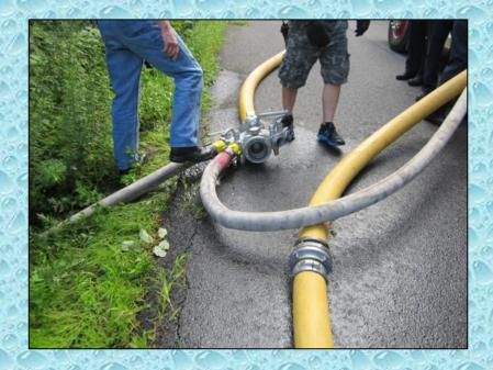
While the LDH manifold does not provide an uninterrupted flow option when adding a relay pumper. It does allow more flexibility than just separating a hose coupling and "hopping" in-line.
