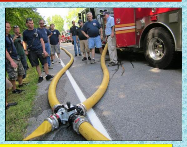
Tower Ladder 46-45 (1,500 gpm) was added at the TFT Oasis valve located in the middle of the initial 3,000 ft hose lay.
