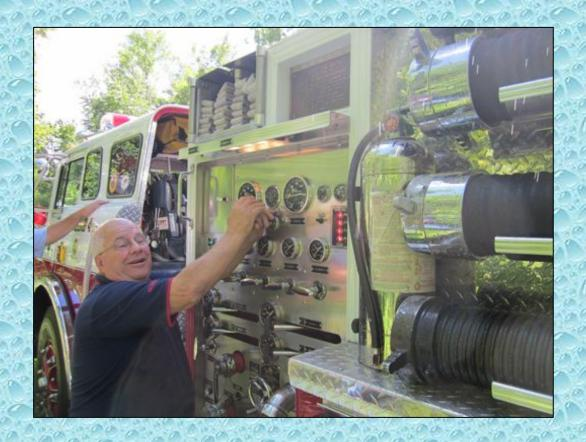
With water now at the relay pumper, the operator makes the needed adjustments in order to send the water to the attack pumper.
