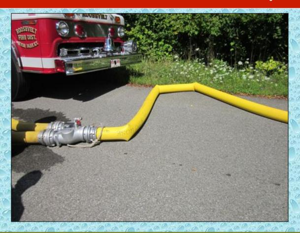
The two lines feeding the siamese are charged and water is on its way to the attack. The kinks removed themselves once the hose was completely charged.
