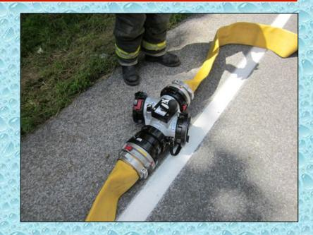
Knowing that a couple of flow tests would be completed during the relay pumping drill, a TFT Oasis valve was inserted at the 1,500-feet mark of the initial hose lay. The Oasis valve is TFT's version of a hydrant valve that can also be used as an in-line relay valve. All that is needed is one adaptor. A Humat valve can also be used as can the old Jaffrey Z-valve. An in-line relay valve allows a pumper to be added in the middle of a hose lay without shutting down water flow.
