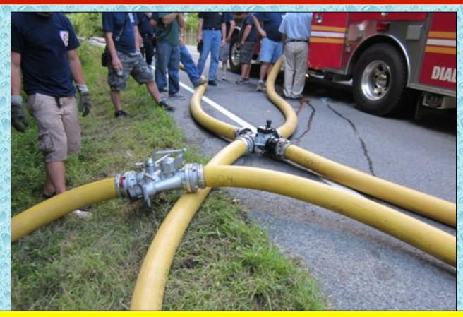
The TFT Oasis valve allowed TL 46-45 to insert itself as a relay pumper without having to stop the water supply to the next pumper. The manifold was added by the operator in order to provide additional supply lines if needed.
