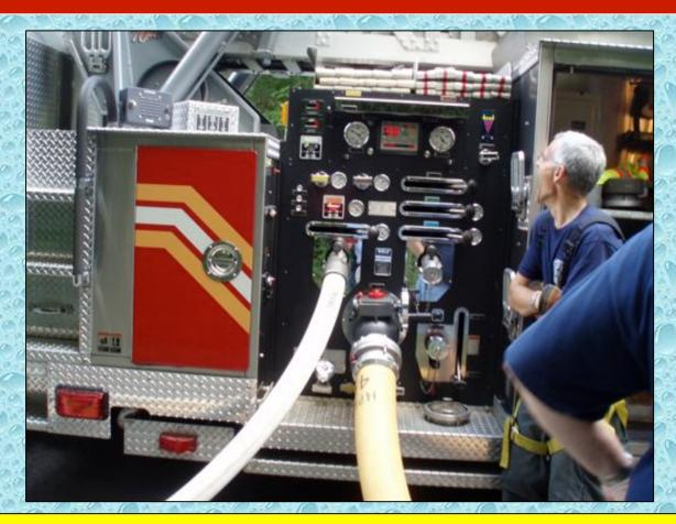
The tower was limited in its LDH discharges, so a smaller hose line was used to supplement the flow.
