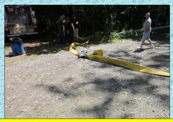
With a water supply secured, Roosevelt Engine 63-14 began laying out its 3,000 feet of LDH. A LDH manifold was used at the source pumper in case additional lines were needed to supply the operation.
