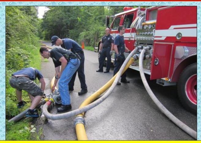
Engine 41-12 pumped two, 3-inch lines to support the relay operation since they did not have a full-flow high-flow discharge. The set-up worked just fine.
