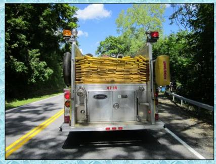
Engine 47-14 served as the attack pumper in the relay drill. The 1,750 gpm pumper also carries 3,000 feet of 5-inch LDH and a multitude of LDH appliances.
