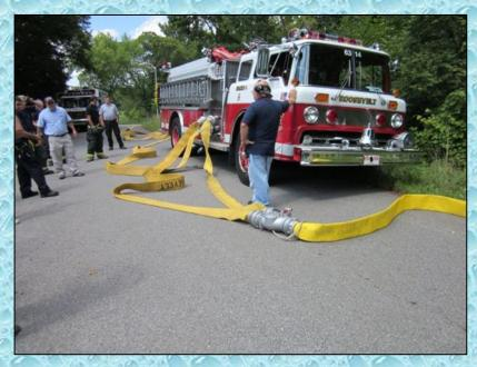
Because Engine 63-14 does not have a "high-flow" discharge, a double-clappered siamese was used to support the expected flows.
