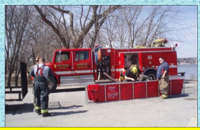
The eductor was fed from this 1,250 gpm pumper. The eductor then supplied water into the dump tank – from which the pumper then drafted and filled tenders with a target fill rate of 1,000 gpm./
