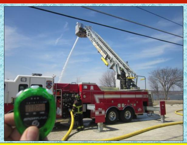
Flow was moved to 585 gpm using LeClaire's elevated master stream which was equipped with a flowmeter.
