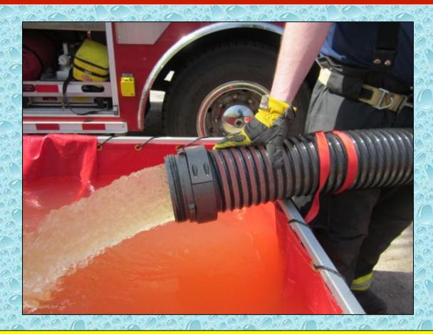
Great looking flow from this jet siphon water transfer system. This is what a jet siphon discharge stream should look like!
