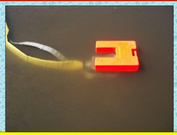
The Fol-Da-Tank floating eductor was on loan to Port Byron for the drill. The eductor uses the simple venturi principle to supply water.
