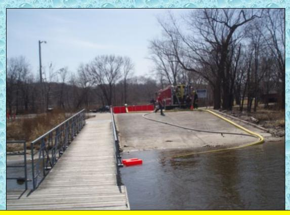
Port Byron PB4 (1,250 gpm) took position at the top of the boat launch and deployed the floating eductor which was fed by2-1/2" hose and supplied water back to a dump tank using 5-inch hose.
