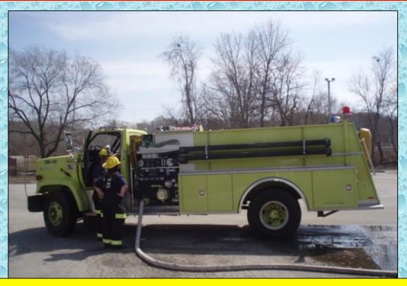
Tenders were then filled using 2-1/2" hose. The fill operation was unable to support a 1,000 gpm fill rate – partly because of the water needed to make the eductor work and partly because of the smaller hose lines used to load the tenders.
