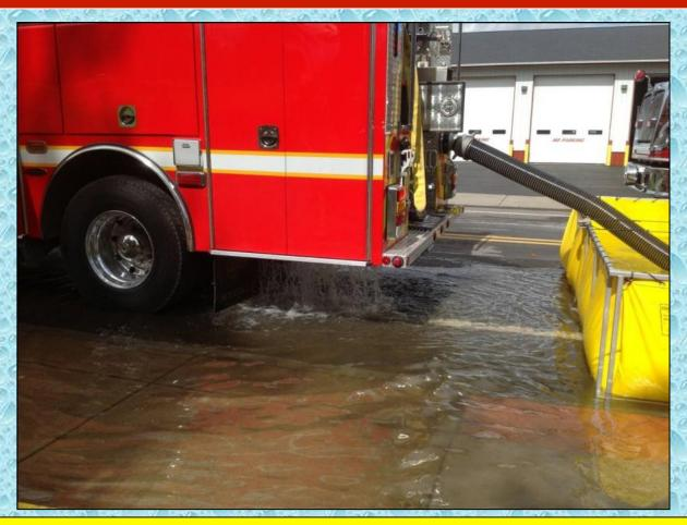
The dump site crew decided to set up the tanks fore and aft of the pumper to allow room for tankers to pass by on the street.
