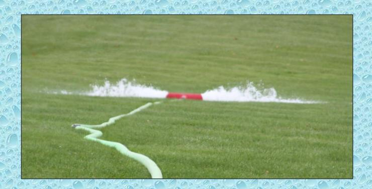
The crew stretched 25-feet of 4-inch hose to a Hose Monster flow diffuser equipped with a built-in pitot tube for measuring flow. The diffuser simulated the use of a portable master stream device.
