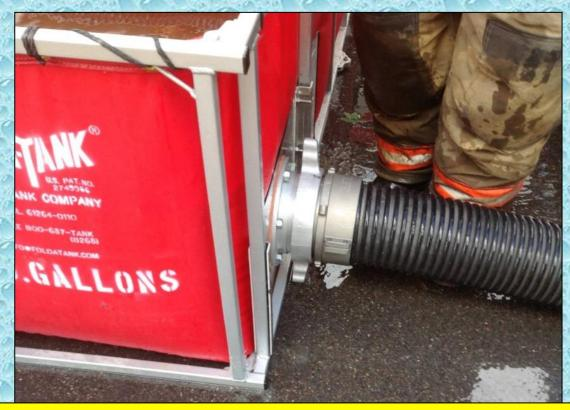
A forth dump tank was obtained and crews quickly put it in service. Unfortunately a leaking hard sleeve coupling had the dump site engine desperate to achieve a prime. This was alleviated by taking suction off the front intake and rechecking the coupling – it was missing a gasket.
