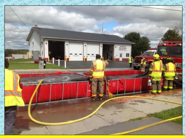
At the 15-minute mark, three dump tanks were down and the dump site was fully operational. The dump site engine switched from tank water to drafting – and dump site operations were underway.
