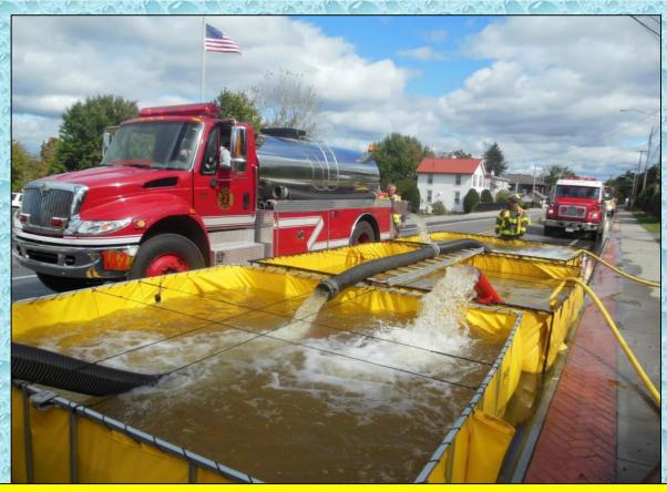
The flow from this Holley Tube jet siphon is a good, solid stream of water – which is exactly what is needed. Note the 6" hard sleeve on the ladder – moving the water once is the most efficient way to manage multiple tanks.
