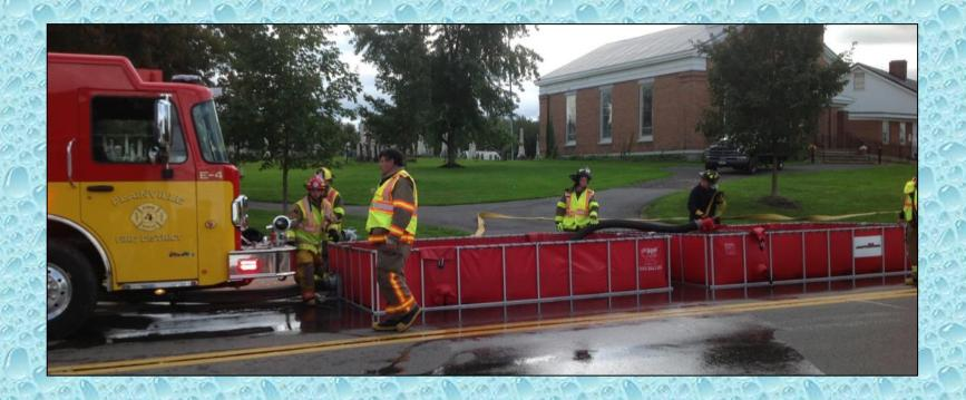
As the fire flow increased, it was noted that the jet siphon supplying the front primary dump tank could not keep up. A second jet siphon was added and that corrected the problem.
