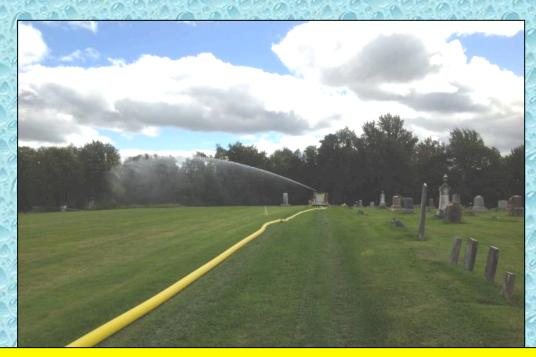
Plainville Engine 2 was the first-arriving unit at the church and assumed the role of the attack pumper. The stopwatch was started when the engine driver applied the air brakes. This unit was followed by Cato Engine 1 which laid out 600 feet of 5 inch hose from the dump site. Engine 1 used 100 feet of 5 inch hose to supply Engine 2.
