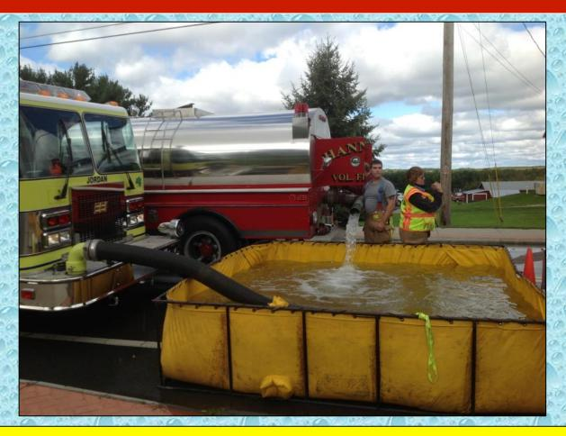
Lots of tankers need lots of direction. A coordinator was appointed to control where (which dump tank) tankers off-loaded their water.
