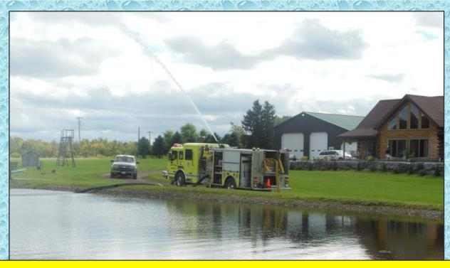
The crew arrived to find a very soft shoulder from an overnight rain and had to figure out a more stable position from which to draft. This position required more hard sleeves than the engine carried so additional hard sleeves had to be obtained from tankers coming in to be filled. The crew eventually established an LDH fill line out to the main road and were able to fill successfully.
