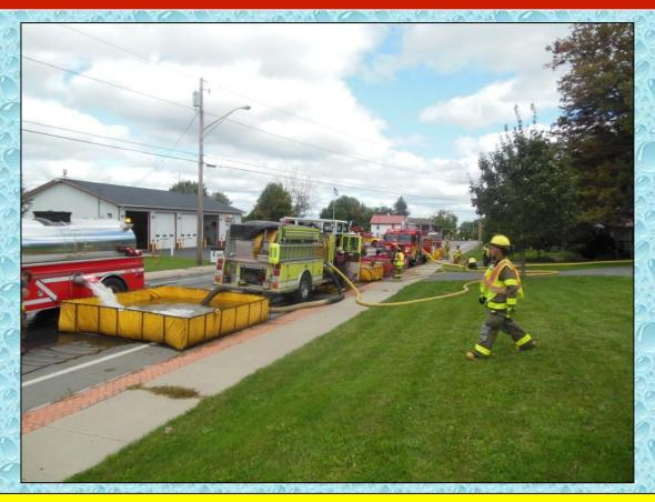
Crews did a nice job of spacing the tanks so that two tankers could dump at once - which is critical when trying to achieve flows in excess of 1,000 gpm.
