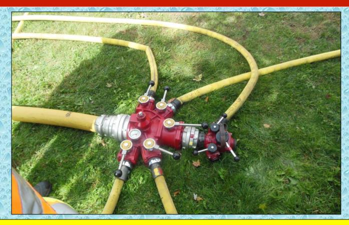
A seventh dump tank was deployed to supply Jordan Engine 2 (to run jet siphons) and the original sixth dump tank was repurposed to support the main water supply. Jet siphons were supplied and controlled using an LDH manifold.
