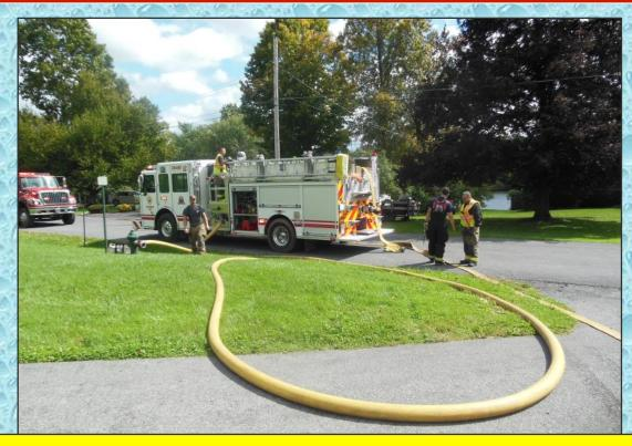
This fill site was established at a fire hydrant. The crew did a good job of trimming out all of the outlets of the hydrant in order to maximize flow. Although the pumper was missing appliances, the crew overcame the problem by controlling flow at the pump panel.
