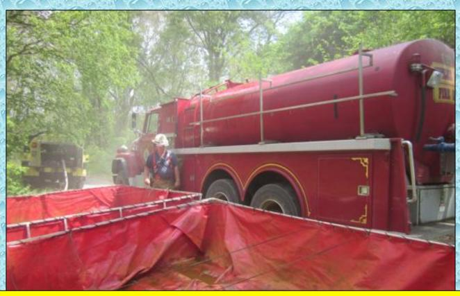
Tanker 1 arrived back just in time. Its 3500 gallons of water were much needed. Brush Tanker 3 is seen in the background pumping off its water into the primary dump tank via 3-inch hose. BT3 has no dump valve on it.
