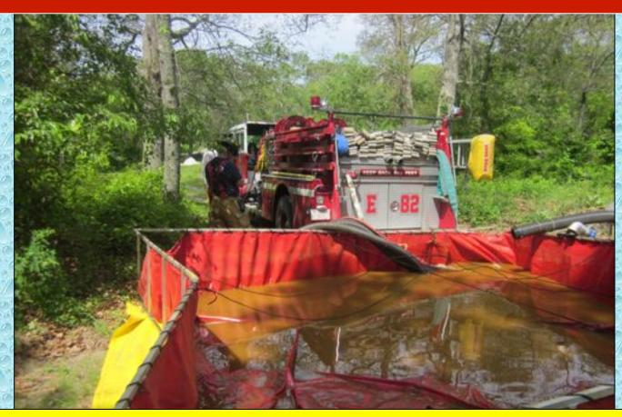
Tankers were delayed getting filled at the lone fill site, so water supply levels ran dangerously low at the dump site. Water flow was interrupted for about 2-minutes around the 30-minute mark in the drill.
