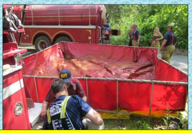
With nurse tanker operations underway using a 3-inch supply line from Tanker 1 to Engine 82, the crews began setting up for dump tank operations using Tanker 1's 4,000 gallon dump tank.
