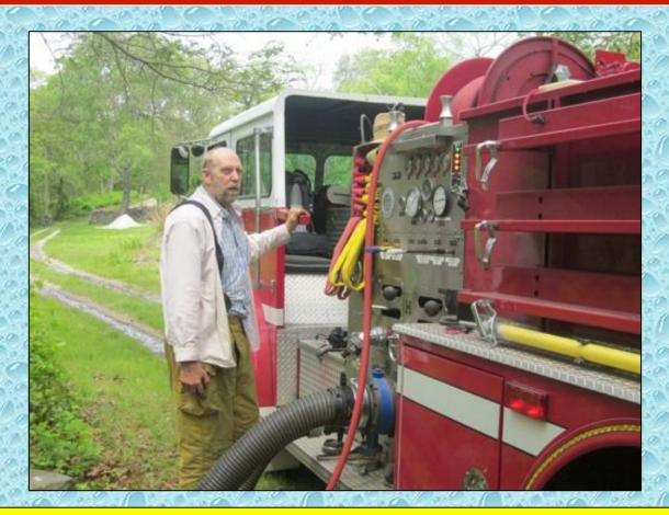
Engine 82's pump operator had to balance time between keeping the attack line working, drafting, and running the jet siphon in the dump tank.
