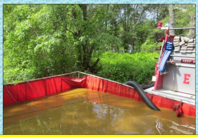
Engine 82 started flowing 250 gpm at the 5-minute mark and at the 13-minute mark, the operation was ready to switch to a dump tank operation.
