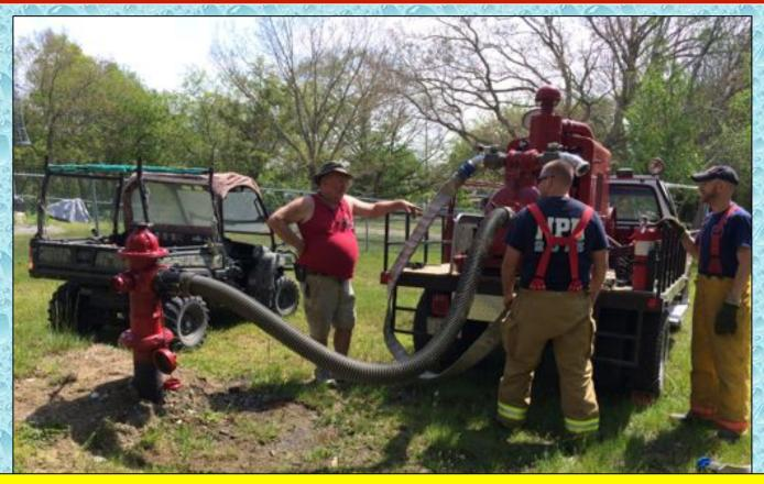
A traditional "looking" fire hydrant is connected to the 15,000-gallon above ground tank. Water comes out of the hydrant under head pressure from the tank, therefore the pump must be hooked up using suction hose.
