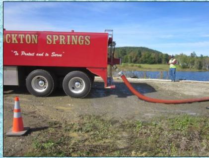
Stockton Springs Tanker 8 (3,800 gal) is shown here being loaded – also through LDH.
