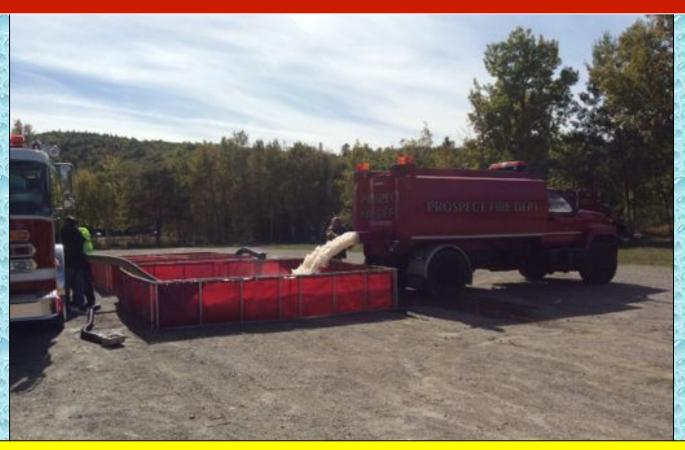
Prospect Tanker 2 was the next tanker to dump its water. Most of the tankers participating in the drill could only dump from the rear, so the arrangement of the dump tanks became important.
