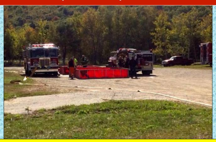
As additional units arrived on the scene, folks helped set up dump tanks. In the meantime, Engine 1 was prepared to supply tank water to Engine 3 through the 300 ft of 4-inch supply line.
