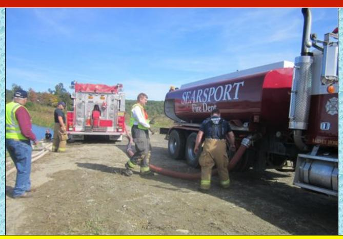
Searsport Tanker 1 (3,500 gal) is shown being loaded in this photo. LDH was used to reduce loading time and to achieve the 1,000 gpm minimum load rate.
