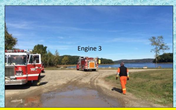
Searsport Engine 3 was the first-arriving unit and assumed the role as the attack pumper. The 4-person crew divided up tasks and deployed two attack lines. Prospect Engine 1 arrived next and reverse laid a 4-inch supply line to the dump site area. The stopwatch was started when the Searsport engine driver applied the air brakes.
