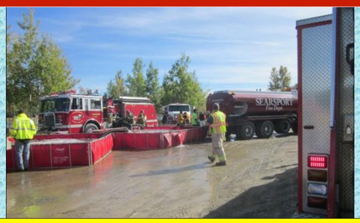
As the dump site was expanded to a 3-tank operation, the outer tanks were placed in a diamond shape to better accommodate the rear-dumping tankers. Plus, all tankers entered the dump site from the same direction.
