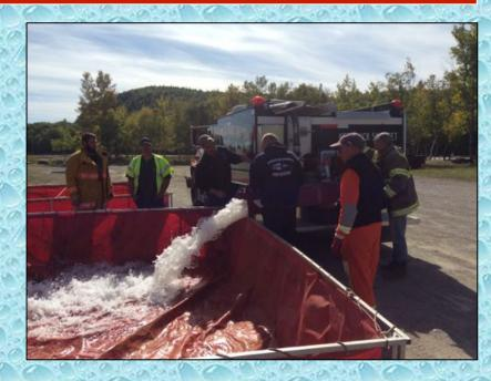
With Engine 1 now ready to draft (note suction inlet control valve), Prospect Engine 3 dumps its water into the dump tank..
