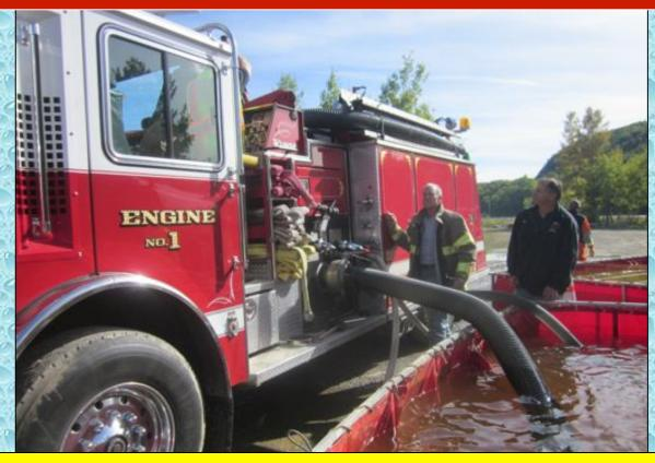
Prospect Engine 1 operated as the dump site pumper. The crew used a length of 2-1/2-inch suction hose to bolster the intake capability of the pumper. The single-4" supply line proved restrictive at 750 gpm, the addition of the 2-1/2" supply line to the attack pumper allowed the flow to move to 1,100 gpm.
