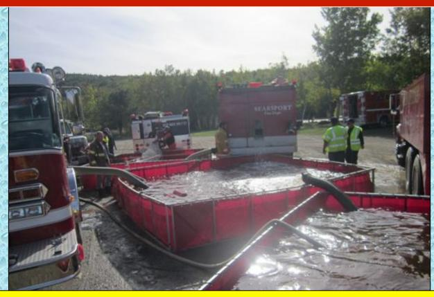
In the end, the dump tank arrangement allowed three tankers to dump simultaneously and the use of the Stockton tanker/pumper to run jet siphons allowed the Prospect pumper to commit entirely to supporting the attack pumper.
