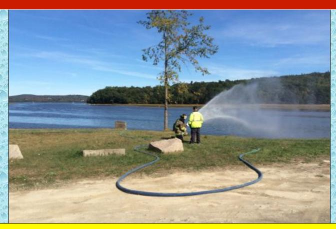
Two, 1-3/4-inch attack lines were used to flow water at the 5-minute mark. The combined flow was 250 to 300 gpm. Tank water from the two engines was used to initiate this flow.
