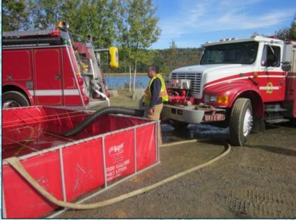
Because the dump site pumper was having trouble supplying the attack pumper and running the jet siphons (pump capacity and pressure), Stockton Springs TP2 (500 gpm) was pulled from hauling water and put into operation running jet siphons. This reduction in tankers hauling water actually increased the flow delivery to 1,100 gpm – sometimes, that is what is needed for success.
