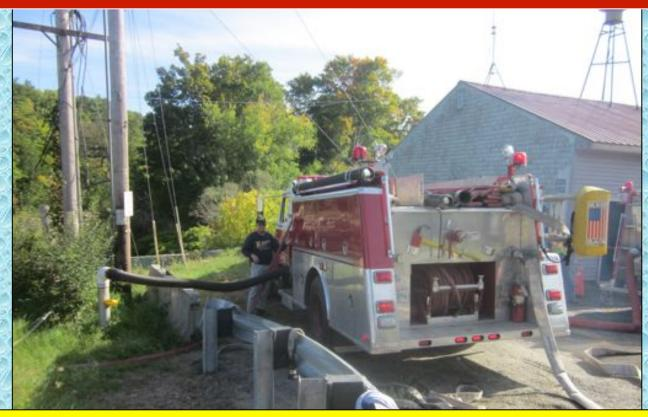
Searsport Engine 1 (1,000 gpm) was used as the pumper at this fill site. The crew really hustled and was able to get the fill site up quickly. Drafting through the dry fire hydrant proved problematic and the crew was only able to support about a 650 gpm fill rate.
