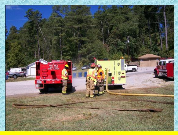
The fill-site crew also did a great job of managing fill site operations. Here they are shown filling the Holly Springs tanker while one of Remlap's tankers is in line to be filled next.
