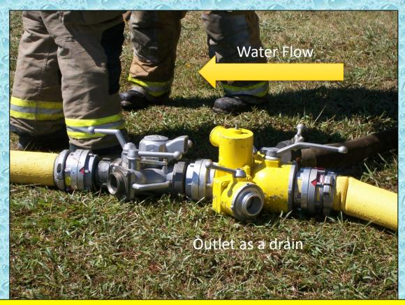
Not pretty – but functional. Two manifolds were connected together at the tanker loading station. This allowed the tankers to be filled using 4-inch hose while still having a 2-1/2" outlet for a drain.
