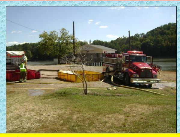
One of the difficulties encountered was that the dump site pumper was at the "end of the line" of tanks – which meant water had to be transferred more often than if the pumper had drafted out of a center tank.
