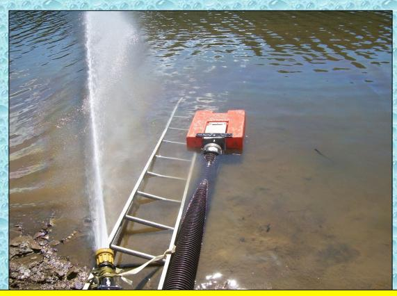
A floating strainer was used due to shallow water near the ramp. The ladder was used to help keep the strainer in place. Note the use of a circulation line – again, good drafting practices.
