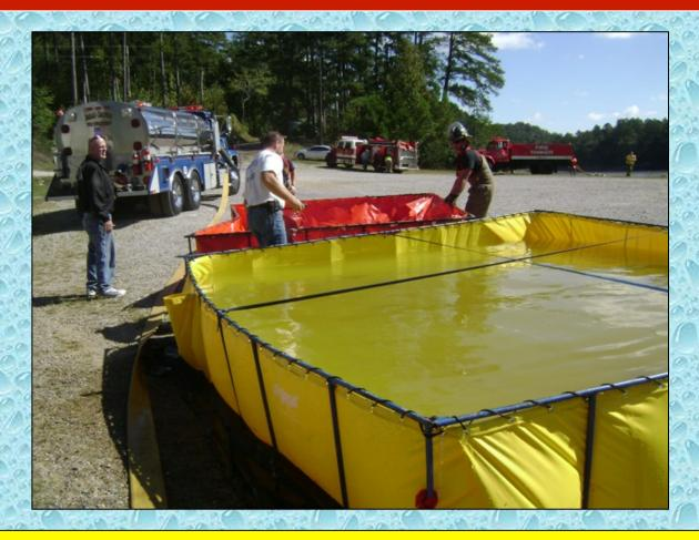
A 4<sup>th</sup> dump tank (1,500-gallons) was set up shortly after the water flow was resumed.
