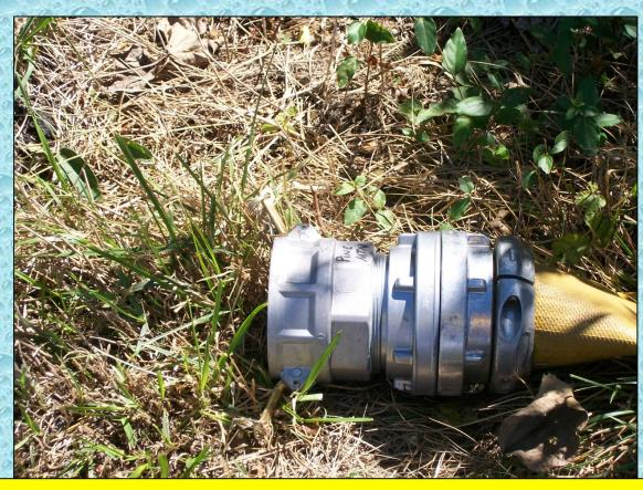
A 4-inch Storz to CamLock fitting was used at the hydrant fill site on the fill line.
