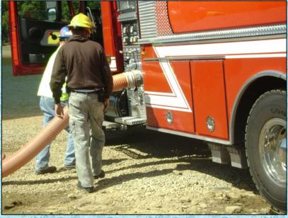
With the vacuum pump engaged and already drawing a vacuum on the tank, the crew connected the 6-inch suction hose to the suction inlet.
