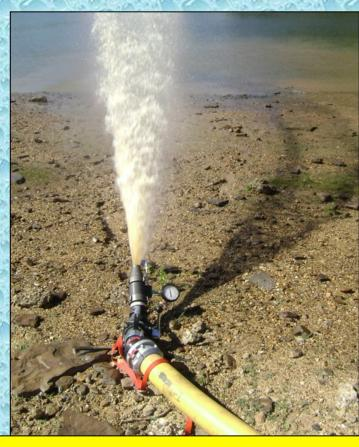
At the 5:00-minute mark, water flow was started at 250 gpm. A flow test device with a fixed pitot tube was used on the Blitzfire to ensure accurate flow measurement.
