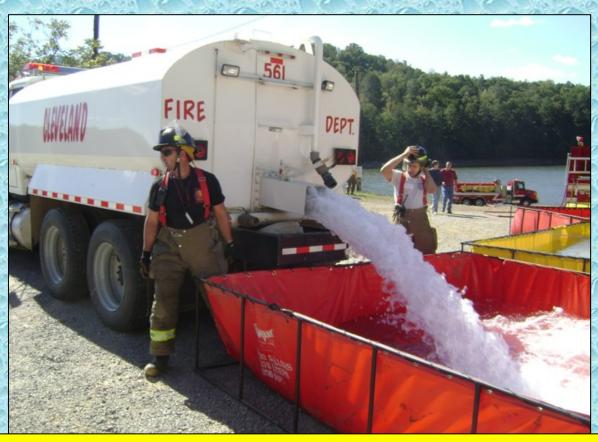
Cleveland's Tanker 561 dumped its 2,500 gallons into the 4<sup>th</sup> tank as the crews prepared to increase the flow.
