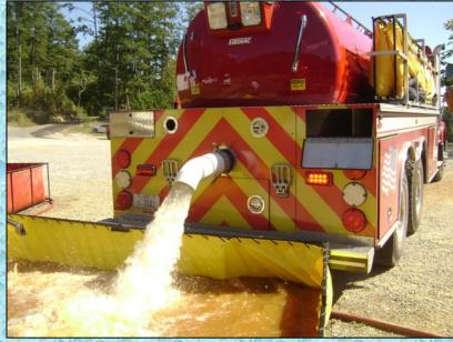
The vacuum tanker uses a large rotary gear pump to develop vacuum for loading and pressure for offloading. The tanker is shown above "blowing off" its water at around 1,800 gpm.
