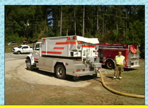
Pine Mountain Tanker 1462 (1800 gallons) was one of the first tankers to get filled at the lake fill site. It was filled in just over 2:00 minutes – or about an 800 gpm fill rate.
