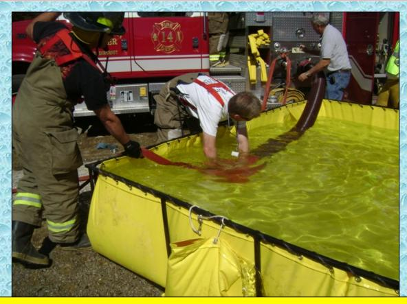
With flow now interrupted, troubleshooting operations commenced. The first option was to try and self-prime using the jet siphon connection on the low level strainer. Unfortunately, that did not work. The pump would not pump.
