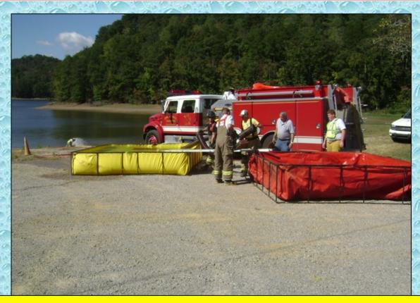
The dump site crews began setting up water transfer operations as the second phase of the ISO test got under way. The crews had ten minutes to expand the flow rate.
