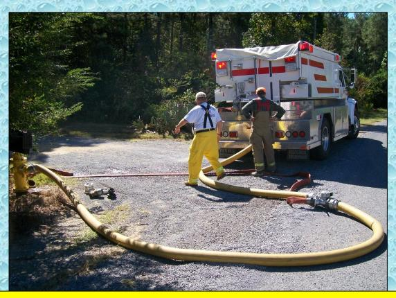
The hydrant fill site was only used once. Pine Mountain's tanker crew is shown here using 4-inch hose to fill directly off of the hydrant.
