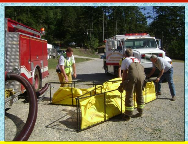
The two crews made great progress in getting the first dump tank set up. The first tank down was a 2,100-gallon tank from the Pine Mountain tanker.
