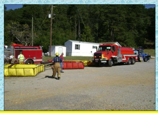
Meanwhile, a third dump tank is set up as the dump site expands. The 3,000-gallon Firovac vacuum also arrived as did the 3,300-gallon tanker from Dallas-Selfville.
