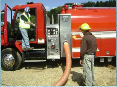
The valve was then opened and water began to enter the tank. The specially designed high-flow strainer allowed the tanker to be loaded at a rate over 1,000 gpm.
