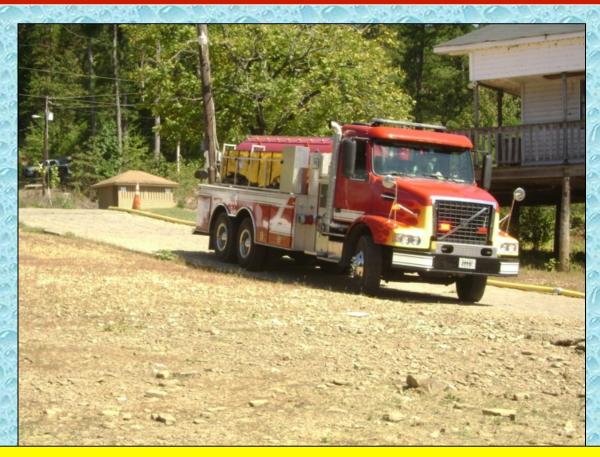
The Firovac vacuum tanker operated independently of all fill sites. The two-person crew was able to fill the 3,000-gallon tanker by simply getting next to the water's edge and engaging the vacuum pump.
