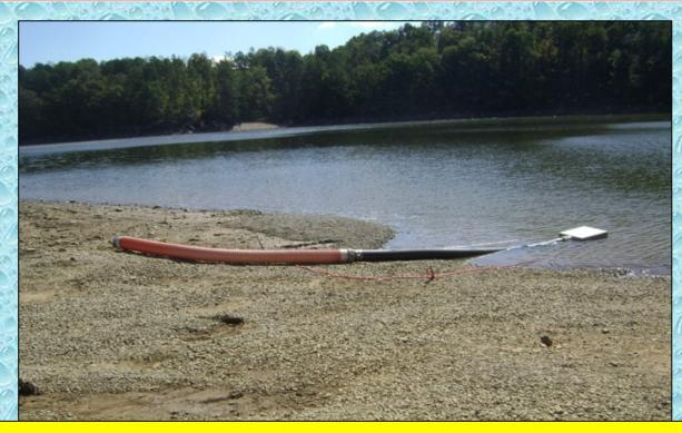
Once the vacuum tanker crew set up their suction hose and strainer the first time, they could just leave it in place and take off hauling water. Upon their return to the fill site, all the crew had to do was connect the suction hose back up to the rig. This is perhaps the greatest feature of the vacuum tanker – no need for a fill site engine or crew!
