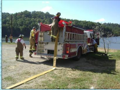
With everyone ready, the drill started. Pine Mountain Engine 1451 arrives on the scene and the clock starts. The 4-person crew works to advance a 4" line to a TFT Blitzfire while also beginning to set up for dump tank operations.
