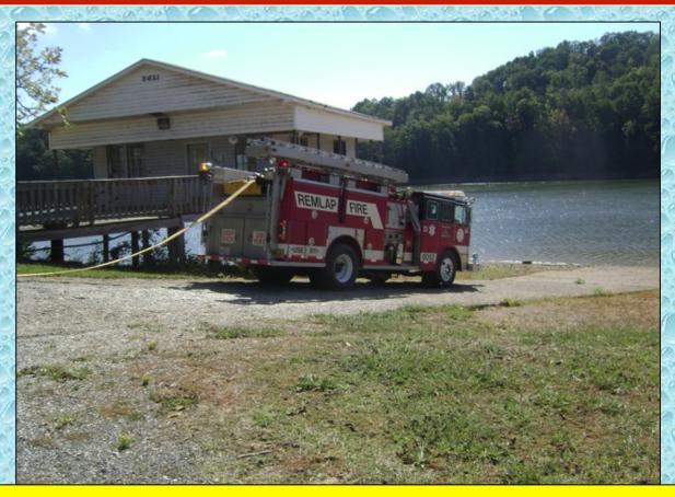
Remlap Engine 8052 (1,250 gpm) arrives at the boat ramp to set up a tanker fill site. They laid out 300-feet of 4-inch hose and dropped an LDH manifold for fill site operations.
