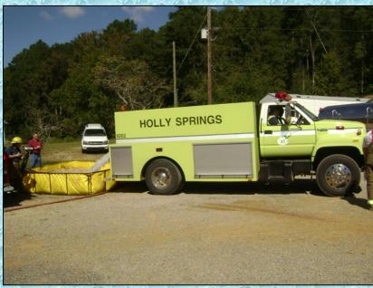
With dump site operations stabilizing, additional tankers began to arrive. Holly Springs Tanker 9262 is shown above dumping its water.
