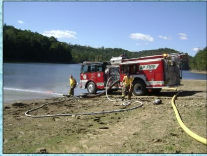
The engine crew did a great job of getting their rig set-up for drafting. By getting their pumper close to the water source, they minimized the lift and maximized pump capacity.
