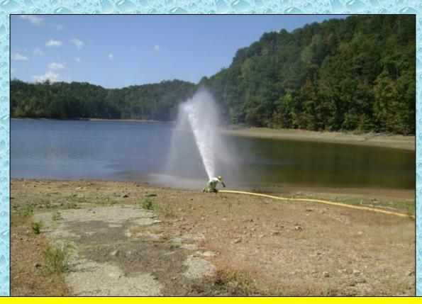
At the 45-minute mark, the flow was moved to 500 gpm where it was basically sustained for the remainder of the drill.
