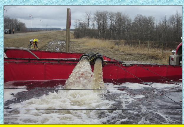
Dual jet siphons were used to transfer water from the 2,100-gallon tank into the 4,000-gallon tank. Engine 8's 1,750 gpm pump had plenty of capacity to support the 750 gpm flow and run the two jet siphons.
