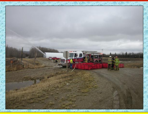
At the 13:16 minute mark, water flow was started at 250 gpm – a bit late because of some radio communications issues with the units in staging.
