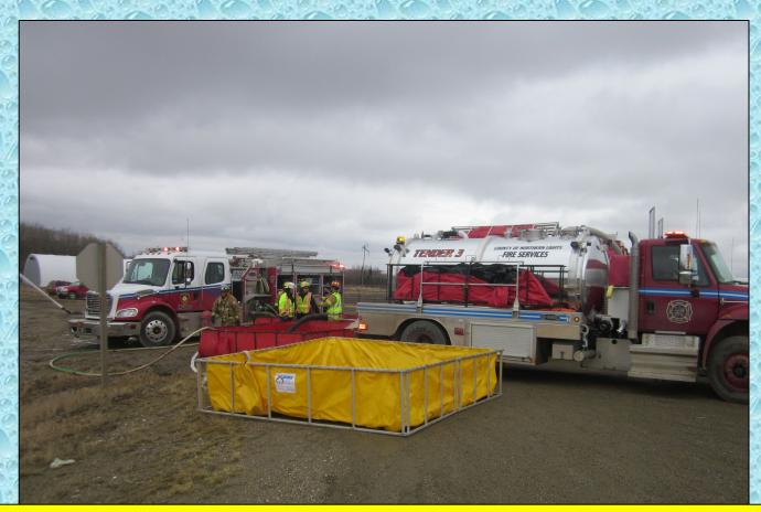
Two vacuum tenders were part of the shuttle and proved to be very critical to the success of the operation because of their ability to self-load at the lone fill site.
