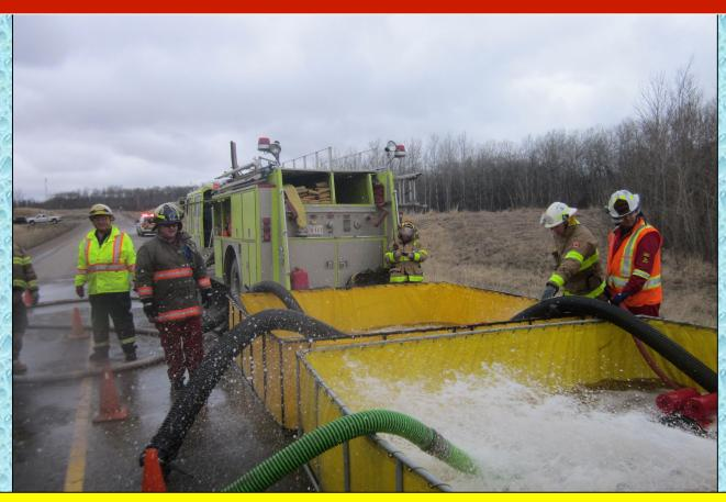
Weberville Engine 2 (1,500 gpm) drafted from the end dump tank and loaded tenders. The crew on the right controlled the flow of the portable pumps into the dump tanks in order to keep the tanks full for the next arriving tender.
