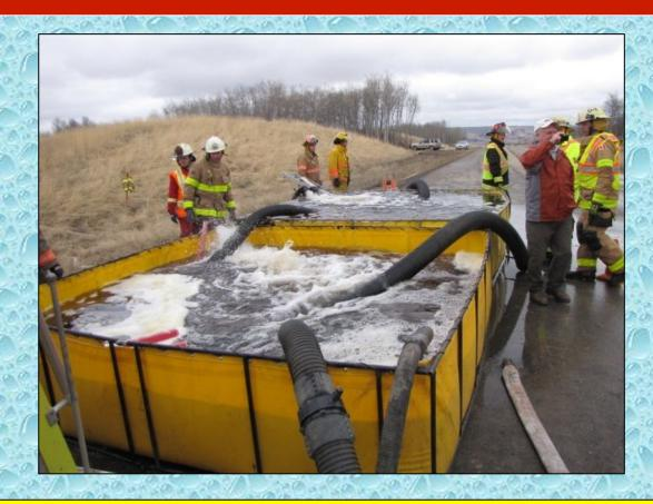
The fill site crew really did a great job of loading the tenders in as short a time frame possible. The 750 gpm tanker shuttle drill was supported by three portable pumps – which is pretty amazing!
