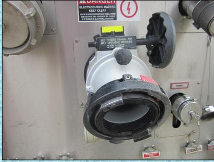
One of the issues that arose was the ability to get more water into the pump on Engine 8. The crew decided to add additional suction lines – starting with a second 6-inch suction from the officer's side of the pumper.
