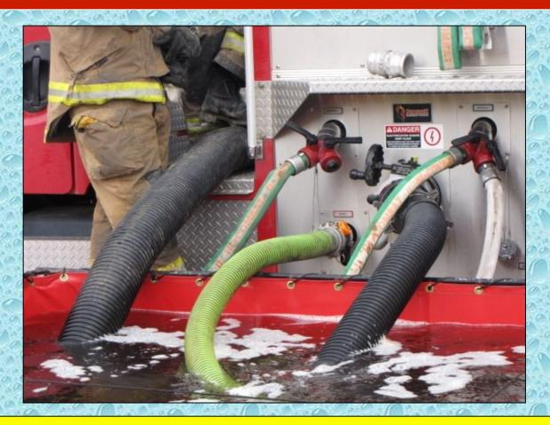
The three suction inlets allowed for maximum flow into the pump given the suction strainer selection available.
