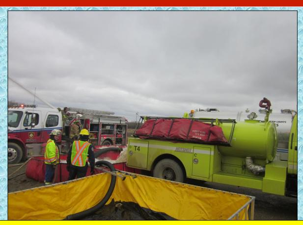
A third dump tank was placed but never put into operation. A 4,000-gallon dump tank was the first tank down – followed by a 2,100-gallon tank and that combination of tanks was adequate to support the 750 gpm flow.
