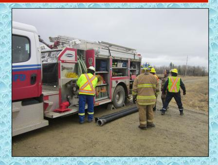
Peace River Engine 8 arrived on the scene and the timer was started when the pumper came to a stop. The crew went to work immediately setting up for a dump tank operation as well as stretching an attack line.
