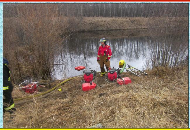
Three 250 gpm portable pumps were used to supply water back to the fill site via 2-1/2" hose. The pumps were able to meet the flow demand of the shuttle operation.
