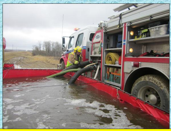
Eventually, the flow was moved to 750 gpm at the 38-minute mark using three suction lines – two, 6-inch suction lines and one 3-inch line (green).
