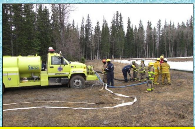
The second fill site never made it into operation because mud prohibited the pumper from getting close enough to draft from the ice covered pond.
