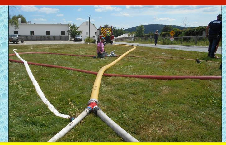
Two, tanker fill lines were set up off the pumper. One was supplied by LDH (red) the other was supplied by two smaller lines siamesed into a 5-inch line.
