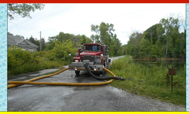
Bedford Engine 108 (1500 gpm) drafted from the pond located at the Patterson fire station and loaded tankers using LDH.
