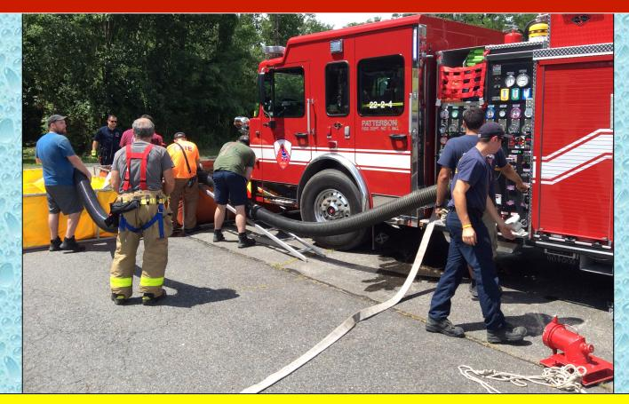
Dump site crews work to get a second, 6-inch suction line in operation. Each suction inlet on Engine 2-4 had a control valve which allowed additional suction lines to be brought on-line without interrupting flow to the aerial tower.
