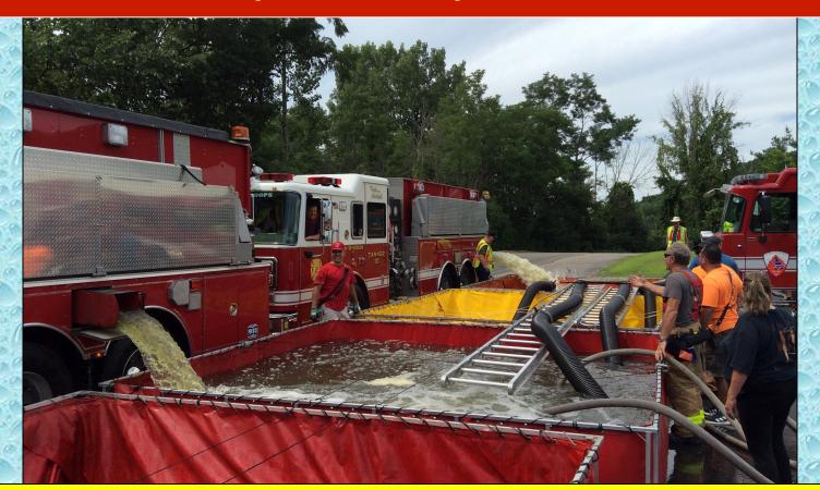
As flow increased it was important to be able to dump two tankers at one time and keep multiple jet siphons running.
