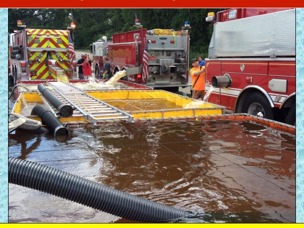
By the 35-minute mark flow was moved to 800 gpm and then again to 1250 gpm at the 52-minute mark. Three dump tanks were now in operation.
