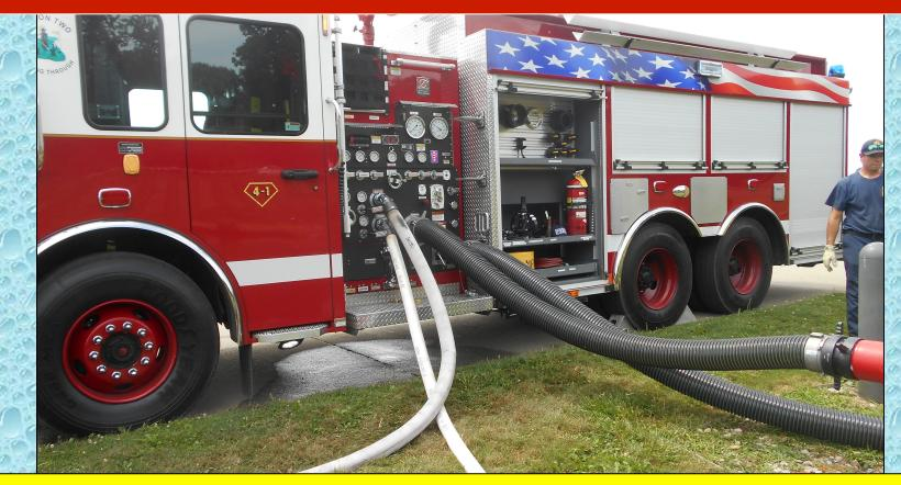
The crew used double, 6-inch suction lines to access the pond water. The first line used the dry fire hydrant and the second line went straight to the pond and used a barrel strainer suspended on a roof ladder.
