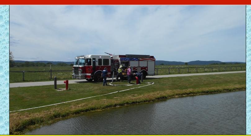
Mahopac Falls Tanker 4-1 (1500 gpm/2500 gal) arrives at the Watchtower pond and goes to work setting up to draft using the dry fire hydrant.
