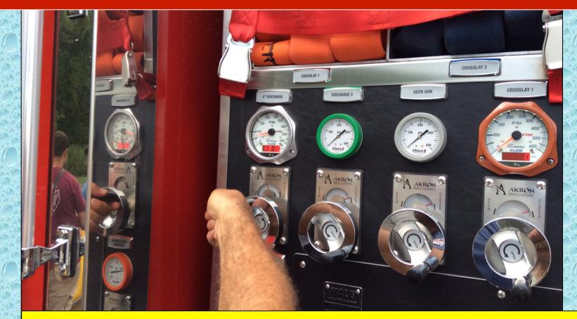
Around the 67-minute mark a flow of 1310 gpm was reached using the single, LDH discharge on Engine 2-4. The engine drafted through triple suctions, flowed 1310 gpm, and supplied water to run four jet siphons.
