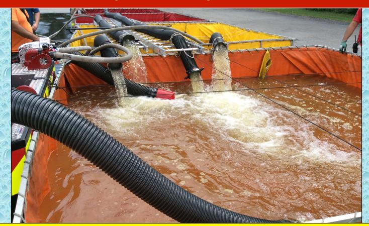
As the flow increased water transfer operations became really important. Four jet siphons were used to support the operation. A fourth dump tank was deployed and placed in-service as well.
