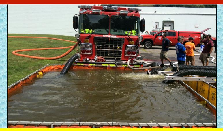
Double suctions in use. All water to the aerial tower was supplied via a single, 5-inch line about 400-ft long.
