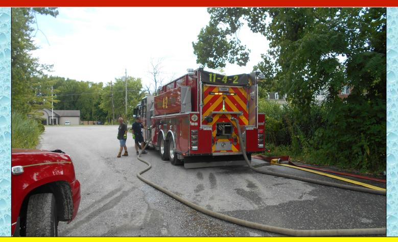
Some of the tankers loaded using 3-inch hose, some were able to load using 5-inch LDH.
