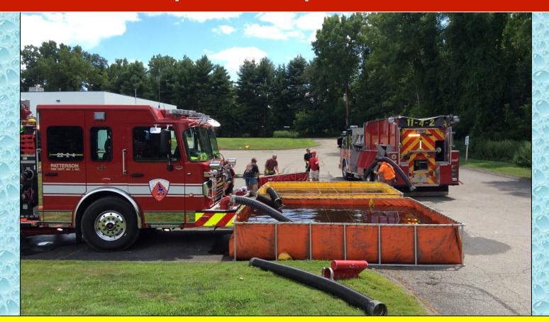
Around the 20-minute mark the flow was moved to 500 gpm and two dump tanks (3000 gal) were up and running.
