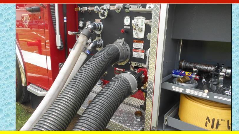
The 6-inch suction hose on the auxiliary intake was not an ideal arrangement but it did work and it did allow the pumper to take in more water. The gated intake allowed the second suction to be brought on line without interrupting flow operations.
