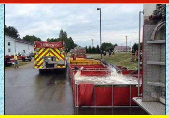
In the end, flow was never once interrupted. Three jet siphons were needed to support the operation and water was never moved more than once from any dump tank. The success of this high performing dump site was attributed to large pumps, a high-performing suction strainer (TFT), and standardized hose and fittings.
