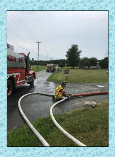
Much of the success of the drill was contributed to the folks loading tankers. Every tanker (10 in all) all loaded using the same method and same fill connection. The two fill sites loaded tankers at rates in excess of 1000 gpm and the sites operated like NASCAR pit stops.
