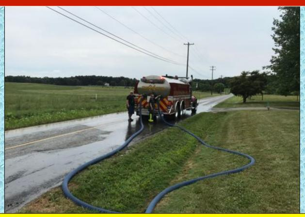
Each fill site pumper supplied water to an LDH manifold and did so using 5-inch LDH. From the manifolds, each tanker was loaded using dual, 3-inch lines equipped with Storz quick-connect couplings.
