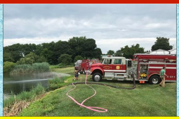
Cochranville Engine 27-1 positioned to use dual, 6-inch suctions to supply water for the second tanker loading station.
