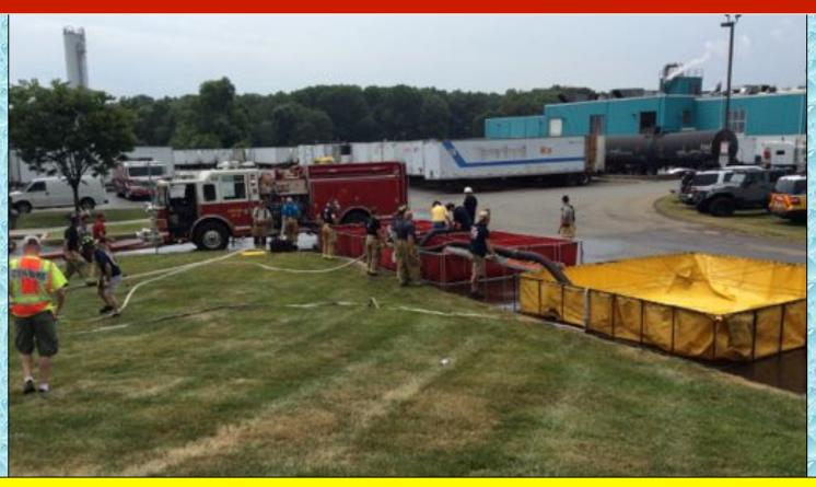
The first two dump tanks (red) set up came from Oxford Tanker 21, which was the first-arriving tanker. Carrying dual dump tanks allowed the crews to make a rapid build out of the dump site in preparation for a large flow operation.
