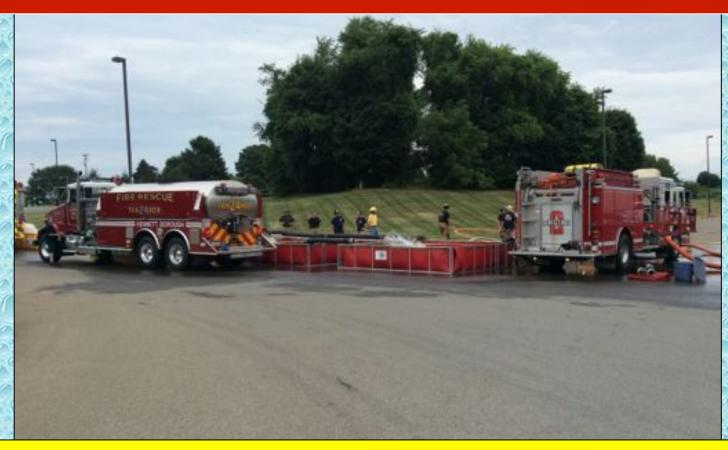
Another view of the dump site. At the 70-minute mark flow was moved to 1600 gpm and the dump site pumper was close to maximizing output since it was also supplying all jet siphons.
