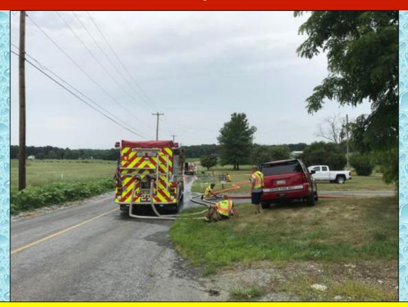
Both loading stations were located along the same road so traffic control was important as was tanker parking so that full tankers could pass tankers being loaded.
