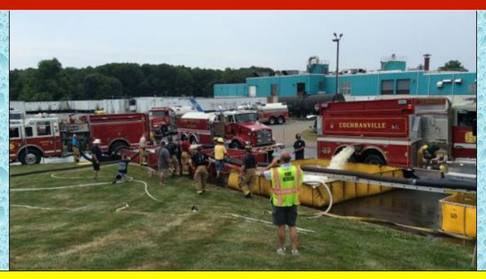
At the 48-minute mark, flow was moved to 1,000 gpm and four dump tanks were now in operation. With all of the tankers being large capacity, side dumping tankers, it was important to space out the third and fourth dump tanks so that two tankers could dump at the same time. This is a great example of the need to carry extra suction hose...which everyone did!
