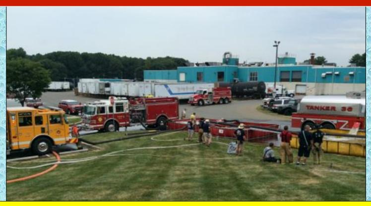
To maintain the 1750 gpm flow, West Grove Engine 22-2 (2000 gpm yellow) was used to run two of the three jet siphons...thus freeing up pump capacity on the Oxford engine. Engine 22-2 drafted from the primary dump tank to obtain its water supply.
