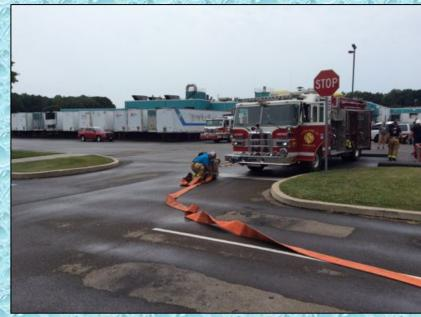
Oxford Engine 21-4 (left 1250 gpm) was the first-arriving engine and set-up to support Oxford Ladder 21 which was located about 600-feet away in a field. Oxford Engine 21-2 (right 1750 gpm) arrived and set up to supply water to Engine 21-4 via 500 ft of 5-inch LDH. Engine 21-4 supplied Ladder 21 using 5-inch LDH.
