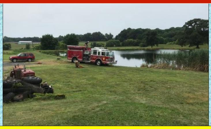
Oxford Engine 21-1 (1,500 gpm) arrives at the fill site and positions to get set up to load tankers by the time the first tanker arrives.
