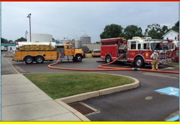
West Grove Tanker 22 was the second tanker to arrive on the scene and operated as a nurse tanker by feeding one side of the 5-inch double-clappered siamese. A 500 gpm flow at Ladder 21 was started at the 5-minute ....which was double the 250 gpm ISO test requirement.
