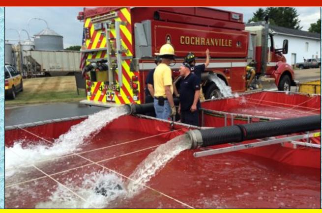
At the 30-minute mark flow was moved to 750 gpm and three dump tanks were in use...two, 3000-gallontanks and one, 4000-gallon tank. Water transfer became very important. Two very nice looking jet siphon streams are seen in this photo.
