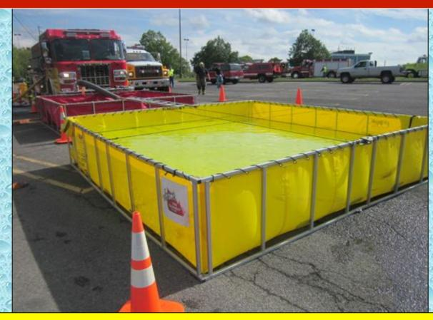
Meanwhile, two dump tanks (2,100 gal red and 2,500 gal yellow) were deployed in front of Engine 4 and the pumper's front suction inlet (5" pipe) was used.
