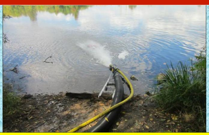
Water access was good, although vehicle access was a bit limited. Thirty feet of 6-inch suction hose was needed to access the water.
