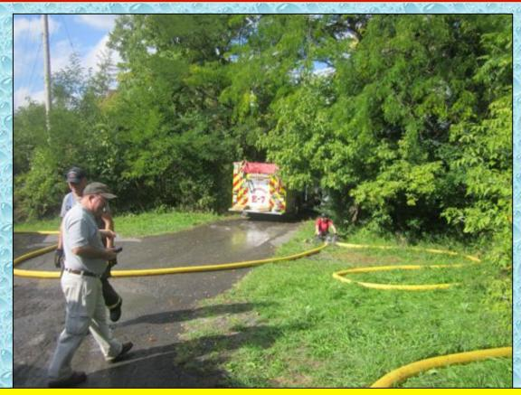
Baldwinsville Engine 7 (1,500 gpm) drafted from the canal and supplied a loading station that loaded tankers using 5-inch LDH.
