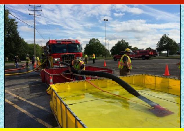
The singe-lane arrangement worked well, even with the four, square dump tanks. Engine 4 was able to support the 1,550 gpm flow and operate two jet siphons at the same time.
