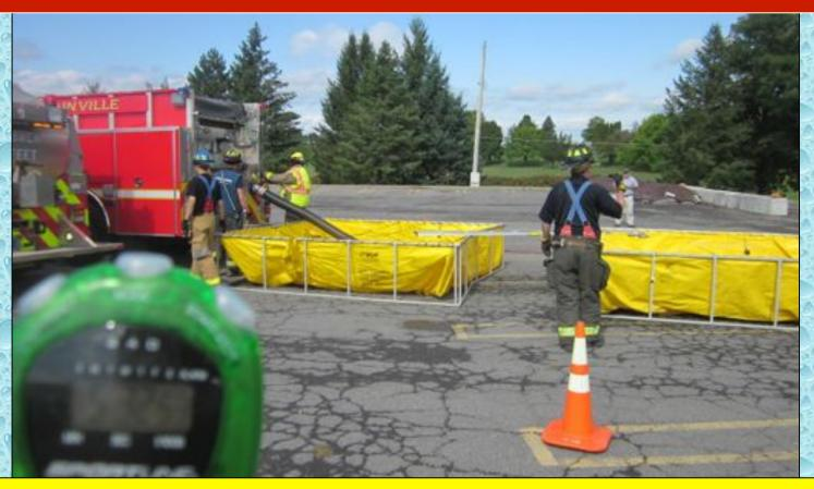
At the 5-minute mark, a second dump tank (2,500 gal) was deployed and crews continued to build out the dump site.
