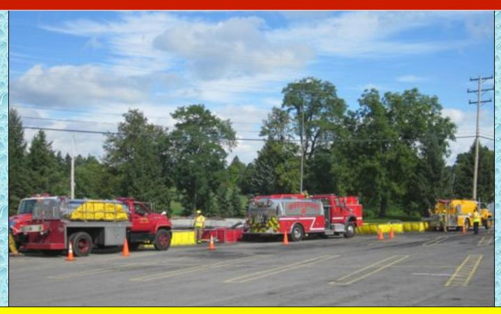
Around the 41-minute mark, the direction of travel was changed so that the tankers could dump off the driver side of the rig. This change reduced the amount of time spent at the dump site.
