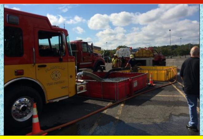
By drafting out of the rear and front intakes simultaneously, only two jet siphons were needed for the four dump tank operation.
