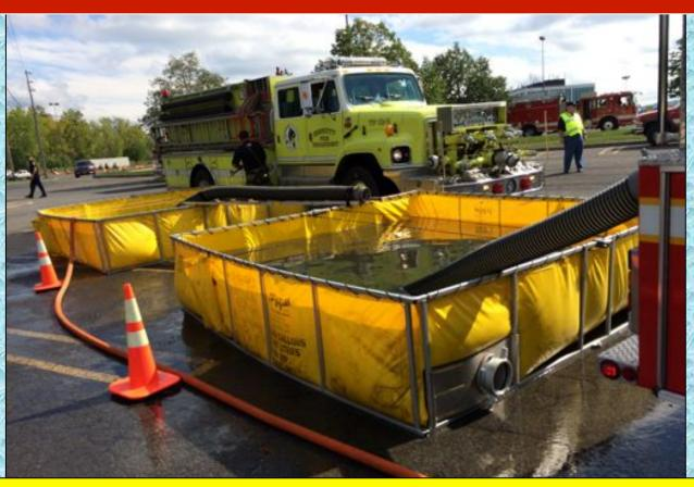
The Water Supply Task Force was able to arrive on scene, establish a 500 gpm flow within 11 minutes, and eventually support a 1,550 gpm flow using 10 tankers.
