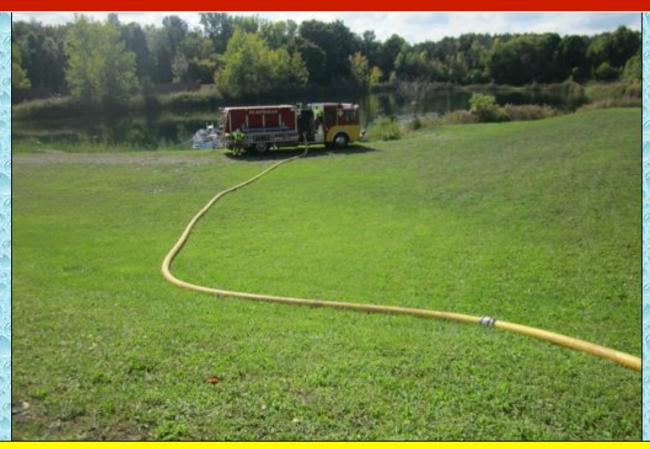
Plainville Engine 3 (1,500 gpm) gained access to this large pond and supplied water to the loading site using 300 feet of 4-inch LDH.
