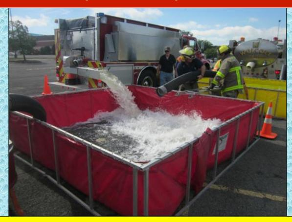
Shown here at the 18-minute mark, tankers are now dumping water while crews continue with the build out operations.
