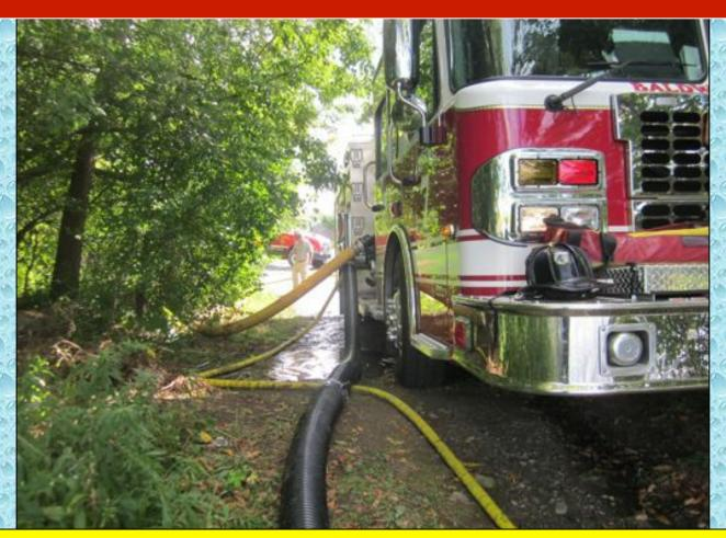
The crew set up to draft using one of the side suction inlets, thus giving the 1,500 gpm pumper the best chance of success for maximizing output.
