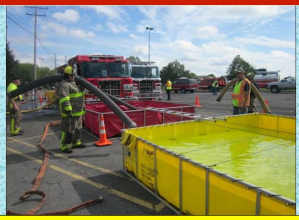
Arriving crews worked to build out the 4-dump tank operation. Meanwhile, two fill sites were under construction using other pumpers from the Water Supply Task Force. At the 11-minute mark, a 500 gpm flow to the tower was started.
