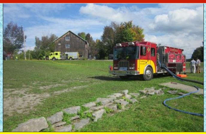
The pumper carried sufficient lengths of suction hose to reach the pond and the crew was able to set up operations without incident.
