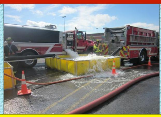
The Firovac vacuum tanker offloads its 3,000 gallons of water. Water transfer operations are now also underway.
