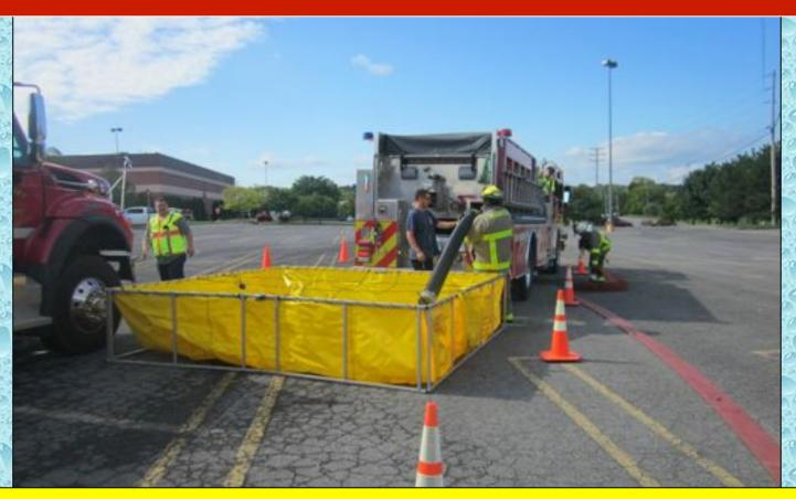
The first dump tank (2,100 gal) was deployed to the rear of Engine 4 (1,750 gpm) and suction was set-up to the pumper's 6-inch rear intake.
