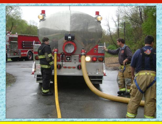
The crew is shown above using a 5-inch and a 3-inch line to fill a tanker. This arrangement made filling operations go rather fast.
