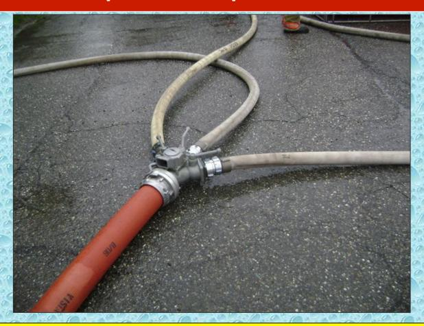
Because E142 (1500 gpm) did not have a high-flow discharge, three, 2-1/2inch lines were used to feed the 5-inch supply line going to the tower ladder.
