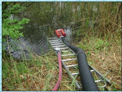
Bedford Engine 110 (1,250 gpm) operated as the pumper at this fill site. Access to the pond was good and crews did a good job of setting up the pumper for drafting operations.
