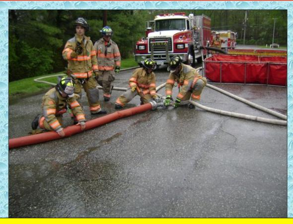
With the dump site pumper (E142) now in position and a draft established, the crews work to switch over from a nurse tanker operation to a dump and run operation.
