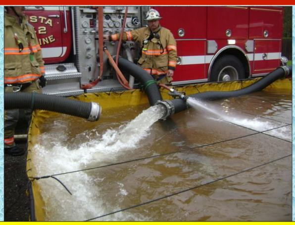
Jet siphons were put into operation in order to transfer water from the outer dump tanks to the primary dump tank. E142 is shown here drafting and running two jet siphons.
