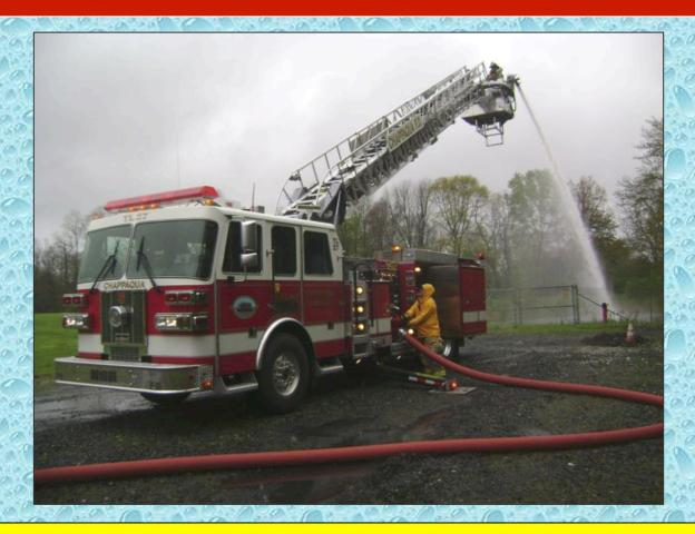
At the 15:00 minute mark, the flow is moved to 500 gpm. The tower's flow meter was used to monitor the flow rate.
