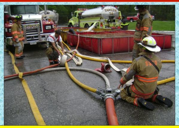
With a goal of 1,500 gpm, the crew works to change out the three, 2-1/2-inch lines feeding the 5-inch line. They are replacing the hose with three, 3-inch lines. This change out should allow the 1,500 gpm pumper to reach the 1500 gpm goal and still run the jet siphons.
