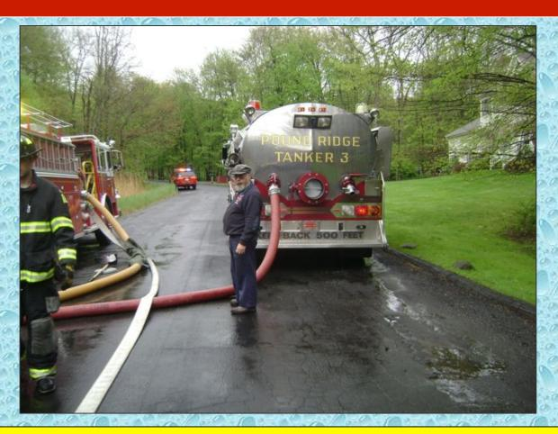
Pound Ridge Tanker 3 is shown above being filled with a 5-inch line through its large capacity direct fill.
