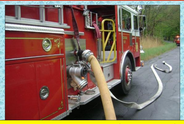
Being an older pumper, E110 did not have a high-flow discharge, so flow through the 5-inch hose shown above was limited - but adequate enough to sustain the filling of tankers at this site. A better approach might have been to feed the 5-inch with dual- 3" lines from two discharges. This would have been needed if flow was to be increased again.
