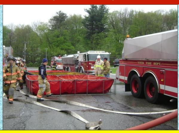
Two more dump tanks - 3,500 and a 3,000 gallon - are placed while nurse tanker operations are continued. First-alarm resources arrived in a timely manner and brought with them plenty of tools and equipment to build a working dump site.
