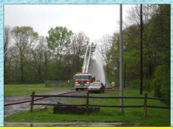
At the 5:49 minute mark, Tower Ladder 27 begins flowing the required 250 gpm. The tower's flow meter was used to measure the flow throughout the drill.
