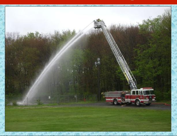
With the 3-inch hose now changed out, the flow is once again increased at the 75:00 minute mark – this time to 1,500 gpm.
