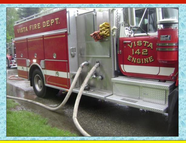
Vista E142 uses all of its available discharges to support the tower ladder and the jet siphons.
