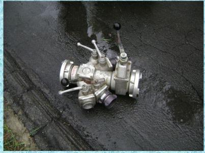
Some problems occurred at this fill site with the use of an LDH manifold, however, the fill site crew was able to work through the problem and keep filling tankers. This was good reinforcement for being prepared to handle malfunctioning equipment.
