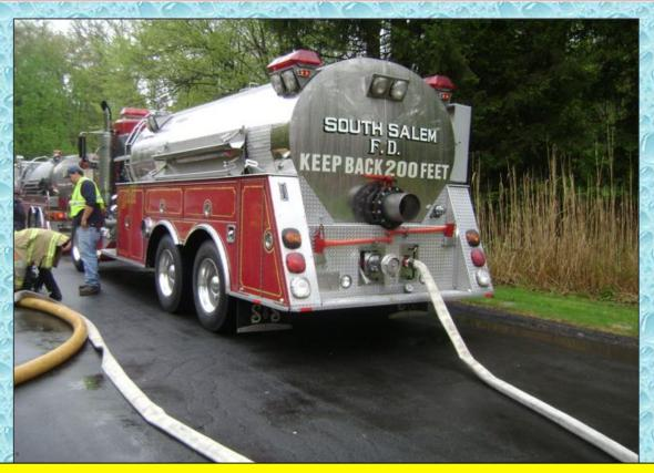
South Salem's tanker is shown being filled by a 3-inch line. However, an improved approach would have been to connect a 5-inch line directly to the large capacity direct fill.
