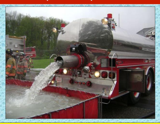
The extra-large dump on this tanker allows for an extremely fast offload rate.
