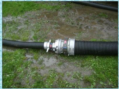
E168 used a 6-inch dry hydrant as the primary suction point and the crew added a 2-1/2-inch suction line to increase the pumper's capability. The photo on the right shows a section of 6-inch suction hose that had to be used to replace a bad section of 2-1/2-inch suction. That is why redundant adaptors are so important!
