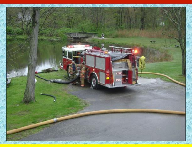
South Salem Engine 168 (1,500 gpm) was used to operate this fill site. The fill site was set-up in short order.
