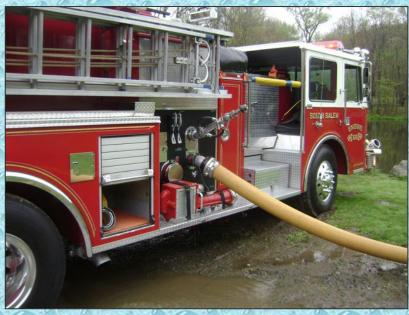
E168 is shown above supplying the 5-inch LDH. The operator also used one of the rig's 2-1/2-inch discharges as a recirculation line for maintaining the pumper's draft when not pumping to a tanker.
