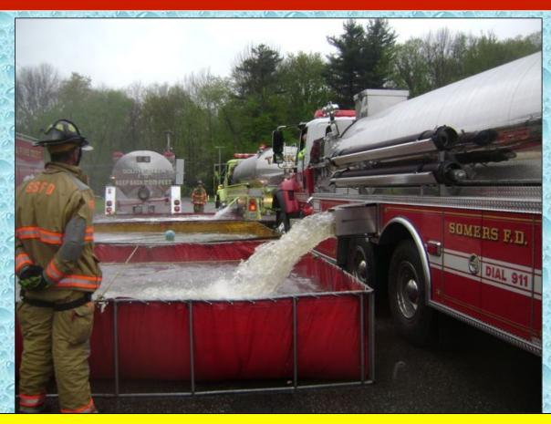
With the large, 3,000-gallon plus dump tanks arranged in a parallel fashion, two tankers can offload at the same time. Such arrangement will really make a difference once the flow moves above 1,000 gpm.
