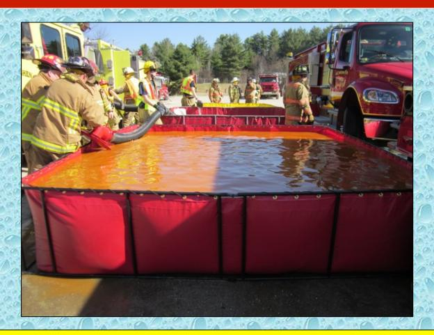
A second jet siphon is assembled and placed in the third dump tank. Water transfer operations are ready to begin from the 3<sup>rd</sup> dump tank.
