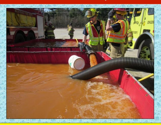
The jet siphon on the 4-1/2-inch suction hose is working just fine as a water transfer device.
