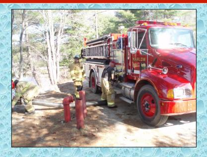
The Marlow crew elected not to use the dry hydrant because of some previous problems with the hydrant. So they set up to draft directly from the pond.
