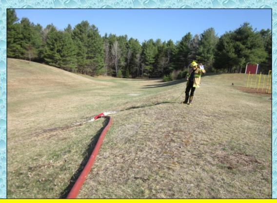
At the 5:00-minute mark, a flow of 280 gpm was started through the flow measuring device. An attendant was assigned to monitor flow readings.
