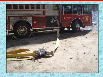
The crew used an LDH manifold to set up a variety of fill lines in order to accommodate the variety of tanker fill connections.
