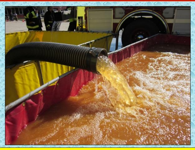
The 6-inch jet siphon from the 2<sup>nd</sup> dump tank is also working just fine in transferring water.
