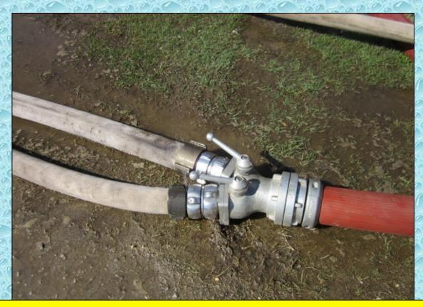
A 2-way gated valve was used and was supply by a 50-ft length of 2-1/2" hose and a 50-ft length of 3-inch hose – both supplied by 2-1/2" discharges on the pumper.
