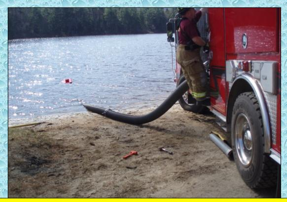
Because the water level was shallow near the shore, 30-feet of suction hose was needed to get the strainer into a proper location.
