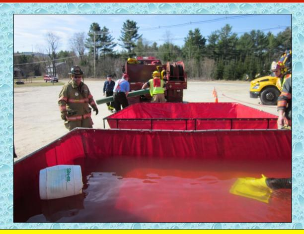
Knowing that they wanted to eventually expand the flow, a third dump tank (2,100 gallons) was deployed.
