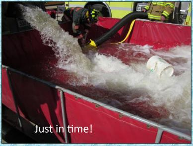
Water flow still hadn't stabilized and Newport's tanker was needed to dump its load of water directly into the primary dump tank.
