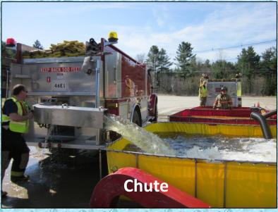
When having to use a detachable chute for offloading, one choice is to just leave the chute at the dump site rather than using up valuable time stowing it back on the tanker.
