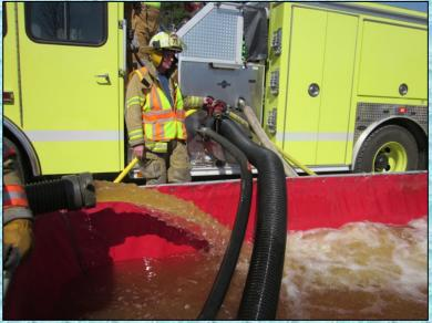
In order to increase the pumping capacity of the 1,250 gpm supply pumper, the crew added an additional suction. By adding in the 2-1/2-inch suction the pumper was able to improve its pump capacity and operate the two jet siphons without jeopardizing the flow to the attack engine.
