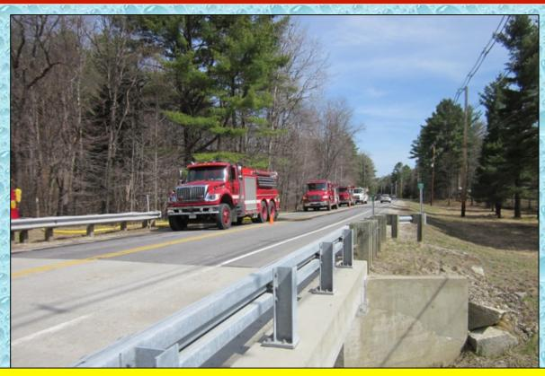
Another issue that actually affected the overall flow rate of the shuttle was the waiting in line to fill at this fill site while the pond site had no one waiting in line. Once the distribution of tankers to fill sites was corrected, flow sustainability was significantly improved.
