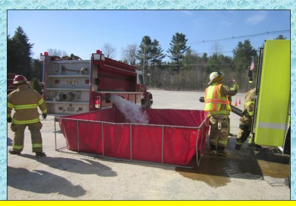
With no nurse tanker operation in place – the crews really hustled to get that first dump tank (2,000 gallons) set up. At the 6:24-minute mark, water was being dumped into the tank. However, note that the pumper is not yet ready to draft. This was a bit of a problem.
