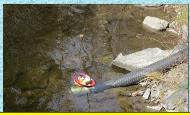
While the brook had plenty of water, the pumper was a little short on suction hose causing the barrel strainer to be right at its point of effective use. At high flow, a vortex would start. To remedy the situation, the crew used a hard as a vortex inhibitor – it worked just fine!
