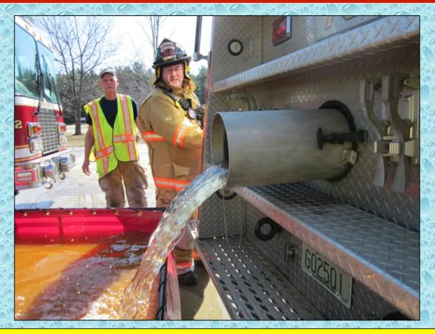
When water flow from a dump chute reaches this level it is time to "cut and run". Efficiency is only going to drop if folks wait for all of the water to offload.
