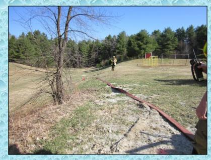
The four person engine crew went to work stretching hose in preparation to start flowing water. A 4-inch line was stretched to support a flow measuring device that was used in lieu of a nozzle for more accurate flow measurement.
