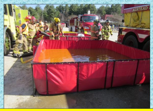
The third dump tank has water in it and awaits a transfer device. Probably not the best scenario because this water is "trapped" until a jet siphon is put into operation.
