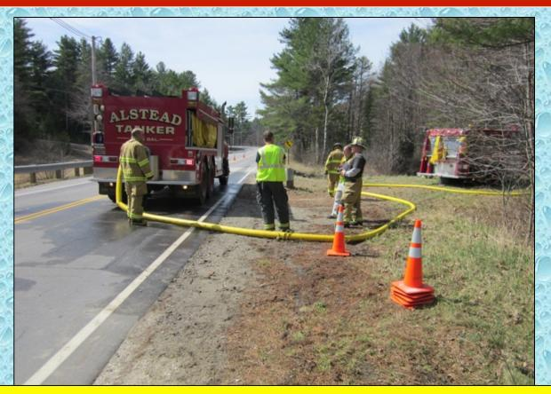
Another item that would have helped would have been the use of an LDH manifold or control valve so that the pump operator did not have to control the fill. However, the site was filling tankers at around 900 gpm.
