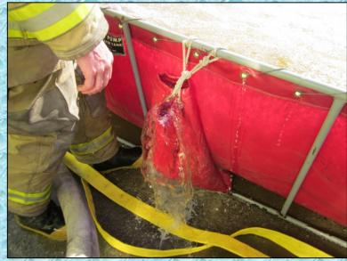
Dump tank drains can create an unnecessary mess when they are not properly secured. A dump site is a wet place to begin with and anything that can be done to reduce more spilled water is a great help. One choice is to tie up the drains on the inside of the tank instead of on the outside as shown above.
