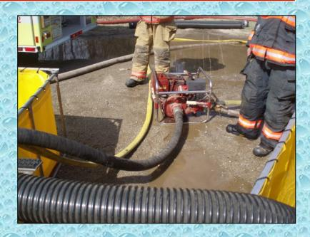
A 250 gpm portable pump was used to run the jet siphon for the 4<sup>th</sup> dump tank. However, the 4<sup>th</sup> tank was never really used much because water was almost always needed in the primary dump tank. This was a sign that the operation had maximized the capability of the water hauling rigs and that in order to move to a higher flow – more tankers or improved filling operations would be needed.
