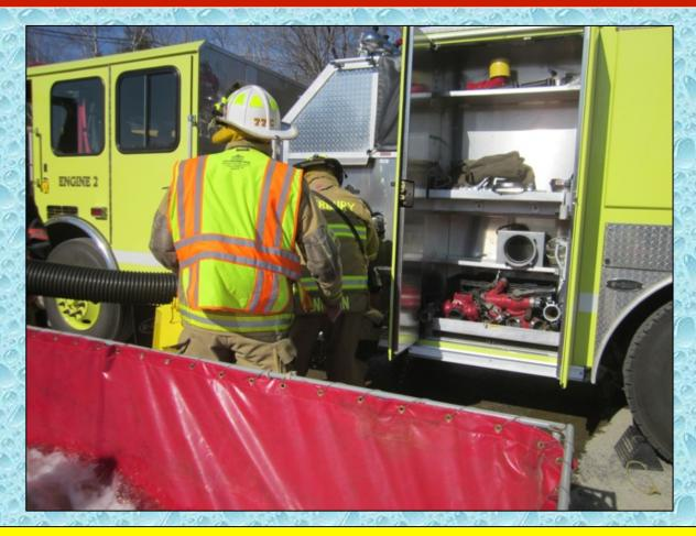
The race is on to get the dump site pumper in operation drafting from the dump tank.
