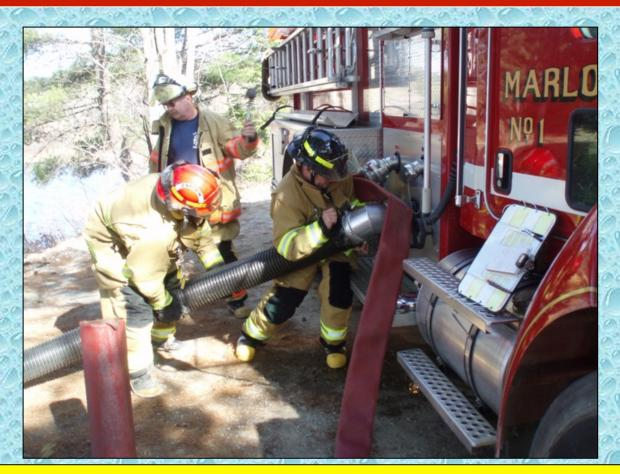
The final connection was made and the pumper quickly picked up the draft.
