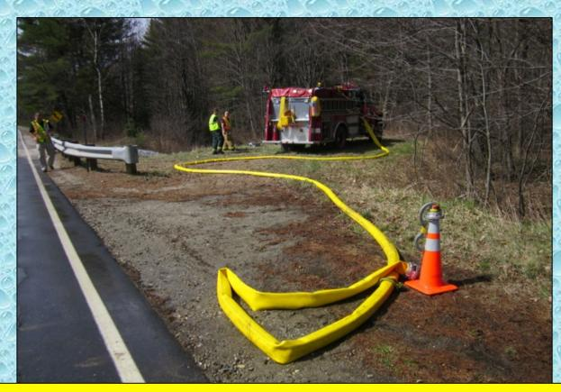
The two-person crew did a nice job of getting the site set-up and equipped to fill tankers. A 4-inch hose line was used as the tanker fill line.
