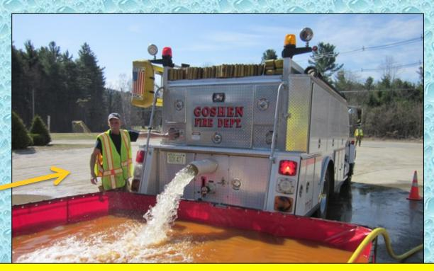
When both rear and side dumping tankers are involved in a shuttle operation, it is best to make arrangements for the rear dumping tankers to offload their water in a position where they don't block out side dumping tankers. Goshen's 77 Engine 1 is shown here dumping in the last dump tank – thus leaving room for side dumping tankers to pass on the left.
