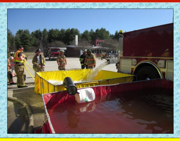
Acworth's tanker dumps its water into the second dump tank now that a jet siphon is ready and in position.
