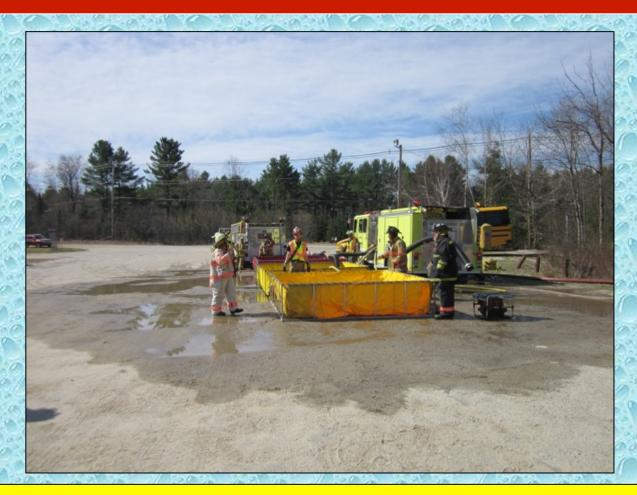
A fourth dump tank (1500 gallons) was deployed around the 56:00-minute mark with intentions of increasing flow once again.
