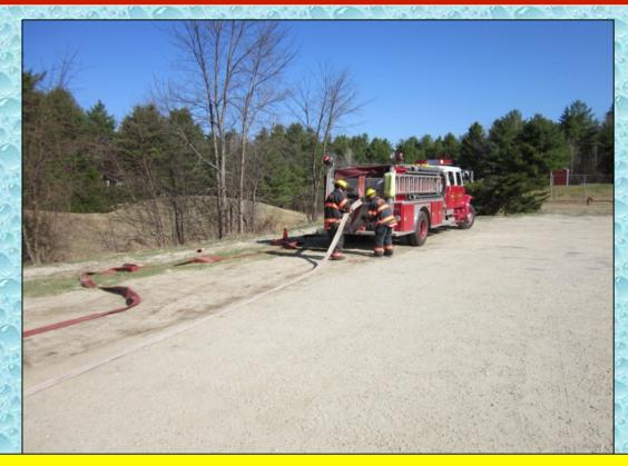
Realizing that the single, rear discharge on the pumper might not support the higher flows that were expected, the engine crew took time to use two smaller lines from individual discharges in hopes of being able to hit the 1,000 gpm flow mark without incident.
