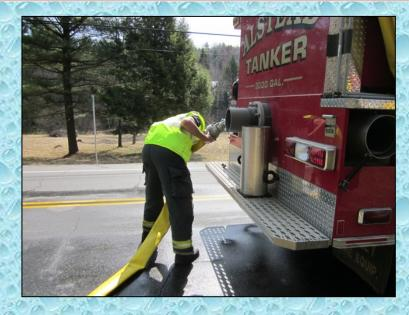
One issue that arose at this fill site was the need for adaptors and fittings because many of the tankers did not use the same fitting – which slowed down the tanker fill process.
