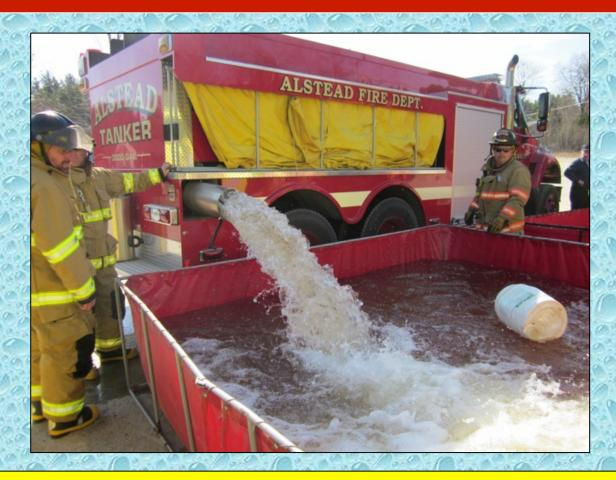
With still just two dump tanks in operation, Alstead's tanker has to dump into the primary drafting tank while jet siphons are set up.
