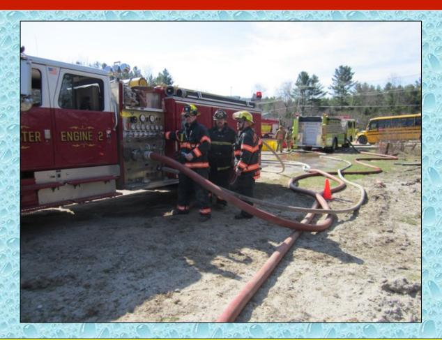
Being supplied through both a 4-inch and a 2-1/2- inch supply line, the attack engine moves the flow to 825 gpm at around the 48:00 minute mark.
