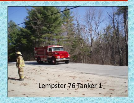
A large pond (Dodge Pond), equipped with a dry fire hydrant, was used as a fill site for this drill. As happens sometimes in real life, a tanker arrived at about the same time as the fill site pumper. A point worth noting here is that if the tanker had been a vacuum tanker, it could have self-loaded and been on its way back to the dump site by the time the fill site pumper got set up.
