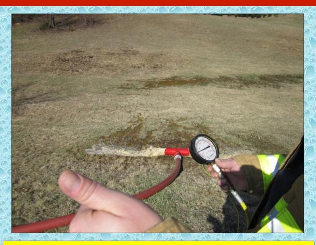
At the 28:00 minute mark, flow was increased to 504 gpm.
