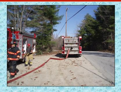
Meanwhile, the Lempster tanker crew helped set-up the tanker fill hose and got their rig into position for loading as soon as the Marlow pumper achieved a draft.
