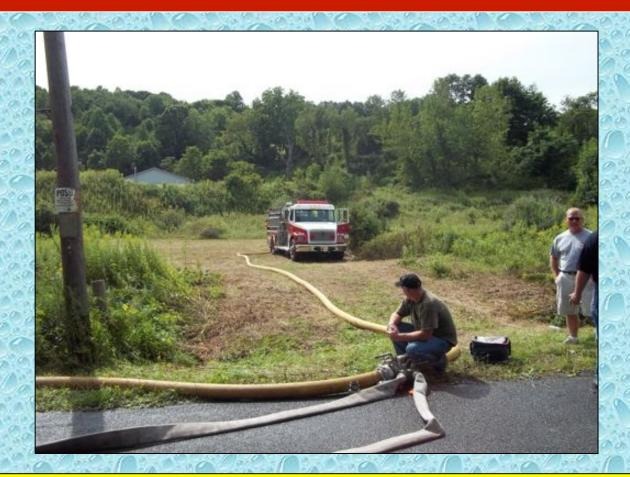
The Cascade fill site was able to fill tankers at the recommended 1,000 gpm rate without any problems.
