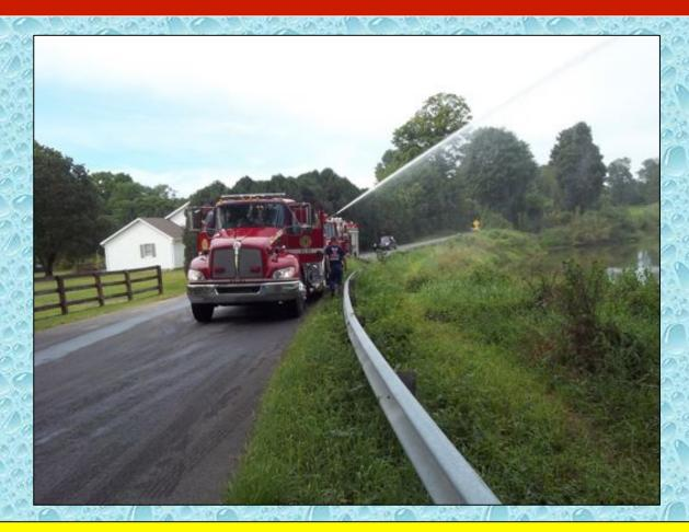
Pine Plains Engine 55-13 (1,250 gpm) was used at this fill site. The pumper can be seen in this picture flowing its deck gun.
