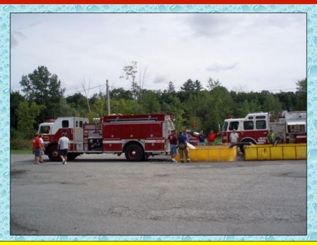
Dump site crews had to manage a mixture of tanker types such as this rear off-loading engine/tanker.
