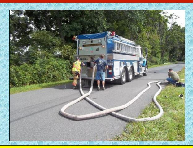
Wassaic Tanker 69-31 was the first tanker filled at the site and 3-inch hose was used as the fill line.
