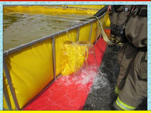
When using dump tanks that have drains that are tied up with rope, it is best to tie up those drains on the INSIDE of the tank.
