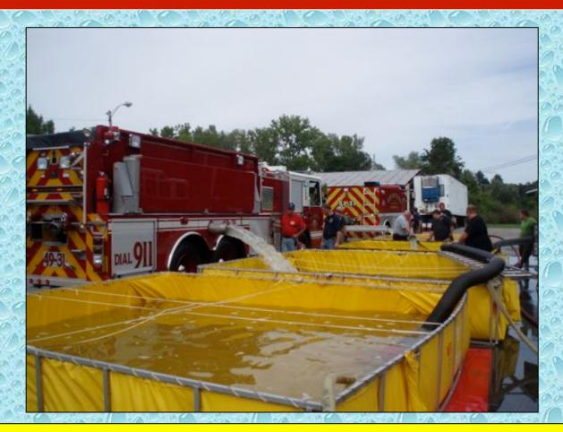
With four tanks up and running, the crews worked hard to keep the 1,000 gpm flow sustained.
