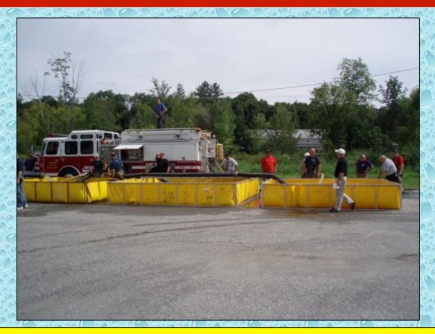
Water was transferred from the fourth tank to the primary drafting tank by "jumping" the third tank.
