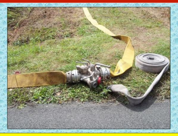
A LDH manifold was used as the loading valve for tanker fill operations at this fill site.
