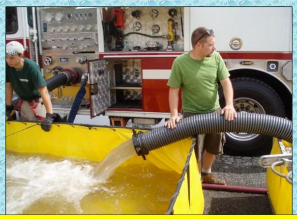
Water transfer operations are critical to the success of increased flow rates. This single transfer device worked fine for the 500 gpm flow rate. However, an additional transfer device was needed once flow was increased.
