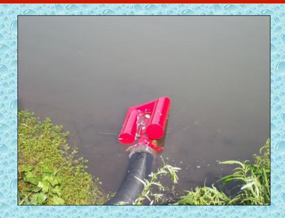
The water supply site for the Mygatt Road fill site required the pumper to draft.
