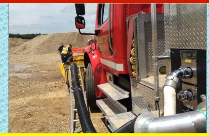
The dump site crew chose to set up the dump tanks in front of Engine 228 and used a Fol-Da-Tank suction elbow to help improve suction hose deployment.
