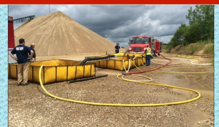
Engine 228 (1250 gpm) worked hard to pump 750 gpm and supply three jet siphons. A second suction line was connected to the pumper. A length of 4-1/2-inch suction hose was connected to the pumper's front intake in order to increase flow intake.
