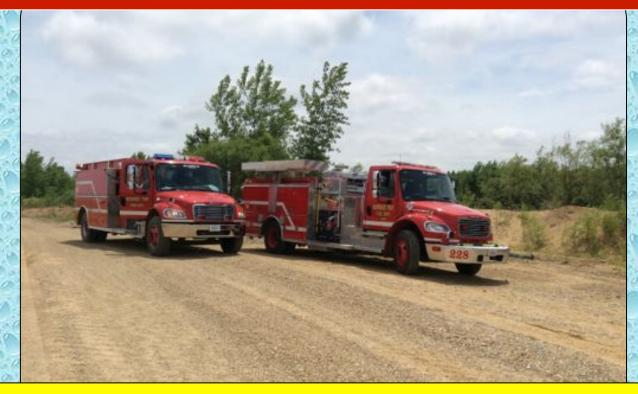
Monroe Engine 228 was the first unit to arrive followed closely by Monroe Tanker 220. The engine was set-up to serve as both the attack engine and the dump site engine. A nurse tanker operation was used to supply Engine 228 during the initial operations. The timer was started when Engine 228's operator applied the parking brake.
