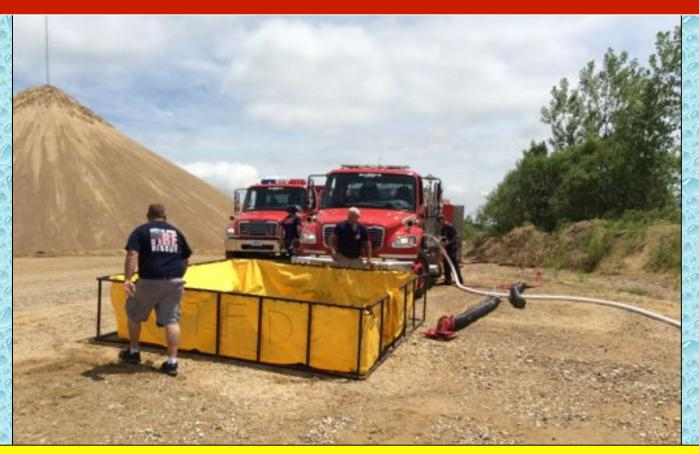
The crews stretched a 100-ft, 2-1/2-inch attack line and fed an Elkhart portable monitor. Meanwhile, other folks worked to get the first dump tank set up while the nurse tanker supported the fire attack.
