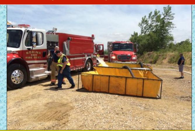
Robins Tanker 360 was the second tanker to arrive at the dump site and the first tanker to dump its water. Operations soon switched to a dump tank operation and the nurse tanker was cut loose to begin shuttling water.
