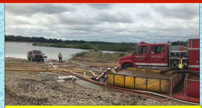
Monroe Engine 224 operated the first fill site by using a combination of a portable pump and a Turbo Draft to supply water back to a dump tank in an open relay format. The engine then drafted from the dump tank and loaded tankers.
