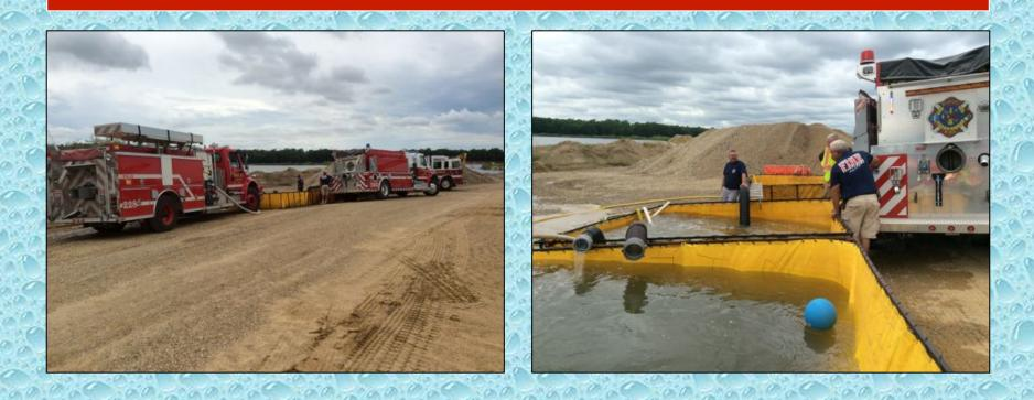
One of the unintended challenges that arose was the placement of the dump tanks. While not severe, the grade of the road reduced the usable capacity of each dump tank.
