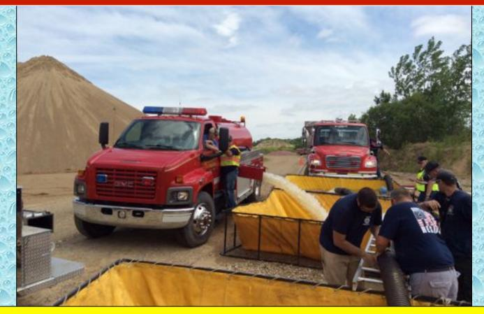
Center Point Tanker 140 dumps its first load of 2000 gallons as part of the second Tanker Task Force. Meanwhile, the dump site crew works to build a jet siphon so that the third dump tank can be made operational.
