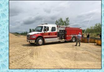
Palo Tanker 345 – 1,250 gpm pump w/3,000 gal tank
