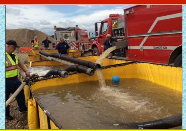
Three jet siphons were used to transfer water to the primary dump tank from the other two dump tanks thus allowing the 750 gpm flow to be pumped uninterrupted.
