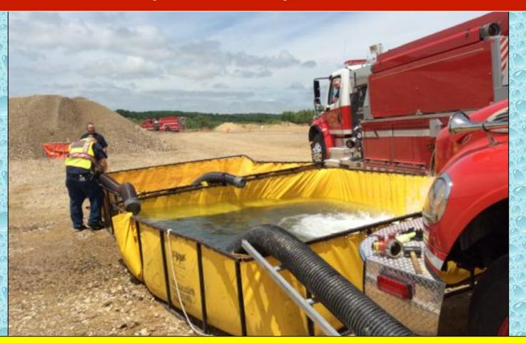
As additional tankers arrived on the Tanker Task Force, crews worked to set up a second dump in preparation for increasing the flow to the ground monitor.
