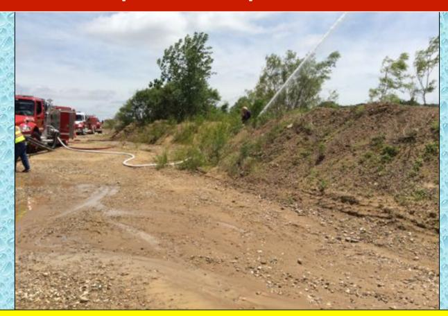
Water flow was moved to 500 gpm at the ground monitor and the pressure was now put on the fill sites to keep the tankers loaded and on the road.
