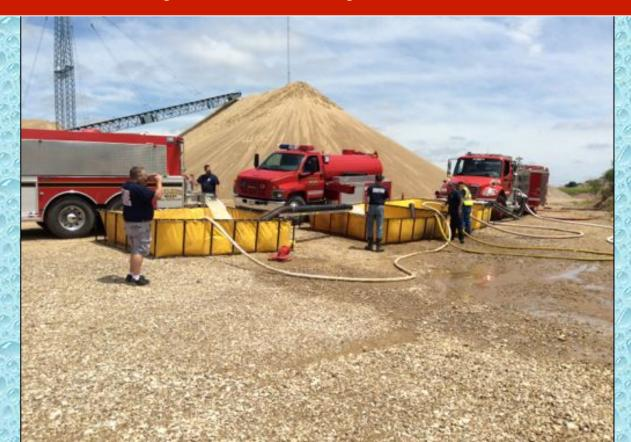
Three dump tanks are now in operation and the flow is moved to 750 gpm using two, portable ground monitors.
