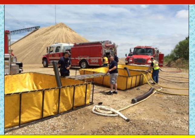
Knowing that they would most likely need to dump two tankers simultaneously, the dump site crew spaced the third dump tank several feet from the second tank and used a ground ladder to bridge the gap.
