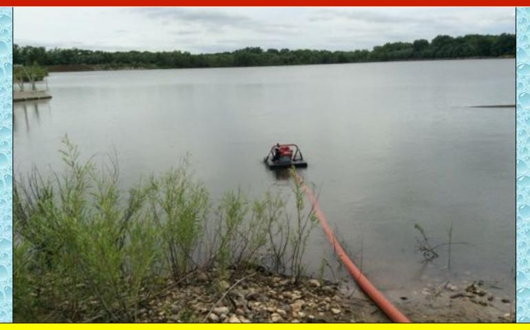
Monroe Engine 224 ran a similar fill site operation using this CET portable floating pump and another Turbo Draft to supply an open relay set-up.
