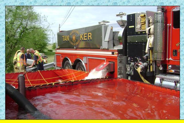
The positioning of the dump tanks next to a bridge made it difficult for the larger tankers to maneuver into position for offloading.
