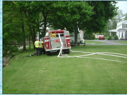
Smithsburg Engine 74 (500 gpm) struggled to provide an effective fill rate even though they had good access to water.
