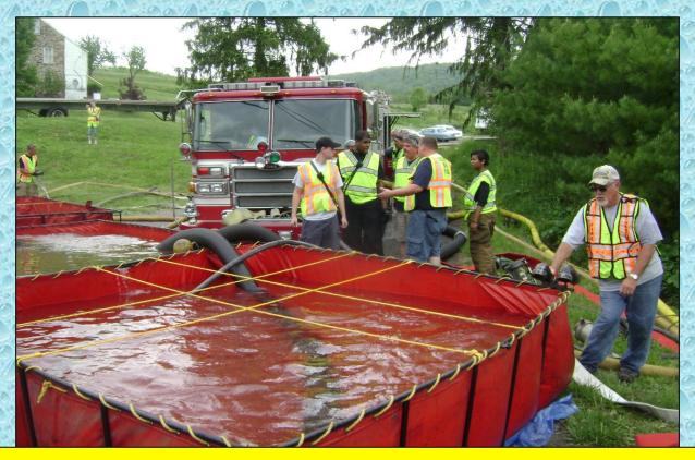
The key to the success at this dump site was the use of a large capacity pumper and large capacity dump tanks.
