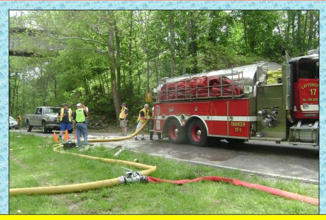
When not pumping to the dump site, the crew filled tankers using an LDH manifold and 5-inch hose.
