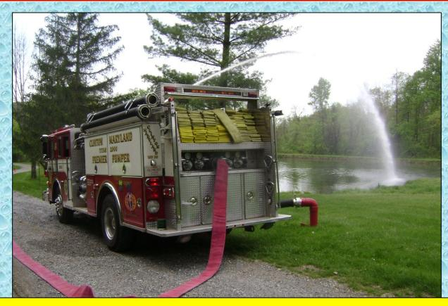
The water supply rig used a dry hydrant at the pond and was able to maintain a strong flow of water.
