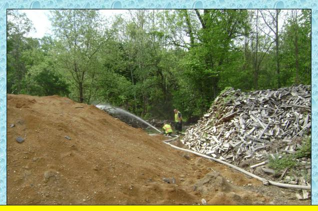
Water flow was started at the 5:00 minute mark with 250 gpm through a 2-1/2-inch attack line.
