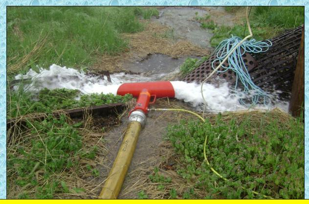
A large, flow diffuser equipped with a fixed pitot was used to measure flow at the attack engine. Here, the flow is moved to 500 gpm at the 15-minute mark.
