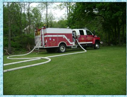
In addition, Engine 74 was using 3-inch hose to fill tankers that had large direct fill lines – this also hampered the fill rate.
