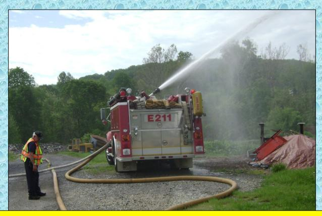
With both a tanker operation and a relay pumping operation supporting the fire attack, Wolfsville E211 placed its 1,000 gpm deck in service – thus moving the flow to 1,500 gpm.
