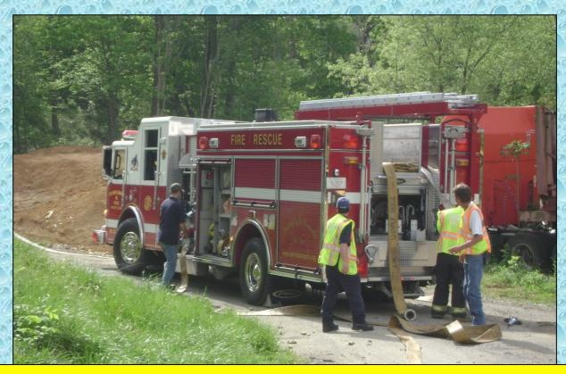
With the clock now running, the attack pumper crew prepares to stretch an attack line for initial water flow. The crew also connects up the supply line so that they can transition to a water supply operation from the dump site pumper.
