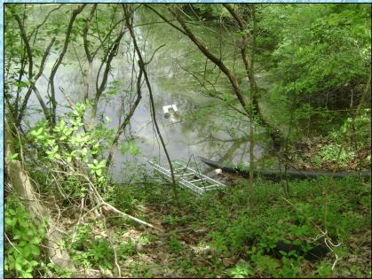
The 3<sup>rd</sup> fill site was supported by Pleasant Valley Special Unit 6 (1,500 gpm). The crew drafted from a stream and pumped water to the dump site through about 2,000 feet of 5-inch hose. They also filled tankers.
