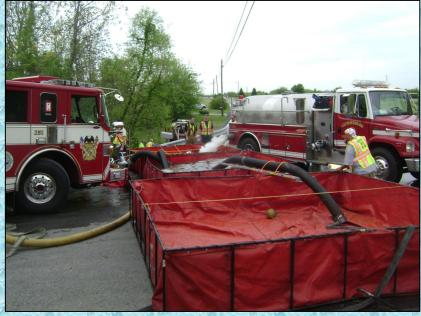
After a brief interruption in flow to replace the broken section of 4-inch hose, the operation was back up and running. The operation moved to a 3-tank set-up. In addition, the dump site pumper also received water from the nearby brush truck and from a 5-inch hose relay from a pond about 2,000 ft away.
